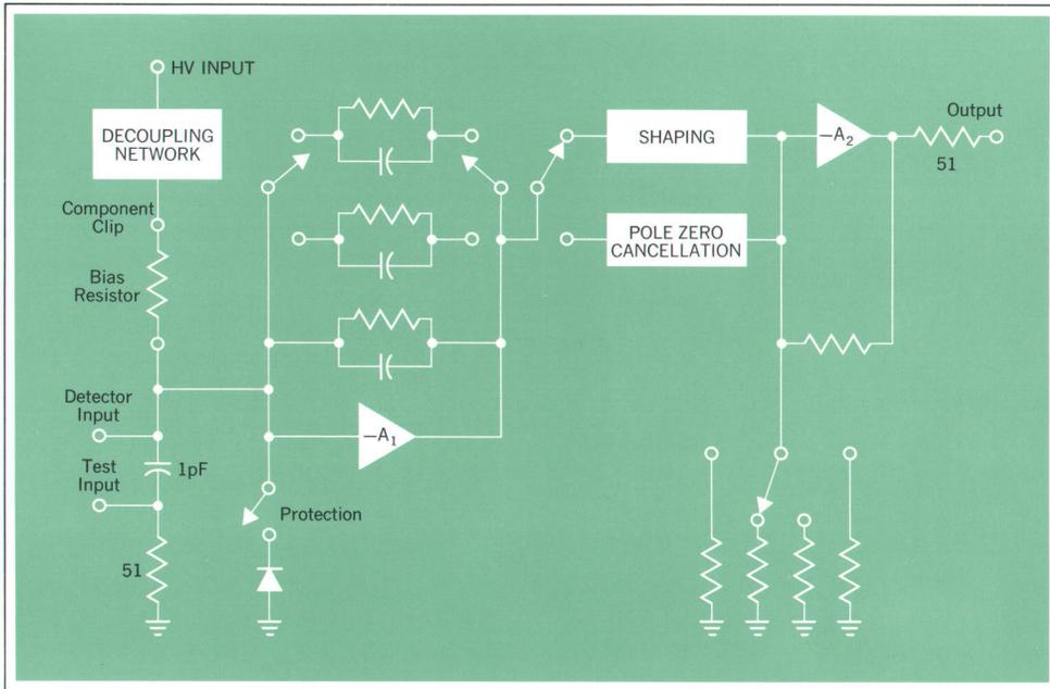
Fig. 3. Block diagram of preamplifier.
