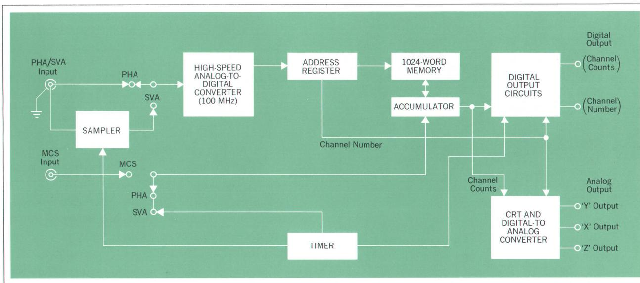
Fig. 4. Block diagram, HP Model 5400A Multichannel Analyzer.
