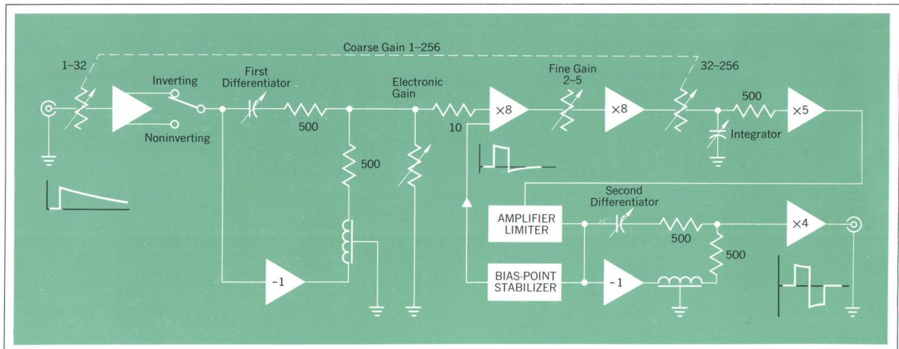
Fig. 2. Linear amplifier block diagram.
