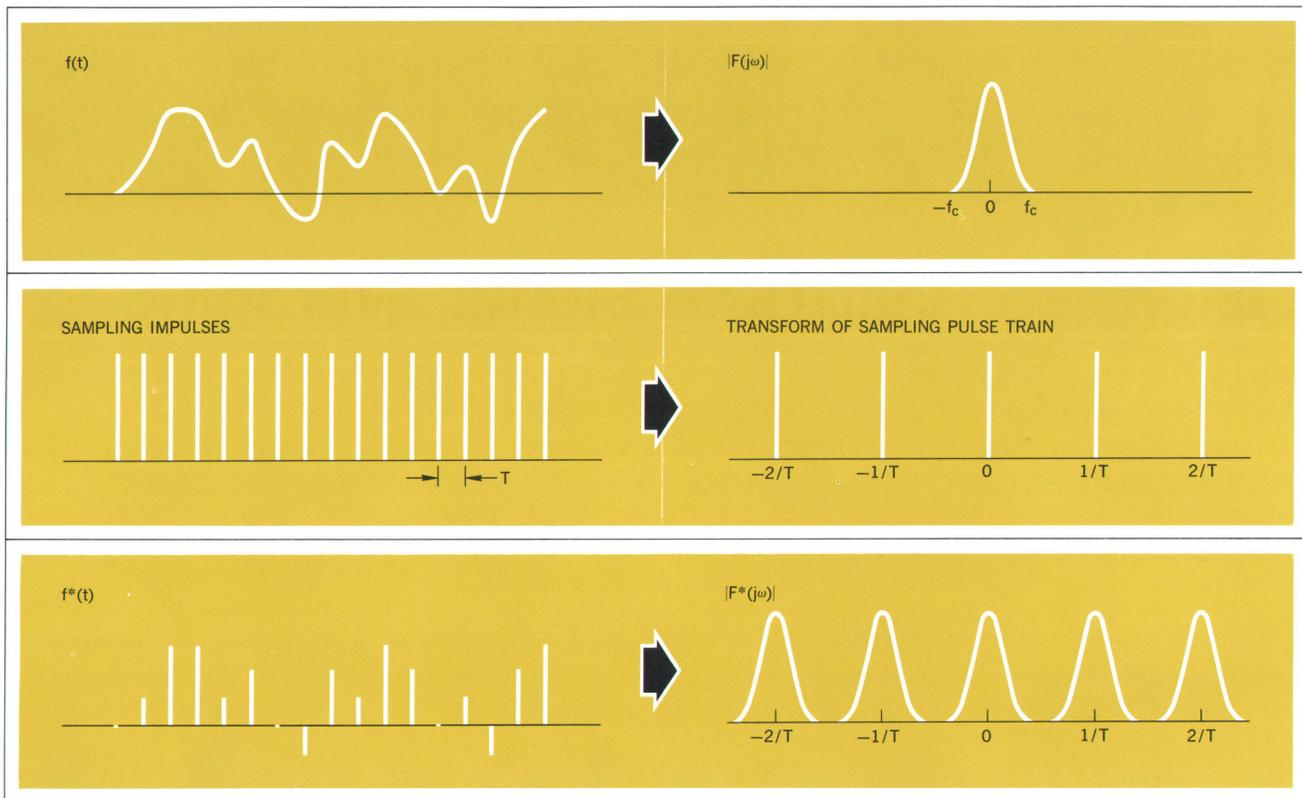
Fig. 5. Band-limited signal (top) sampled by infinite impulse train (middle) has frequency spectrum consisting of original spectrum duplicated at multiples of sampling frequency  $1/T$ . No information about signal is lost as long as duplicate spectra do not overlap, i.e., as long as  $1/T > 2f_c$ , where  $f_c$  is highest frequency present in signal  $f(t)$ .
