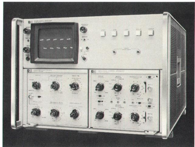
**Fig. 1.** New HP Model 5480A Signal Analyzer is an instrument that applies statistical principles to the on-line, real-time analysis of input data. The first two plug-ins make it a signal averager. Features include a display which doesn't flicker or grow off-scale during averaging, 100 kHz maximum sampling rate, memory of 1024 24-bit words, and ability to enhance slowly varying waveforms.
