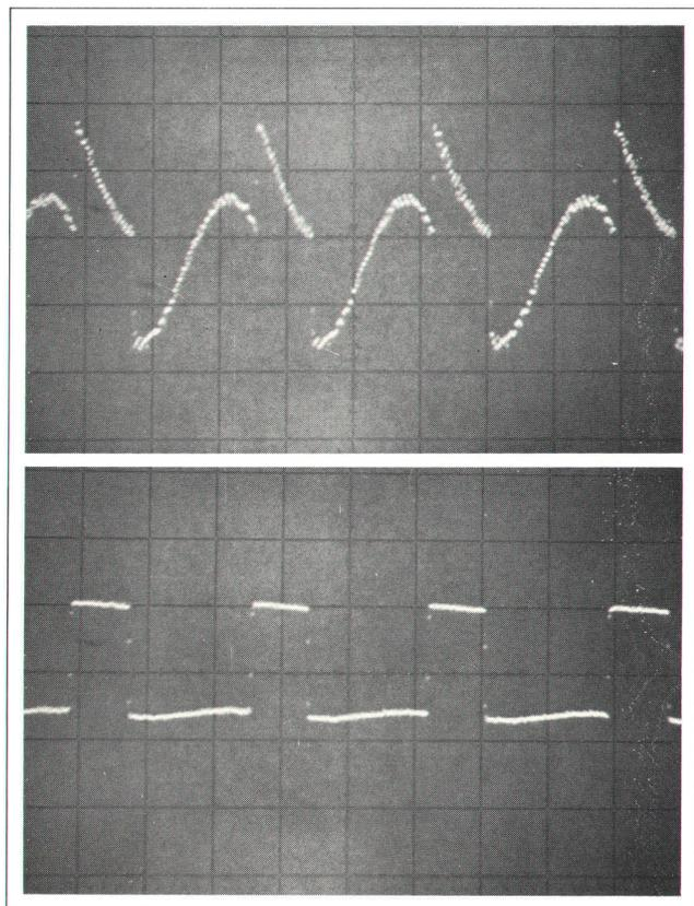
Fig. 4. Top: 200.0-Hz rectangular wave plus 200.1-Hz sine wave, before averaging. Bottom: 200.0-Hz rectangular wave recovered by signal averager after  $2^{14}$  repetitions. In this case, averager had the effect of a comb filter whose teeth had 3-dB bandwidths of 0.0027 Hz.
