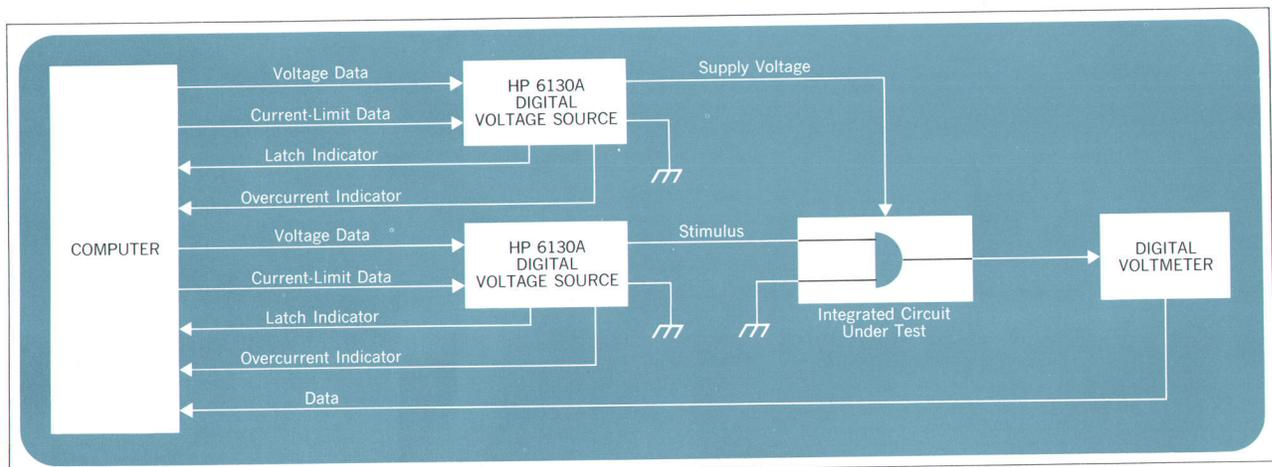
Fig. 1. Semiconductor Testing
