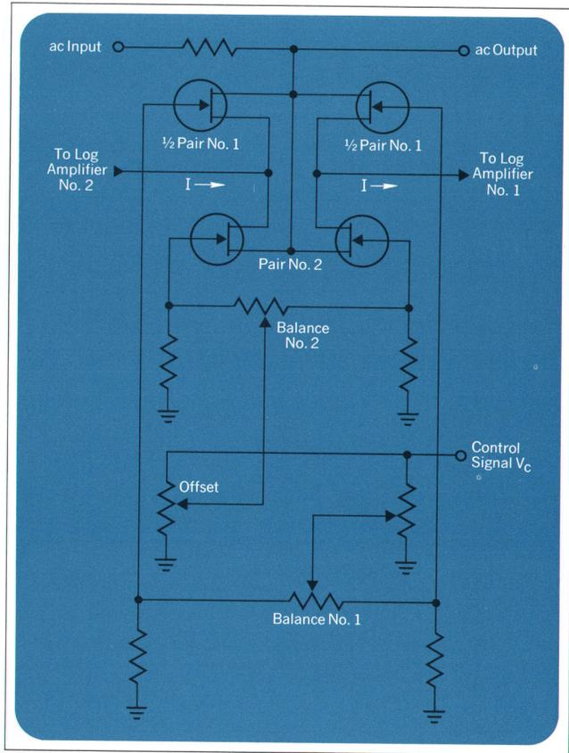
Fig. 7. Using field-effect transistors as variable resistors, the electronic attenuator can vary its resistance over more than an 80 dB range, from about  $30 \Omega$  to  $1$  M $\Omega$ , in response to a control voltage.
