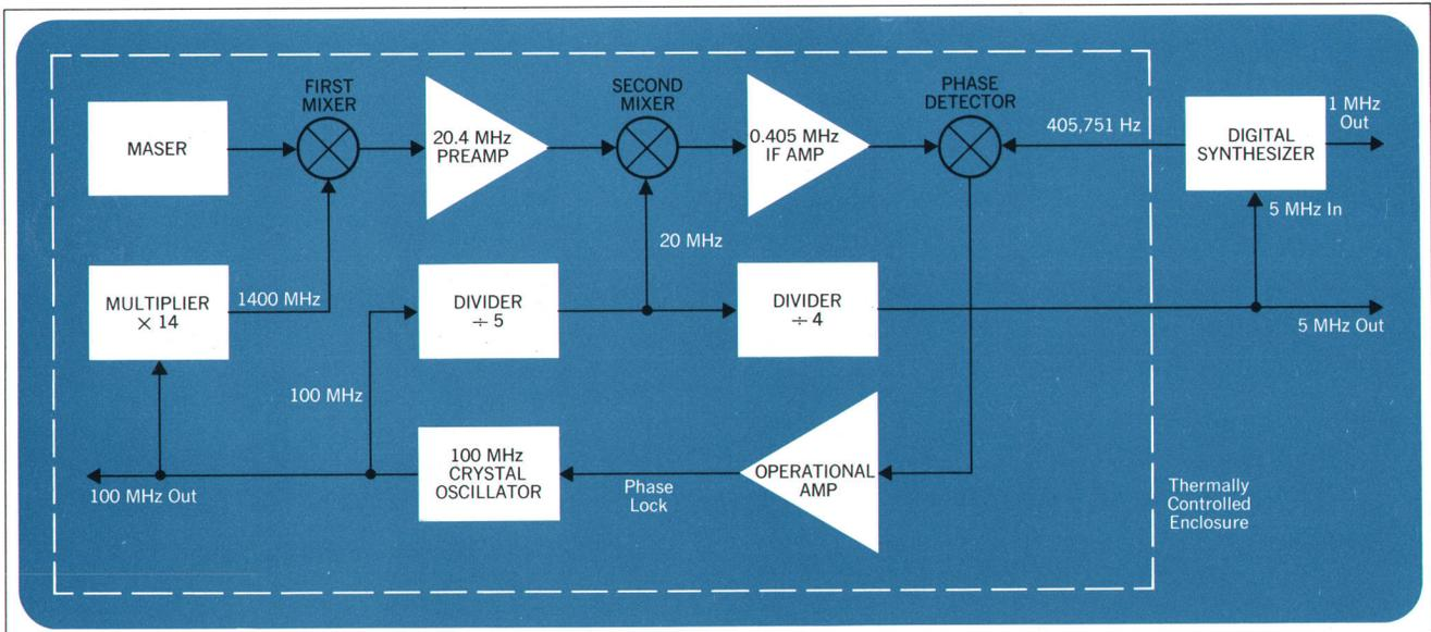
Fig. 4. The hydrogen maser's output frequency is 1420.405 751 786 4 MHz and its output power level is typically  $-97$  dBm. Here is a system for obtaining 100-MHz, 5-MHz, and 1-MHz outputs at useful power levels.
