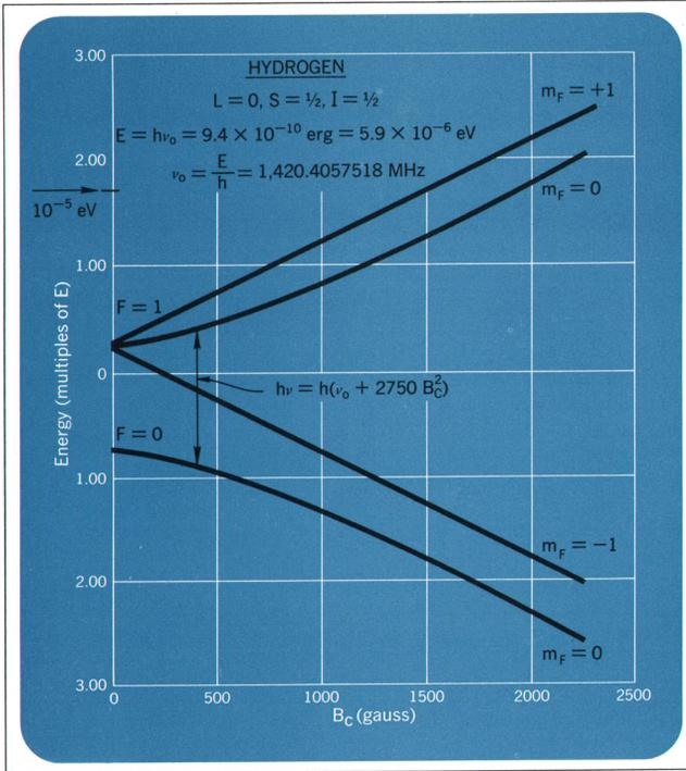
Fig. 3. In the hydrogen maser, the desired transition is from energy state  $F = 1, m_F = 0$  to energy state  $F = 0, m_F = 0$ . The energy of this transition, and therefore the maser's operating frequency  $\nu$ , depend upon the magnetic field  $B_c$ , so maser cavities are carefully shielded to eliminate stray fields.
