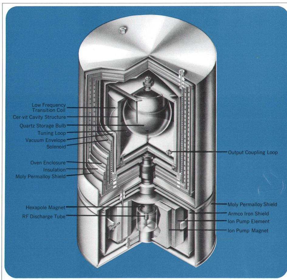
Fig. 2. In a hydrogen maser, atoms of hydrogen in certain energy states are directed magnetically into a teflon-lined quartz storage bulb inside a microwave cavity. The atoms stay in the bulb for nearly a second, some of them changing energy states and radiating energy at 1420 MHz. Maser oscillations occur when enough power is radiated by the atoms to overcome losses in the cavity.
