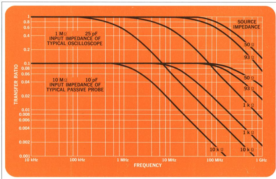
with a passive probe attached. These curves of transfer ratio versus frequency indicate less error when a high impedance probe is used, but sensitivity is reduced by a factor of 10.
