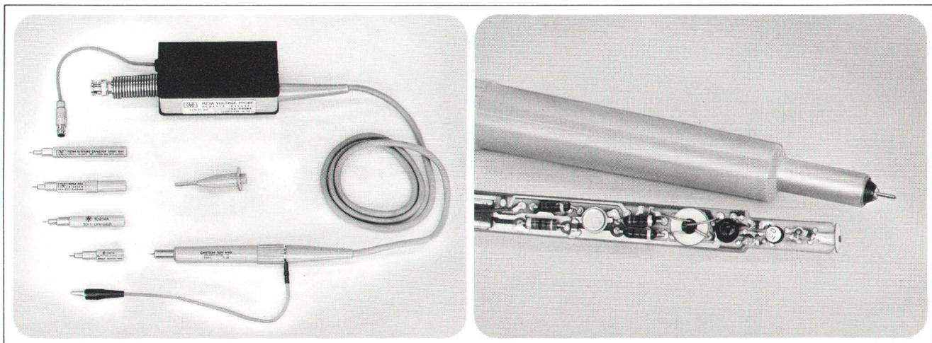
**Fig. 1.** Various tips (left) may be used with the HP Model 1123A Voltage Probe to increase dynamic range or ac couple the probe. The spring mounting of the amplifier assembly reduces the possibility of connector damage. **Fig. 2.** By mounting a FET in the probe tip and using miniature components, the input capacitance is kept low.
