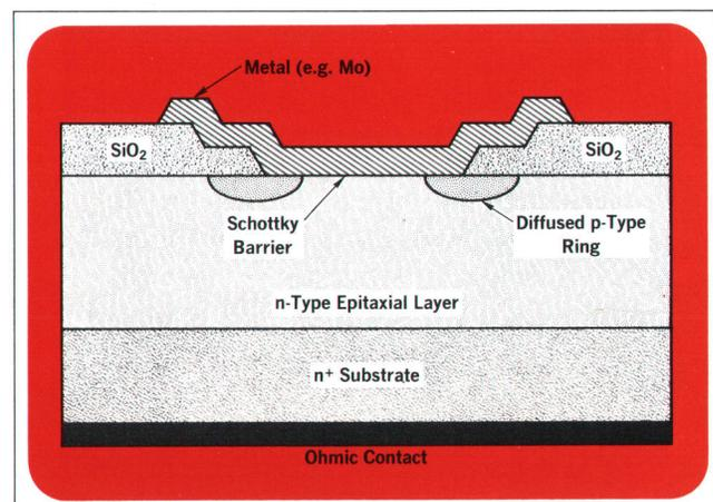
**Fig. 2.** Hybrid Schottky barrier diode has a diffused p-n junction guard ring under the metal and the passivating oxide layer. Proper choices of metal and diffusion profile give the new diodes high reverse breakdown voltages, low noise, and nearly ideal I-V characteristics.
