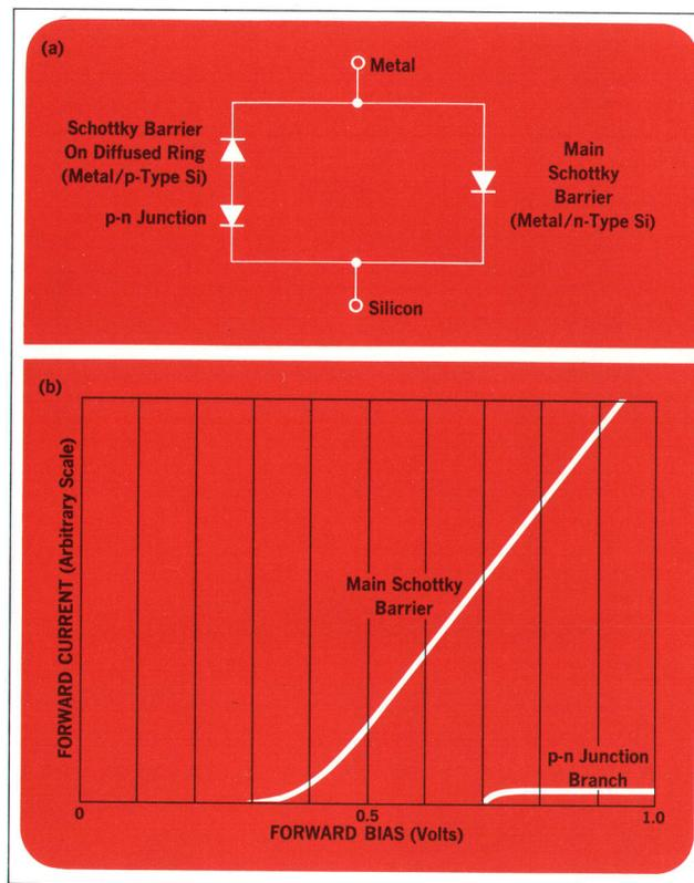
**Fig. 4(a)** Equivalent circuit of hybrid diode, assuming a rectifying contact between the metal and the diffused ring. Molybdenum/silicon and titanium/silicon hybrid diodes behave like this. The new HP 5082-2800 is a molybdenum/silicon diode. **(b)** *I-V* characteristics of the two branches in (a).
