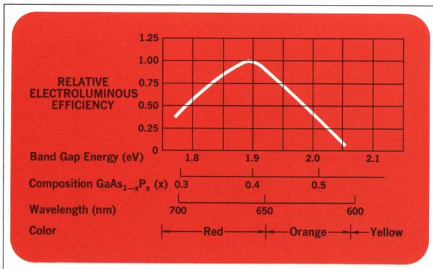
**Fig. 6.** Red was chosen as the color of the light emitted by the new solid-state indicators because the electroluminescent efficiency of HP's gallium arsenide phosphide alloy is highest for that color. Electroluminescent efficiency is a measure of visual brightness per unit diode current. It is a function of the alloy composition, that is, the value of  $x$  in the formula  $GaAs_{1-x}P_x$ .
