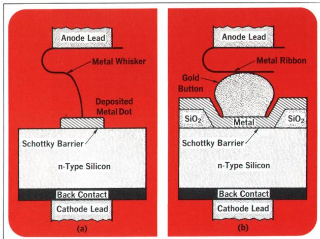
**Fig. 1.** Two types of Schottky barrier diodes that preceded the new hybrid type. (a) Unpassivated Schottky barrier diode is expensive to produce and has relatively low maximum storage temperature. (b) Passivated diode is less costly and has higher storage temperature, but has low reverse-breakdown voltage (typically 5 to 10 V).
