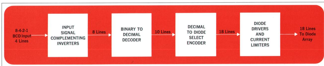
**Fig. 8.** The IC chip decodes BCD input signals into ten signals representing the digits 0 through 9. These signals are then encoded into signals which drive groups of diodes. There are 18 groups, and the diodes in each group are always lighted together. A two-step decode/encode process was chosen so the input code or character font could be changed simply by changing the interconnections between the logic elements.
