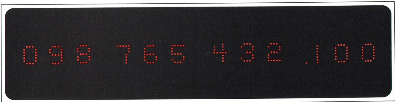
**Fig. 2.** The new solid-state indicators come in one-digit and three-digit modules. Here four three-digit modules display the full character font, which includes the numerals 0 through 9 and a decimal point.
