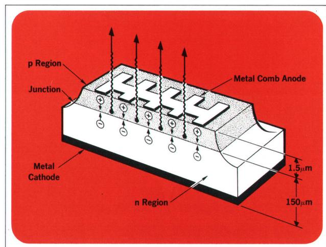
**Fig. 5.** Each light-emitting diode chip is a mesa-type p-n junction diode. Light is given off in recombinations of minority carriers, predominantly on the p side of the junction. The comb anode gives even current distribution while blocking less than 25% of the light.
