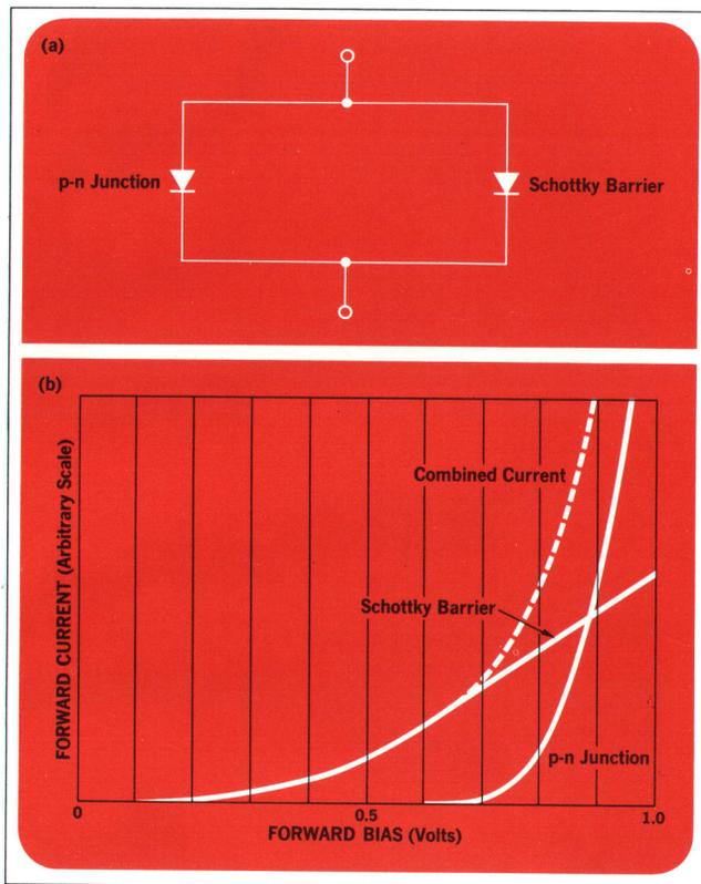
**Fig. 3(a)** Hybrid diode equivalent circuit, assuming the contact between the metal and the diffused ring is ohmic, or non-rectifying. **(b)** *I-V* characteristic expected from this structure. Shape is typical of gold/silicon and platinum-silicide/silicon hybrid diodes.
