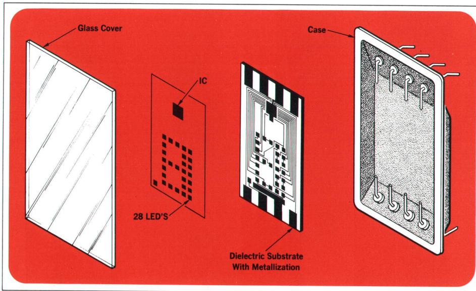
**Fig. 4.** Model 5082-7000 Solid-State Numeric Indicators consist of 28 gallium arsenide phosphide red-light-emitting diodes and an IC chip containing some 400 circuit elements, all mounted on a ceramic substrate and sealed in a case designed for wide-angle viewability. On the substrate is a metal interconnection pattern.
