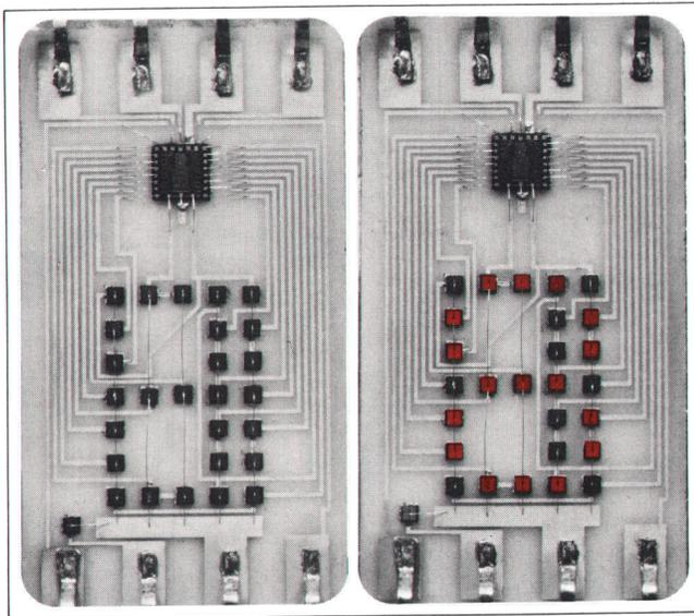
**Fig. 1.** Model 5082-7000 Solid-State Numeric Indicator accepts four-line BCD and displays any numeral from 0 to 9 in an array of bright red dots. It takes five-volt power and logic levels compatible with integrated circuits. Shown here is the bare module; mounted behind red glass, only the numeral is visible.
