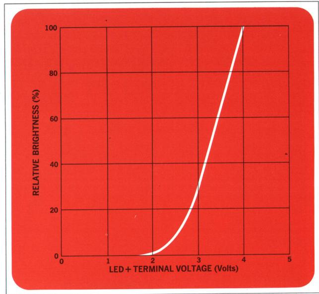
**Fig. 3.** The brightness of the solid-state indicators can be adjusted by varying the voltage applied to the LED + terminal of the module. Variable brightness and red color make the indicators useful in dark working environments.
