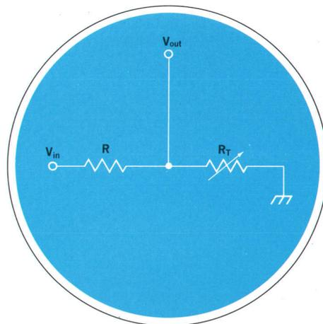
**Fig. 8.** To accurately determine the value of  $R_T$ , the ratio of  $V_{\text{out}}$  to  $V_{\text{in}}$  is more important than the absolute value of  $V_{\text{out}}$ . Accuracy is then independent of variations in  $V_{\text{in}}$ .
