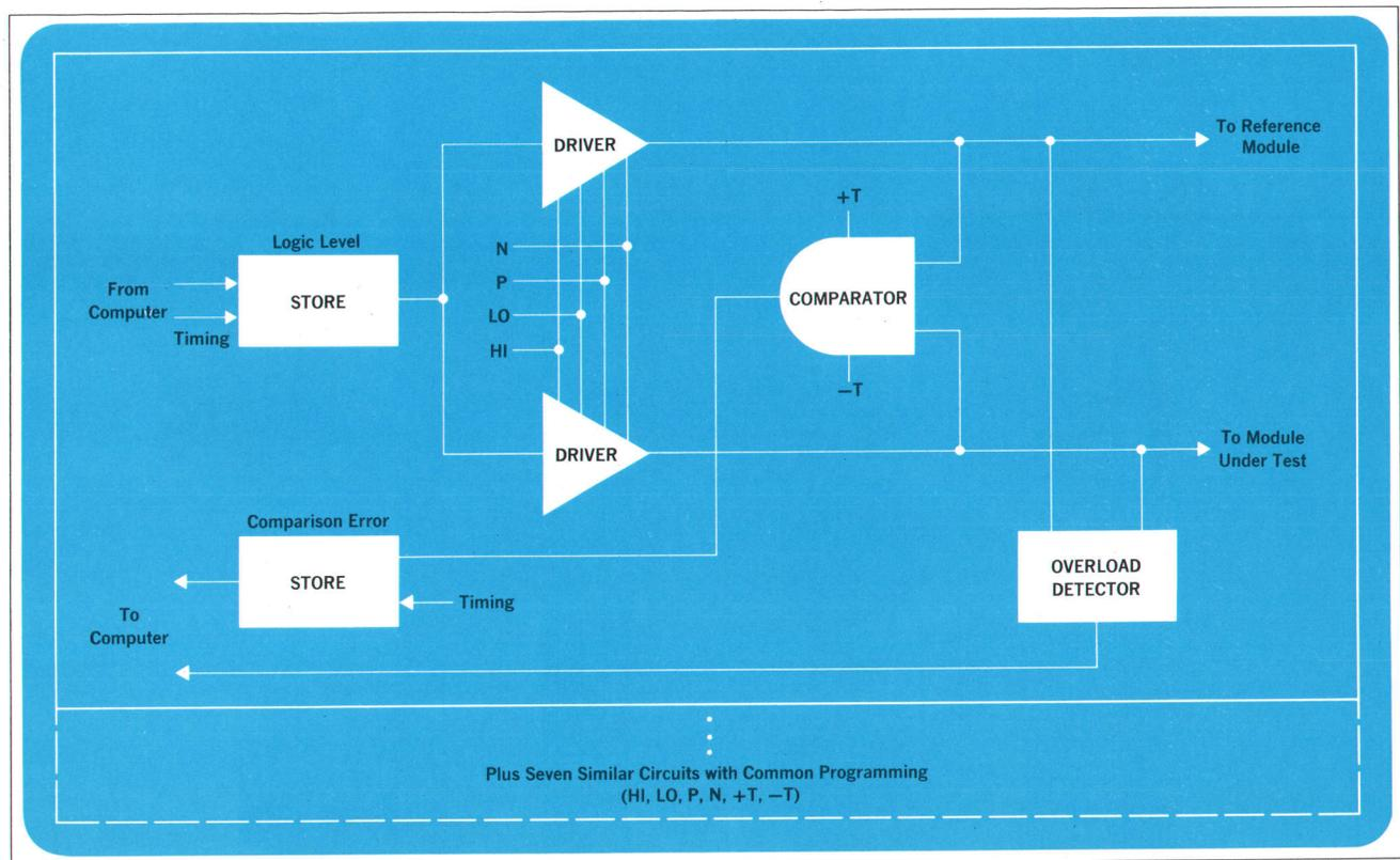
**Fig. 3.** The driver/comparator registers are the interface between the modules and the system. They have six programmable parameters: low and high logic levels, source and sink current limits, and plus and minus comparison tolerances.
