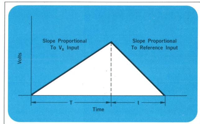
**Fig. 5.** (left) The dual-slope DVM compares an unknown voltage for a known time with a known reference voltage for a variable time. Thus the variable time is proportional to the ratio of the unknown voltage to the reference voltage, and is counted to determine the readout. **Fig. 6.** (right) Dual slope conversion technique averages the unknown voltage  $V_x$  over a known time  $T$ , but the ultimate conversion is voltage to time, or  $V_x$  to  $t$ .
