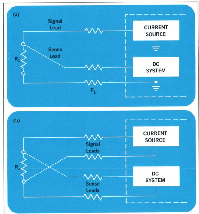
**Fig. 15.** (left) In each of these techniques for measuring unknown  $R_x$ , current  $I$  must be well controlled. **Fig. 16.** (right) A two or three-wire ohms measurement (a) includes the effect of lead resistance  $R_L$ . If the signal and sense leads are isolated (b),  $R_L$  is not included as a possible error source.
