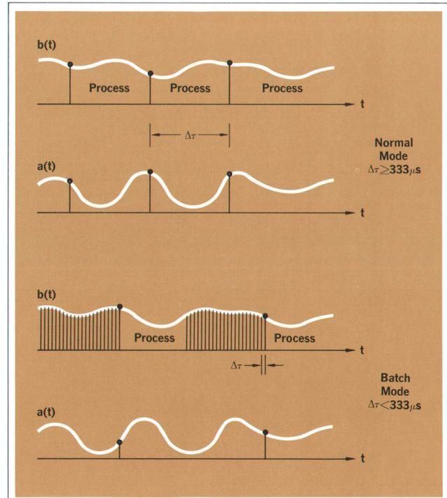
**Fig. 4.** For delay increments  $\Delta\tau$  (time/mm) of  $333 \mu\text{s}$  or more, the correlator operates in the normal mode, going through a process cycle — updating the 100 stored average products — after each sample of the inputs is taken. For shorter delay increments, the correlator uses the batch mode, taking 100 samples of input  $b$  for each sample of input  $a$ . Although much slower, the batch mode is used only at very short delay increments and isn't a practical limitation.
