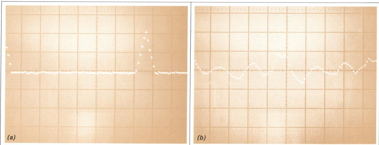
**Fig. 2.** Examples of 100-point correlation functions computed and displayed in real time by Model 3721A Correlator. (See also page 20 for autocorrelation functions of speech sounds.)
