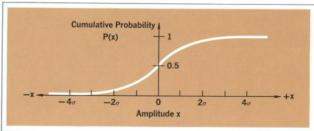
**Fig. 8.** Cumulative probability distribution function gives the proportion of time or probability that the signal lies below any given amplitude. It is the integral of the probability density function.  $P(-\infty)$  is always zero;  $P(\infty)$  is always one. This is the Gaussian distribution function.
