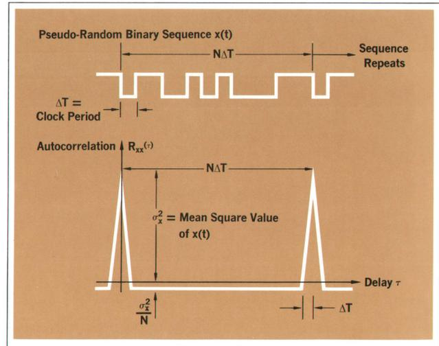
**Fig. 2.** The autocorrelation function is a measure of the similarity between a waveform and a shifted version of itself. Here is a pseudo-random binary sequence and its autocorrelation function. The autocorrelation function of a periodic waveform has the same period as the waveform.
