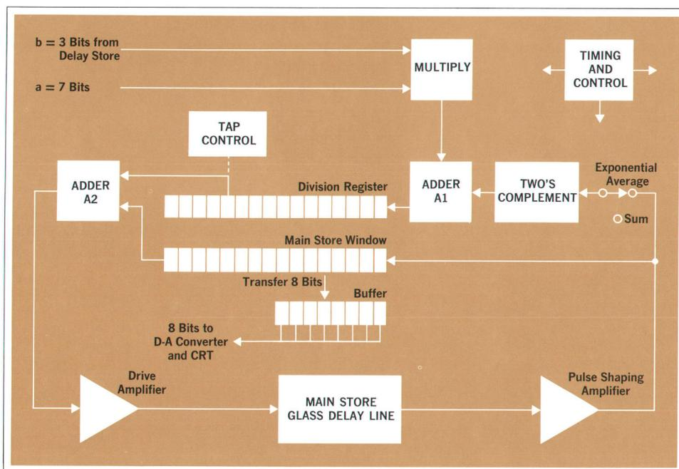
**Fig. 5.** The arithmetic unit computes averages digitally, so it doesn't have the stability problems of capacitive averaging. Multiplications and divisions, all by powers of two, require only time shifts.
