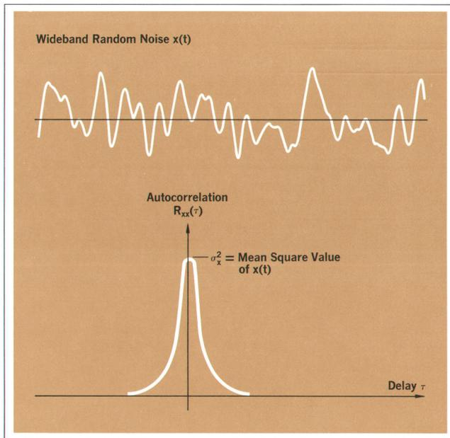
Fig. 3. The autocorrelation function of a wideband non-periodic waveform is non-periodic and narrowly peaked. The wider the bandwidth, the narrower the peak.
