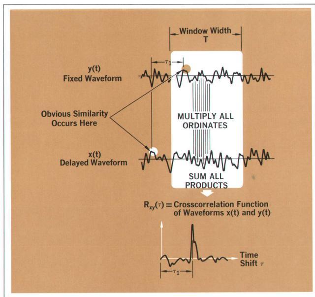
**Fig. 4.** Crosscorrelation function shows the similarity between two non-identical waveforms as a function of the time shift between them. Here the peak in the crosscorrelation function of  $x(t)$  and  $y(t)$  shows that at a time shift  $\tau$ , there is a marked similarity between the waveforms. The similarity is clearly visible in this example, but crosscorrelation is a very sensitive means of signal analysis which can reveal similarities undetectable by other methods.
