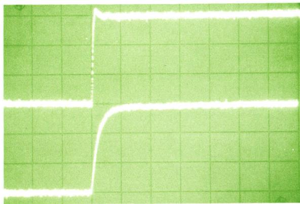
**Fig. 7.** Probe response with 10:1 voltage divider added to probe tip. Upper trace was made with Probe in 50Ω circuit. Lower trace was made in 1kΩ circuit and shows fast response time of Probe when used with divider to probe higher impedance circuits. (All scope photos were made with 4 GHz sampling scope.)
