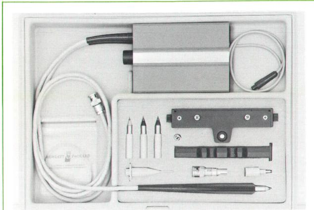
**Fig. 4.** Model 1120A 500 MHz Probe is supplied in kit with accessories, including 10:1 and 100:1 1-pF voltage dividers, 27-MHz bandwidth limiter, 2½ inch ground lead, hook tip, spanner tip, BNC adapter, and mounting brackets.
