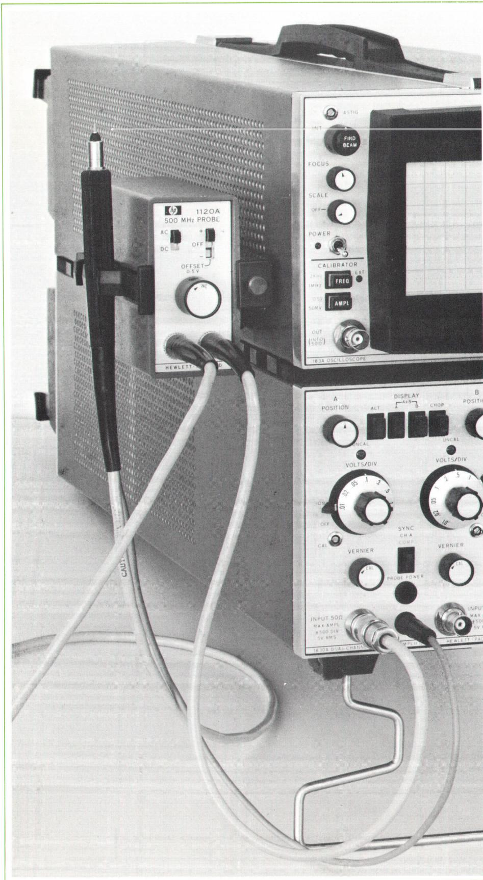
**Fig. 1.** New 500 MHz Probe connects to amplifier box through 4 ft. cable. Box mounts to side of instrument with versatile bracket supplied, and obtains power either from Probe Power jacks on instrument as shown, or from optional Probe Power Supply.
