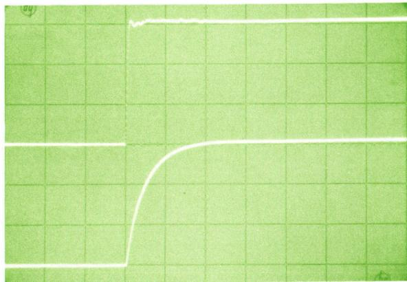
**Fig. 6.** Upper trace shows response of 500 MHz Probe to 0.35 ns, 300 mV step in circuit with 50Ω source impedance. Probe response time here is 0.75ns (sweep time: 10 ns/cm). Lower trace shows Probe response to same signal in circuit with 1kΩ source impedance.
