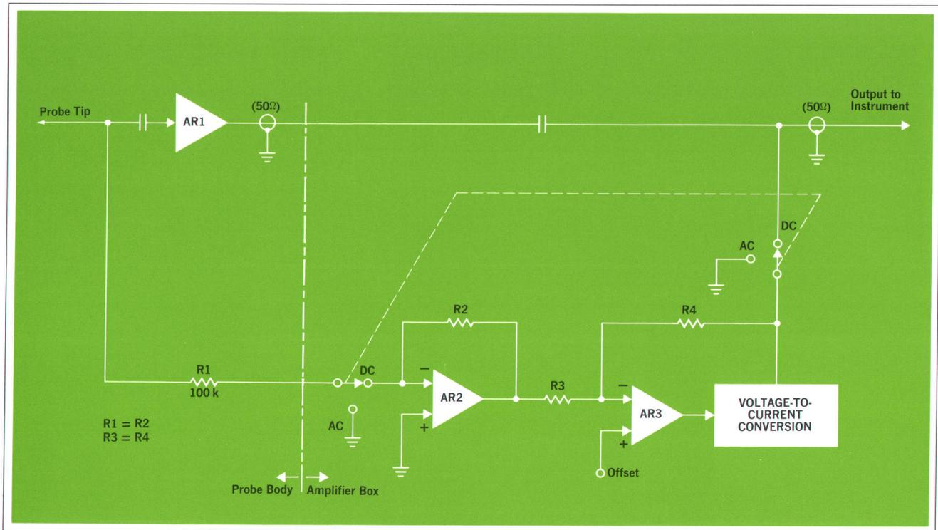
**Fig. 2.** Block diagram of 500 MHz Probe. AC path is through AR1, dc through AR2. AR3 compares outputs of AR1 and AR2 in lower part of frequency spectrum, reinserts low frequencies into output signal where AR1 output differs from AR2.
