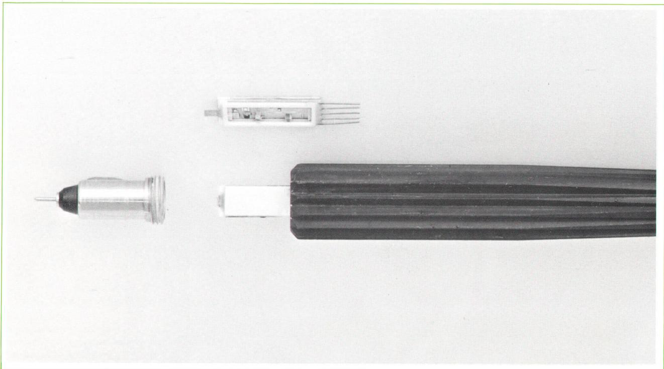
**Fig. 3.** Probe input is to hybrid microcircuit (rectangular unit shown detached at top). Probe tip connects to microcircuit, when installed at front of probe, through shock-absorbing contact which prevents damage to microcircuit.
