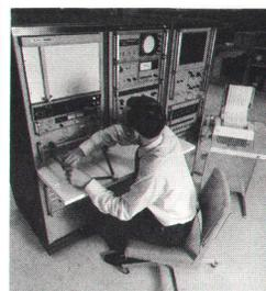
*Cover: Automatic network analyzer systems can vary widely, depending on the uses to which they are to be put. This one can show its findings on large-screen oscilloscope, on scope faces of more usual size, by teleprinter, and by X-Y plot. The power of these systems has produced a revolution in*
