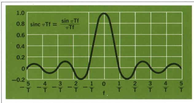
**Fig. 7.** Spectral lines of a sampled function will have this  $\sin x/x$  shape if the function isn't periodic in the record length  $T$ . Hanning weighting doubles the width of the main peak, but causes later peaks to fall off at 18dB per octave instead of 6dB per octave.
