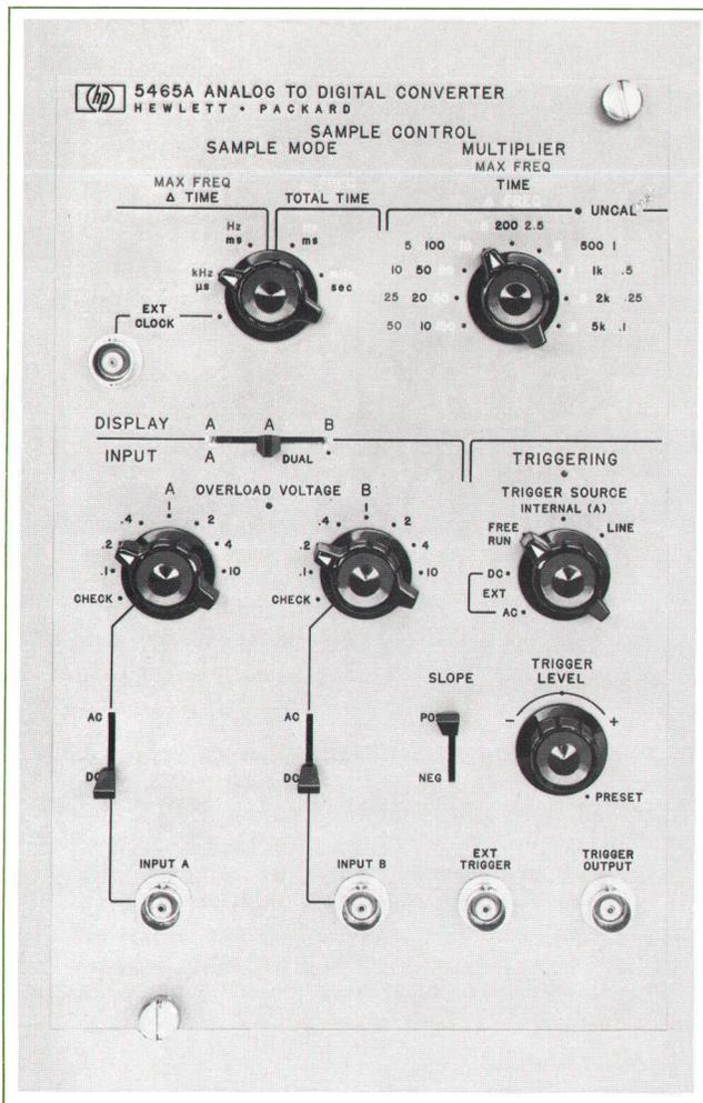
**Fig. 3.** Analog-to-digital converter is the principal input device for analog signals. It can be operated as a single-channel unit or a dual-channel unit. The maximum sample rate for single-channel operation is 20 μs per data point; the minimum rate is one sample in every five seconds. Data can also be read into the analyzer via peripheral devices, such as a tape reader or a teleprinter.
