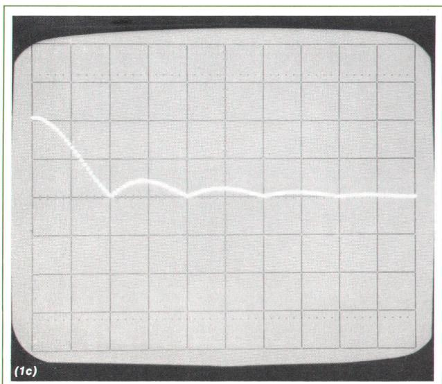
**Fig. 1.** The real parts of the Fourier transforms of two rectangular pulses which are identical except for a time shift are shown in (a) and (b). (c) is the magnitude of the Fourier transforms of both pulses. Because it is independent of time position, the magnitude-and-phase form of the transform is more useful than the real-and-imaginary form. However, the square of the magnitude, or the power spectrum, is even more widely used.
