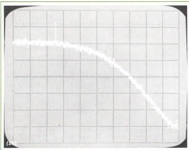
**Fig. 2.** The power spectrum (a) computed from a single sample record of a random signal is as random as the signal itself. But when 100 such spectra are averaged, the result (b) shows not only the spectral shape of the random signal, but also that there was a sinusoid hidden in the signal.
