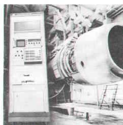
*Cover: Model 5450A Fourier Analyzer makes a variety of measurements fundamental to the analysis of waveforms and time series. Among its many uses is analysis of sound and vibration, symbolized here by a jet engine mounted in a test chamber. We are grateful to United Air Lines for allowing their engine to pose for us.*
