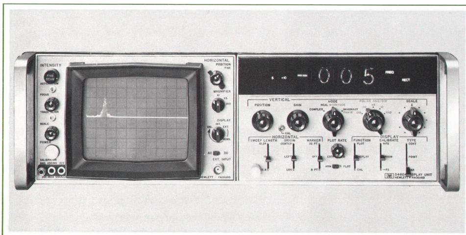
**Fig. 4.** Built-in display unit is the principal analyzer output device when the recipient of the data is human. The digital display and annunciation indicate the vertical scale factor and the type of display. Data in the analyzer are always absolutely calibrated.
