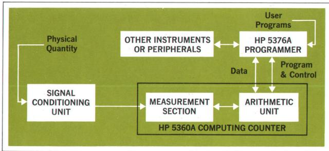
**Fig. 1.** Computing-counter systems, like computerized systems, can make measurements and arithmetically manipulate the data resulting from the measurements, all under program control. Applications are in data reduction, statistical analysis, process control.
