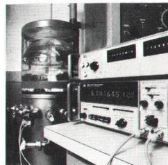
*Cover: Crystal plating is a typical process-control application for the 5360A Computing Counter and its new Programmer, Model 5376A (on top of the computing counter). See page 5 for a more complete description.*
