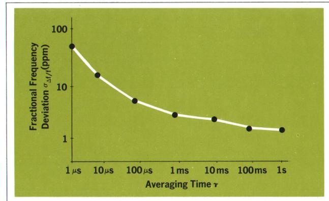
Fig. 4. Short-term stability of an oscillator. The computing-counter system can be programmed to make the frequency measurements and perform the computations needed to obtain a direct readout of  $\sigma_{\Delta f/f}$ .
