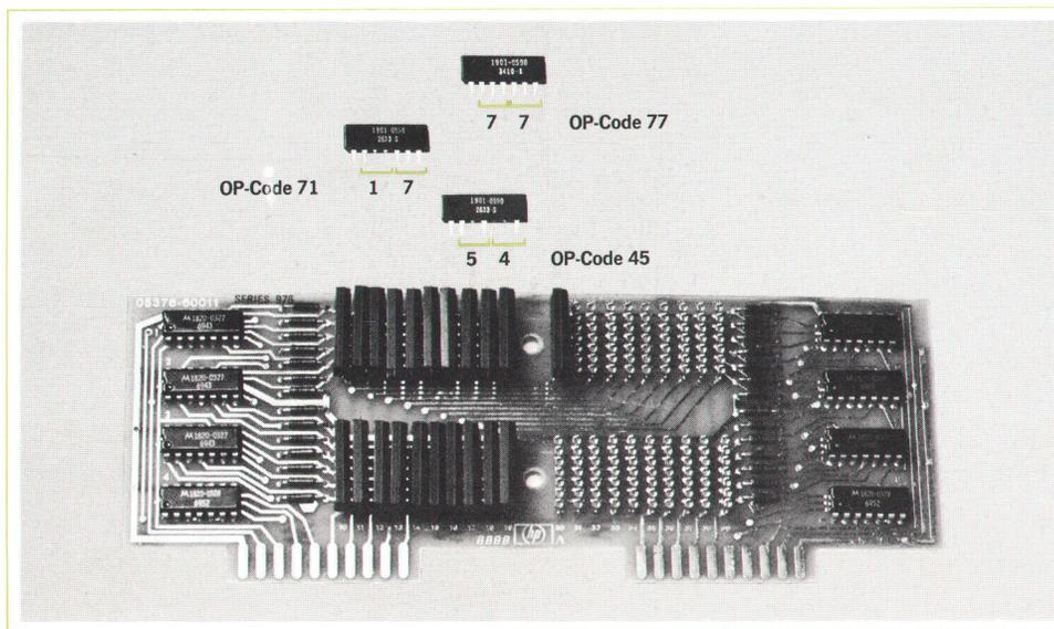
**Fig. 3.** When diode programming is used (rather than punched card), program instructions are coded by clipping leads off diode packages which are then plugged into program boards as shown. Programmer comes with one 40-instruction program board and can accommodate four more.
