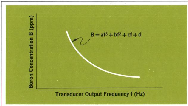
Fig. 3. Transducer transfer function relating boron concentration to transducer output frequency. Computing-counter system can solve this equation and display boron concentration directly, like a 'boronmeter.'
