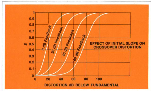
Fig. 14. Effect of initial slope on crossover distortion.
