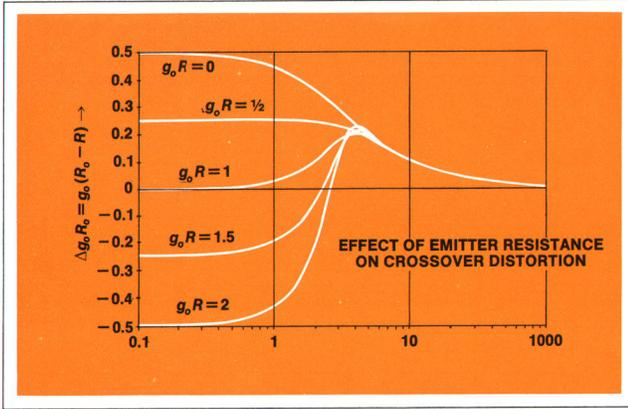
Fig. 6. Effect of emitter resistance on crossover distortion.
