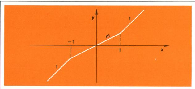
Fig. 8. Transfer characteristic of entire nonlinear stage.
