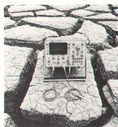
**Cover:** Dry lake bed dramatizes ability of new 1700-series Oscilloscopes, operating on optional internal battery pack, to bring lab scope performance anywhere it may be needed. Up to 75 MHz response, dual trace display, and delayed sweep can all be had where ac line power can't. And since these cool-running instruments need no fan or ventilating holes for circulating air, dusty or other hostile environments pose no special problems.
