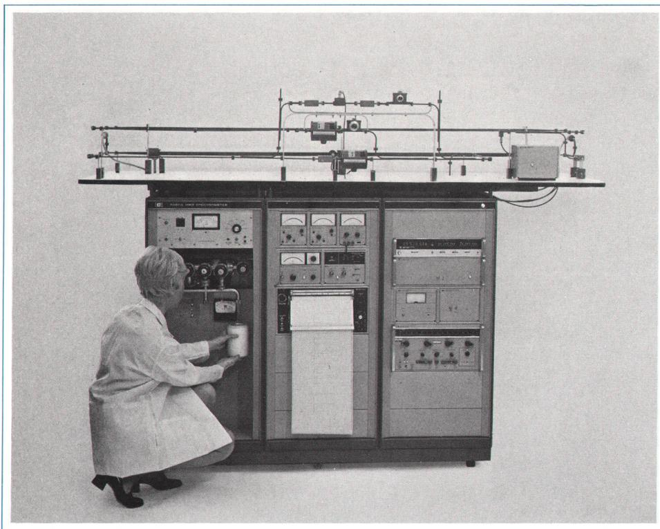
**Fig. 1.** New HP 8460A MRR Spectrometer is the first rotational microwave spectrometer that's really easy to operate. 'Table tops,' which hold all the microwave circuitry already mounted and ready for use, make it easy to change frequency bands.
