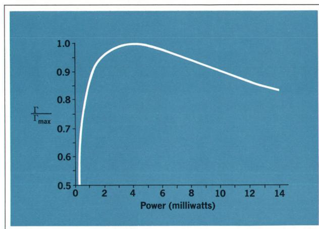
**Fig. 10.** Intensity coefficient  $\Gamma_{\max}$ , readily measured with an HP 8460A MRR Spectrometer bridge option, is a measure of the partial pressure of a mixture component independent of mixture composition. It's useful for quantitative mixture analysis.
