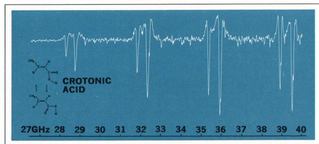
**Fig. 8.** The two conformations of crotonic acid shown here are impossible to separate chemically, but the band spectrum clearly shows two series of bands, one for each conformation. This is why rotational microwave spectroscopy is valuable for determining molecular structure, its principal use to date.
