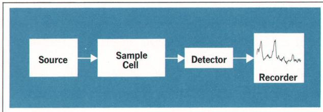
**Fig. 2.** Like all spectrometers, the HP 8460A has four basic parts: a source of radiation, a sample cell where the radiation interacts with the sample, a detector to monitor the power absorbed by the sample and a recorder to plot absorbed power versus frequency.
