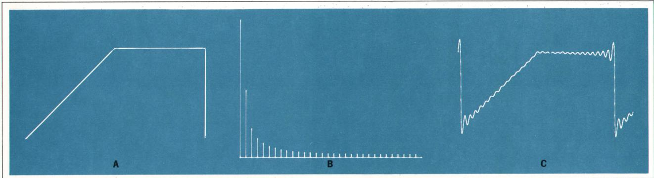
**Fig. 2.** The time function (A) is digitized, and the frequency spectrum (B) is the resulting plot of the Fourier analysis. Plotting the reconstructed  $f(t)$  from the computed coefficients gives an approximation of the original time function (C).
