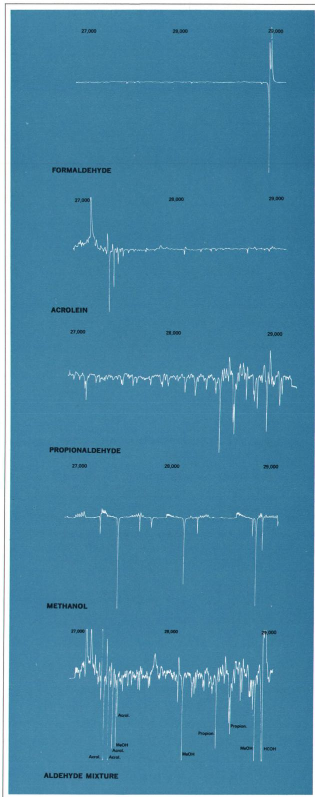
**Fig. 6.** Mixture analysis—qualitative and quantitative—is an important application of high-resolution rotational microwave spectroscopy. For example, given the individual spectral fingerprints of these four compounds it's easy to spot them in the mixture.
