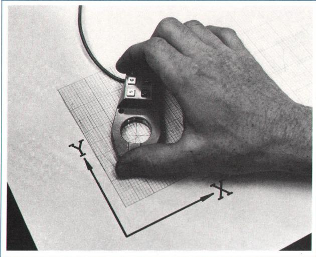
**Fig. 1.** In using the Model 9107A Digitizer, the graphic data to be analyzed is placed on the platen. The cursor is placed over the chart and the curves traced as shown. Coordinate pairs under the cross hairs are automatically entered into the X and Y registers of the Model 9100 calculators.
