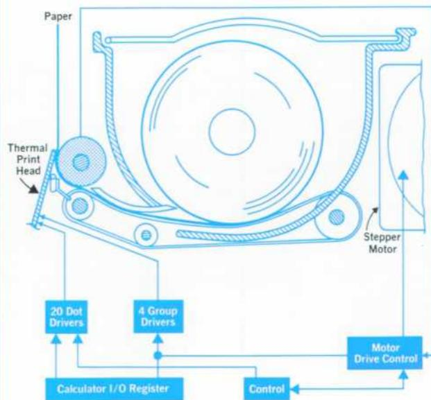
Fig. 1. Thermal printer has few moving parts.
