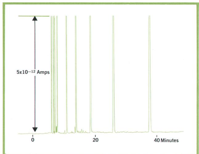
**Fig. 11.** Chromatogram generated by 5700A Gas Chromatograph using new FID shows low amount of noise on baseline (sample was *n*-paraffin blend using 150-foot capillary column with instrument set to Range 1, Attenuation 1).
