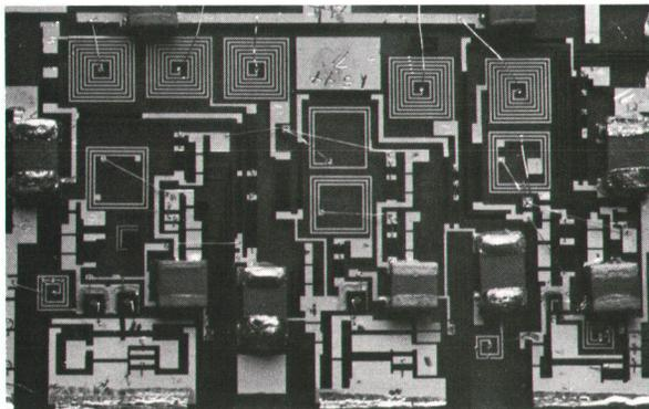
A key element in making 1.3 GHz performance possible in the Model 8660A/B Synthesized Signal Generator, and in several other instruments as well, is the hybrid integrated circuitry like that shown above.
