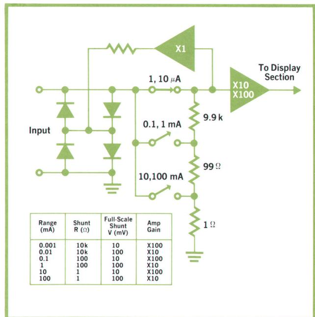
**Fig. 3.** In milliammeter mode, shunt resistors develop voltage proportional to current for measurement by Display section. Diodes bypass current at times range switches may be open during ranging. During measurement, upper pair of diodes are boot-strapped to current-derived voltage to prevent leakage of current around shunts.
