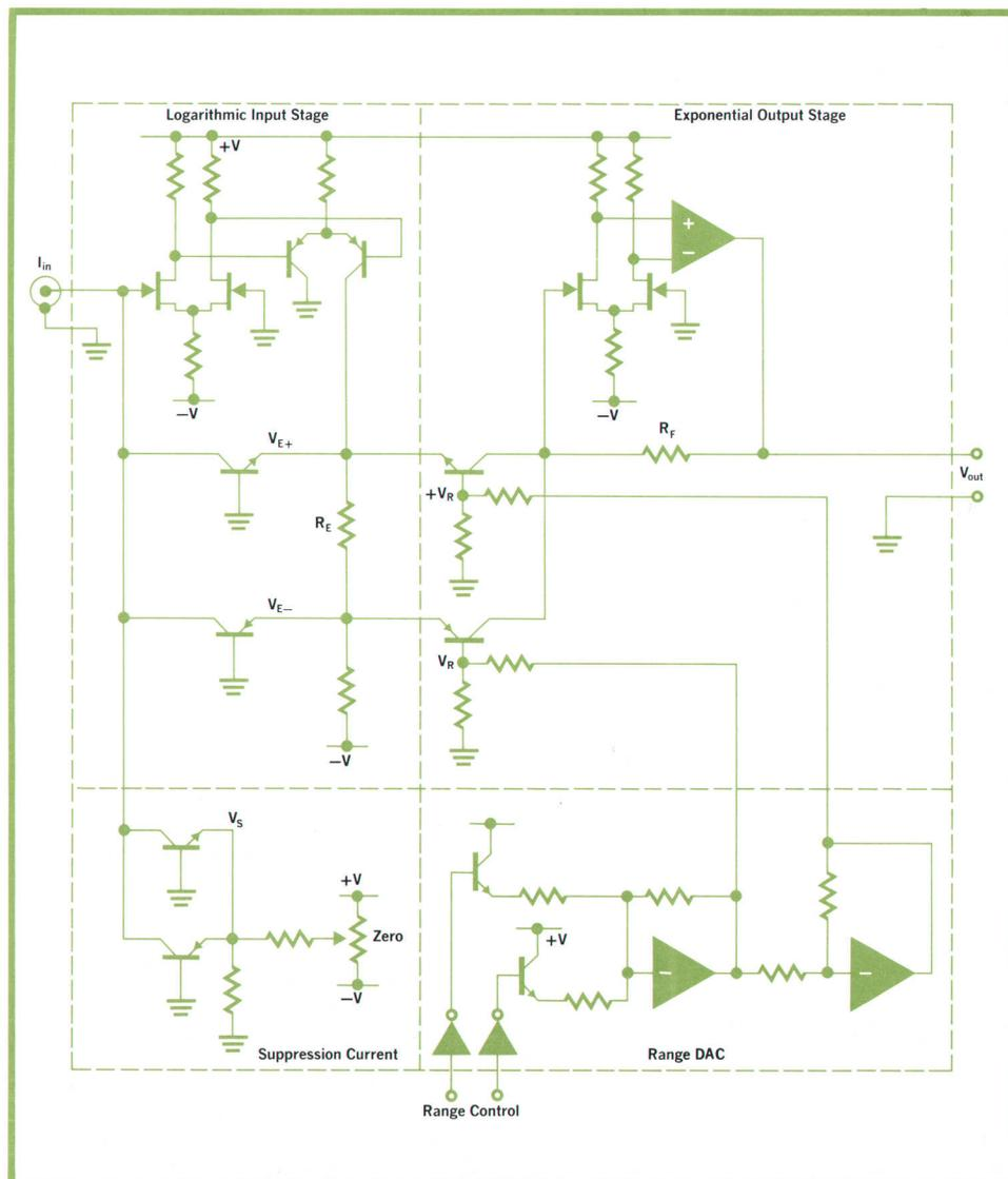
**Fig. 6.** Simplified schematic drawing of electrometer circuit. Matched pairs of NPN and PNP transistors permit bipolar operation. Constant voltage drop across  $R_E$  overlaps plus and minus inputs to log amplifier about  $10^{-13}A$  to maintain fast response around zero input current. Range control input can be contact closures or standard 5-volt logic levels.
