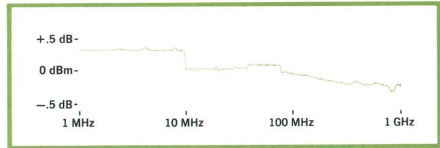
**Fig. 4.** Frequency response plotted at 0 dBm output level.
