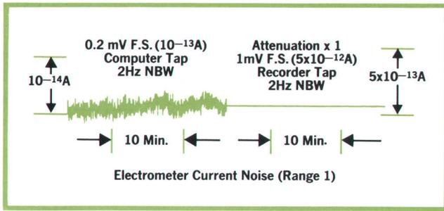
**Fig. 7.** Electrometer noise is not visible on recorder trace during normal operation of instrument on most sensitive range. Expanded scale portion (left half) shows noise to be about  $3.5 \times 10^{-15}$  A peak-to-peak.
