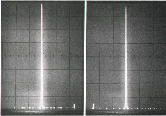
**Fig. 6.** Spurious outputs always lie outside  $\pm 50$  MHz band centered on output. Fifth-order spurious output is 50 MHz above output frequency of 999.999 MHz (left photo) but jumps to 50 MHz below when output is stepped to 1000.000 MHz (right photo).
