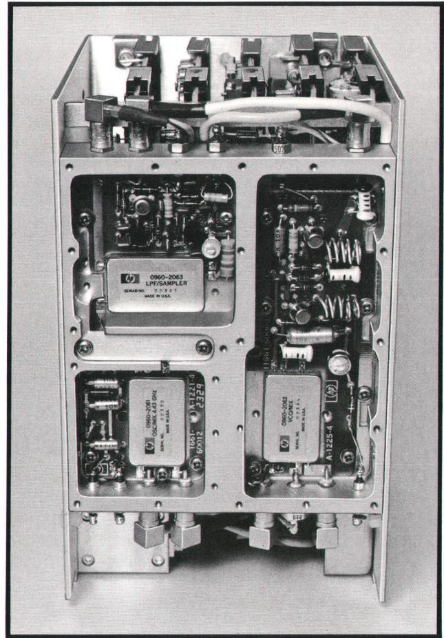
**Fig. 12.** Thin-film hybrid microcircuits (rectangles with HP insignia) are mounted in Frequency Extension Module on printed-circuit boards in same way as conventional components. Signal transfer in and out of microcircuits is by way of strip-line transmission lines, eliminating coaxial lines and space-consuming connectors. Electromagnetic isolation between circuits is provided by walls in solid metal casting.
