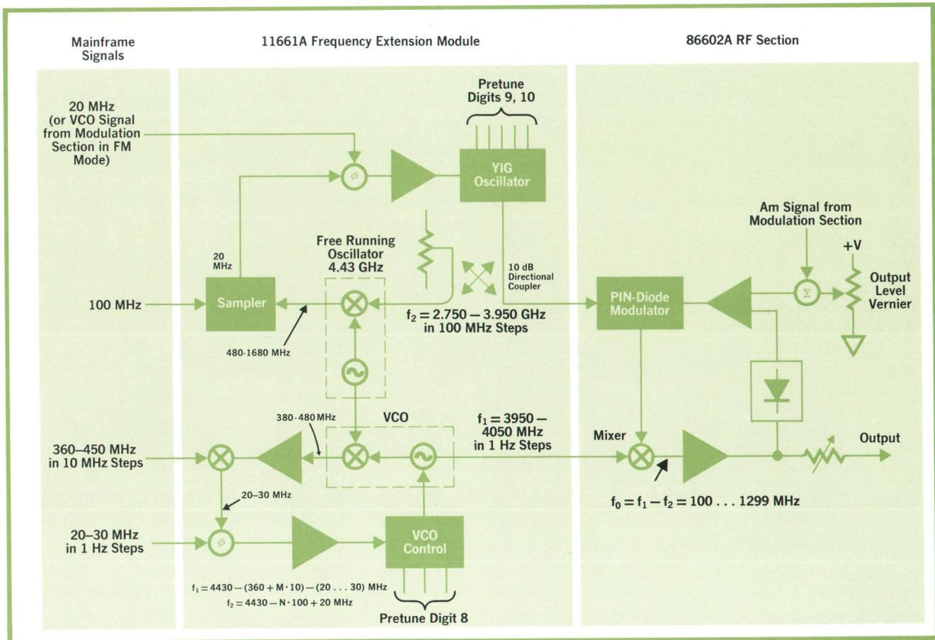
**Fig. 2.** Block diagram of 1-1300 MHz frequency generation. YIG oscillator is tuned in 100 MHz steps by digital control signals, then locked to mainframe 20-MHz reference through chain of frequency conversions in phase-lock loop. VCO is locked to mainframe frequency derived from choice of 1-Hz-to-10-MHz frequency-selection digits. Output frequency is difference between YIG and VCO frequencies.
