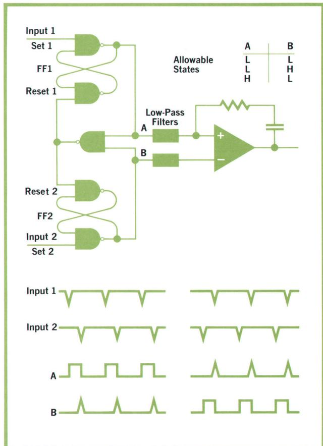
**Fig. 7.** Phase-frequency detector, useful with inputs up to 50 MHz, has high-speed Schottky TTL gates in three-state logic configuration. Waveforms show how outputs proportional to phase difference are generated.
