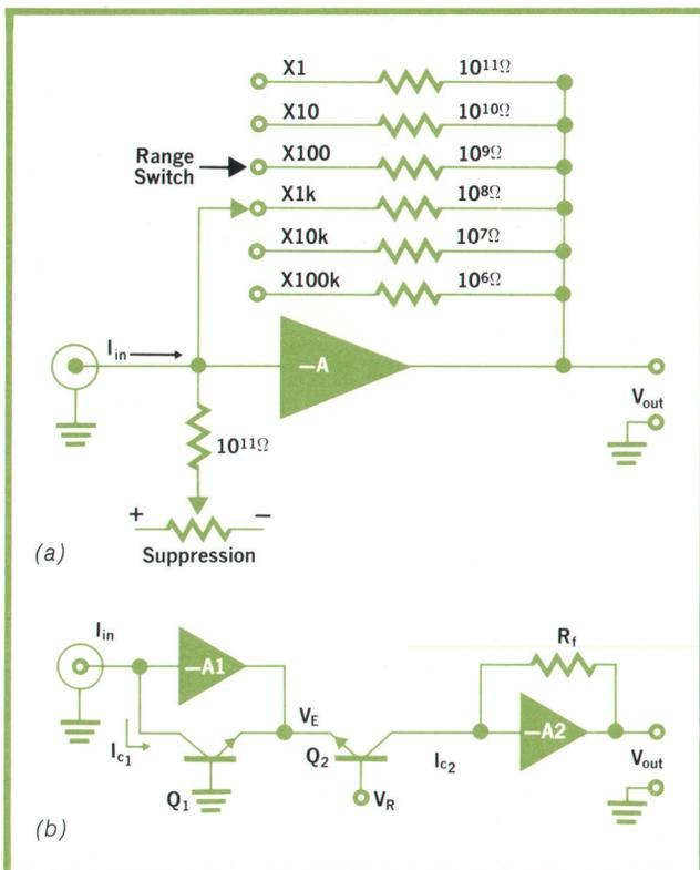
Fig. 4. Conventional electrometer (a) switches feedback resistors to change range. Ranges are changed on new electrometer (b) by switching voltage input,  $V_R$ , to exponential-responder transistor Q2.
