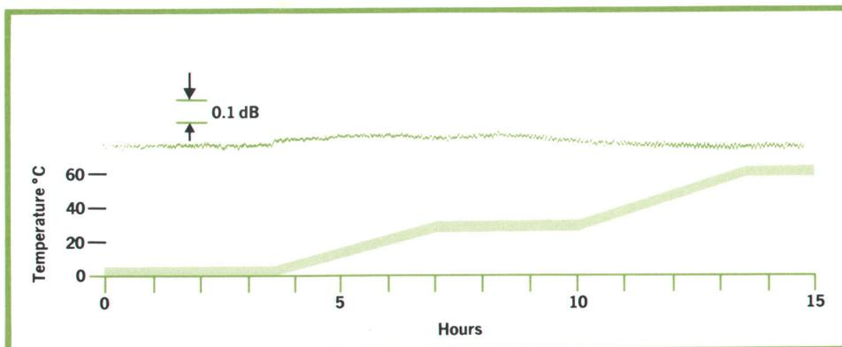
**Fig. 5.** Output level stability in varying ambient temperature. Lower trace shows temperature profile of environmental chamber in which test was made. Noise-like variations in output result from  $5^\circ$  temperature variations caused by chamber's on-off heat control system.
