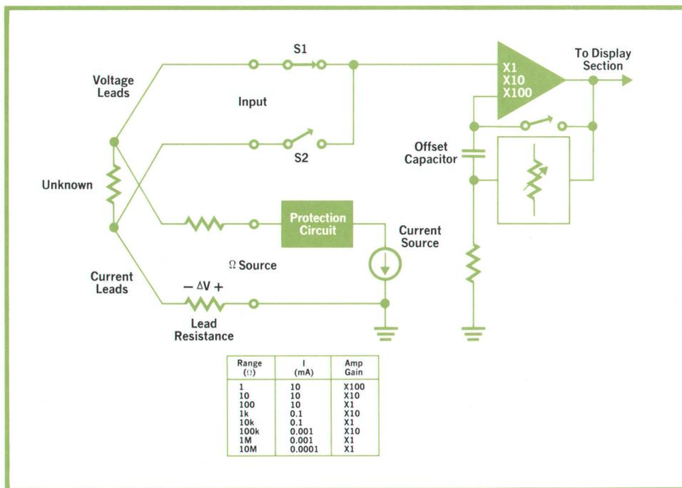
**Fig. 4.** In ohmmeter mode, current through unknown develops voltage proportional to resistance for measurement by Display section. Just prior to measurement cycle, S1 opens and S2 closes. Voltage  $\Delta V$  resulting from current through lead resistance is stored on offset capacitor. During measurement, offset voltage is subtracted from measurement voltage, eliminating effect of lead resistance on measurement.
