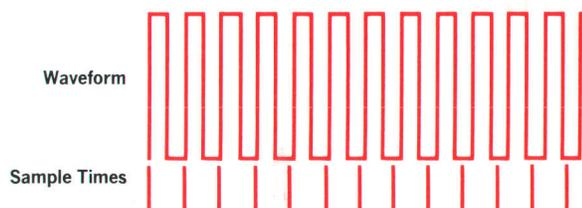
For a given upper sampling rate, a slightly higher signal frequency can be handled if the samples are taken over 32 cycles rather than 31. Even so, the input frequency is limited to about 1030 Hz unless cycles are skipped between samples:
