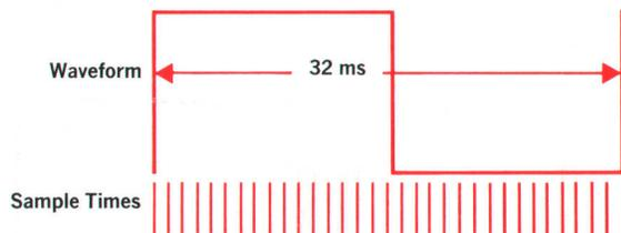
If the waveform of interest has a frequency higher than 31 Hz, the system uses a sampling-oscilloscope approach, taking 32 samples over more than one period of the waveform. The simplest case consists of 32 successive cycles of some repetitive waveform, as shown below. It can be seen that each successive sample falls a little later in the cycle (by  $1/32$  of a cycle).
