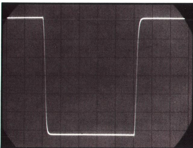
**Fig. 3.** Oscillogram shows clean response of new current sources to changes in output level. Initial output level was  $+160$  mA; the instrument was then programmed across its full output range to  $-160$  mA, then back to  $+160$  mA. Oscilloscope sweep speed is  $100 \mu\text{s}/\text{cm}$ .
