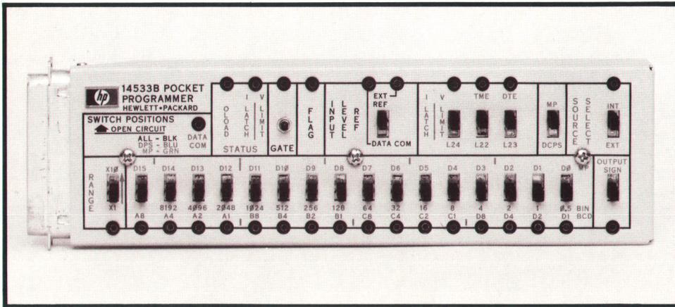
**Fig. 7.** Pocket programmer, shown here without interconnecting cable, enables the Model 6140A Digital Current Source to be operated manually for off-line service and calibration or for use on the lab bench. Programmer operates all the Current Source input functions by switch closures.
