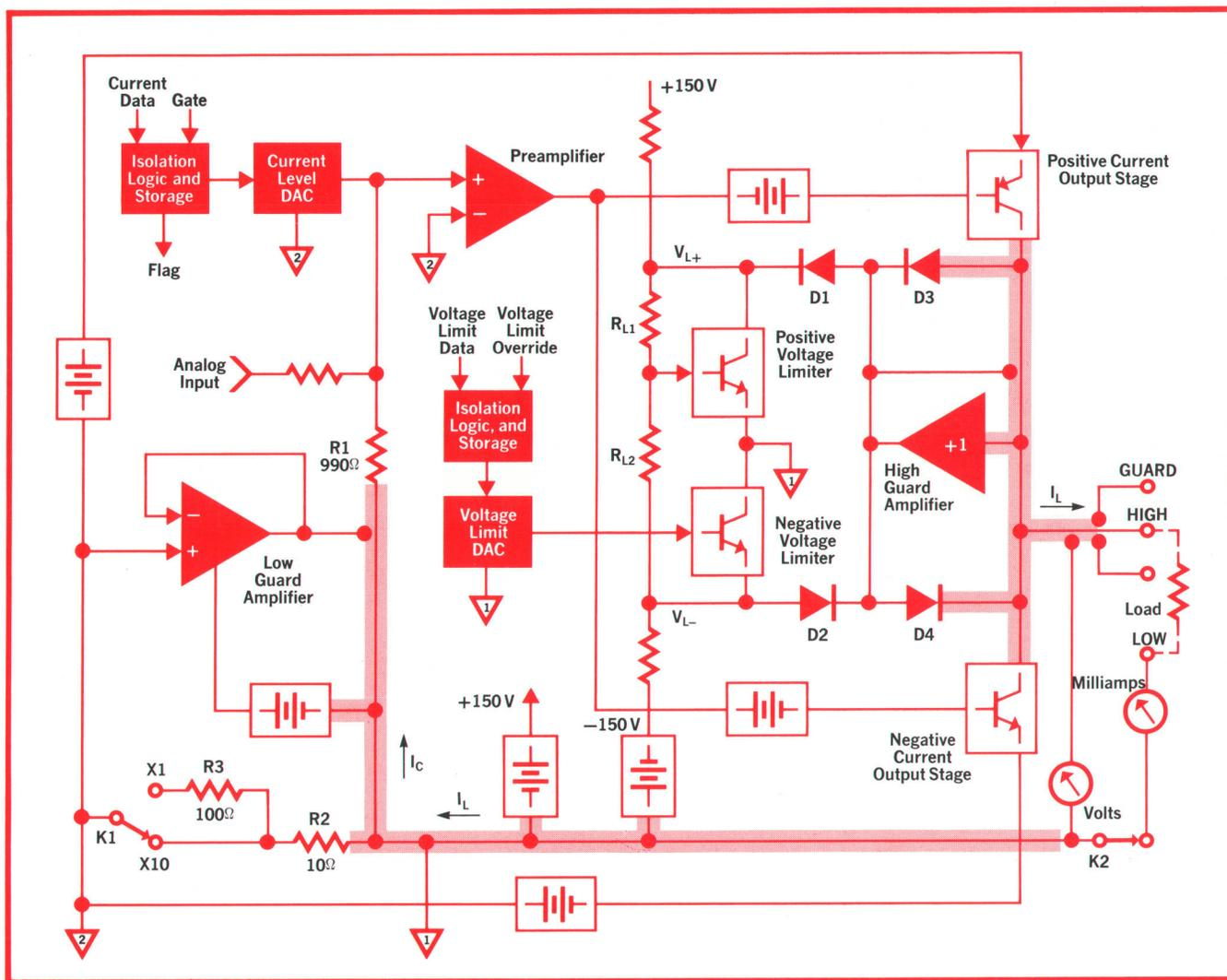
Fig. 6. Block diagram of new Digital Current Source.
