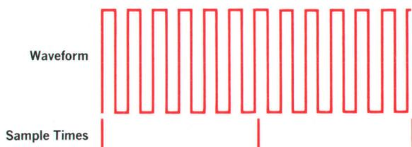
To measure a 2 kHz waveform, 32 samples can be taken over 64 (or 63) cycles. At the upper 9540 System frequency specification of 6 kHz, the 32 samples are taken over at least 191 cycles of the waveform.
