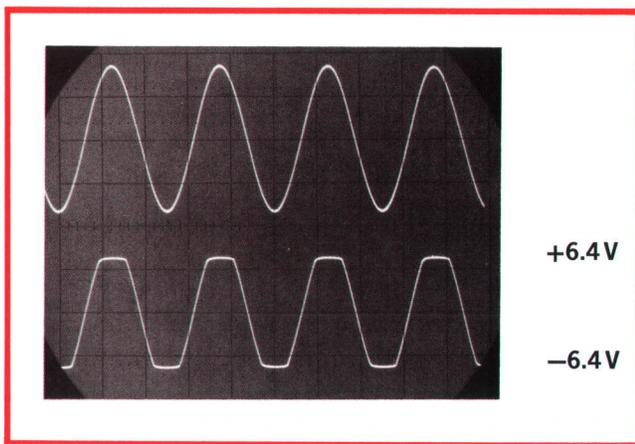
**Fig. 5.** Effect of voltage limiting is shown by this oscillogram. Upper trace shows 11.5 V p-p output of the current source in response to a sinusoidal waveform at the analog input. In the lower trace, the voltage limiters have been set to  $\pm 5$  V, resulting in hard limiting at 1.4 V beyond the selected level.
