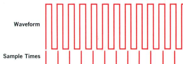
An equally valid approach is to sample 32 times over 31 cycles, as shown below. Here, each sample falls a little earlier on each successive cycle.
