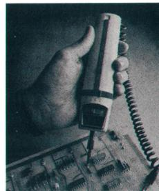
**Cover:** *The hand-held digital multimeter—a concept that's been in the back of many an engineer's mind ever since integrated circuits went large-scale—has become a reality. Doing it required more than an integrated circuit, however; it required a combination of technologies as described here. (Zero is added to 3-digit display here to indicate range.)*
