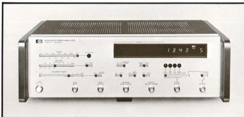
**Fig. 1.** Model 1645A Data Error Analyzer generates digital test patterns in its transmitter section, transmits the patterns through a communications channel, and analyzes the received patterns in its receiver section by comparing them to locally-generated patterns. It analyzes the patterns six ways simultaneously.
