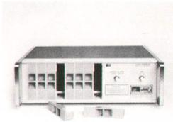
Controller contains the electronics to transfer data to and from the mass memory.
