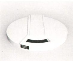
Each cartridge provides 2.4M bytes of storage. In addition, 7K of system software resides on each platter after it is formatted for system use.
