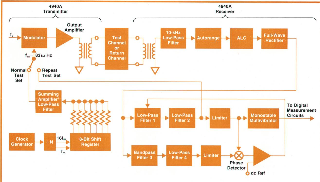
Fig. 2. 4940A envelope delay transmitter and receiver circuits
