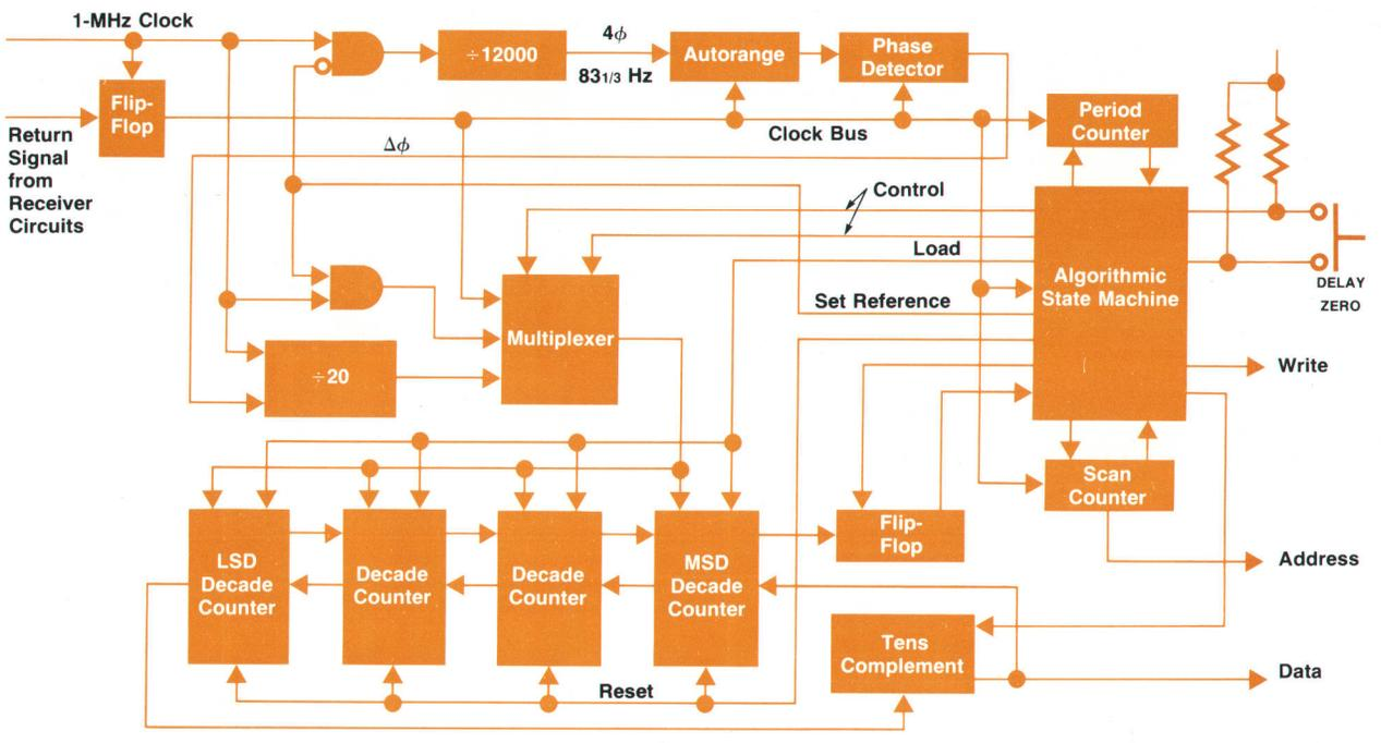
Fig. 3. 4940A envelope delay measurement circuits
