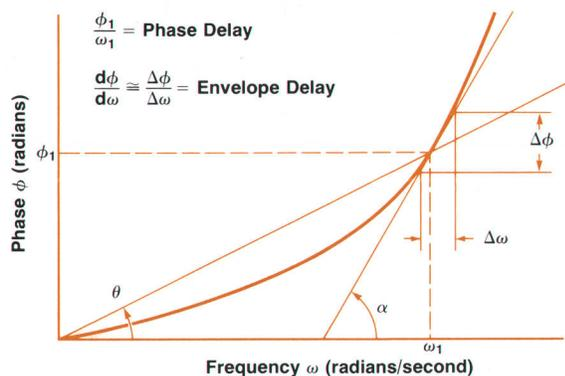
Fig. 1. Phase delay and envelope delay defined.
