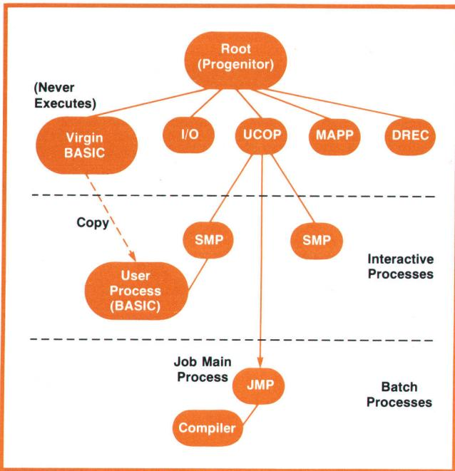
**Fig. 3.** Since BASIC is invoked so often in MPET, it is permanently linked into the operating system. A virgin BASIC process, created when the first user requests BASIC, is simply copied for subsequent requests.
