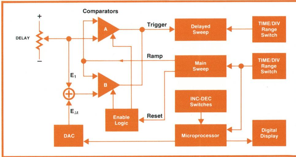
DEC-INC switches (Fig. 5) which, when held to one side or the other, cause  $E_{\Delta t}$  to decrease or increase, moving the right-hand marker to the left or right along the waveform. The microprocessor reads the value of  $E_{\Delta t}$ , converts it to the equivalent time interval scaled according to the time base setting, and displays the result.
