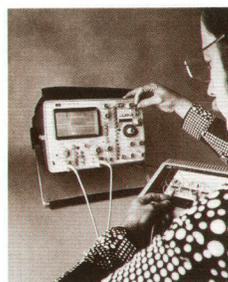
**Cover:** *The LED numeric display on this oscilloscope is an essential part of a new way of measuring very short time intervals, such as the propagation delay of a flip-flop breadboarded here on the HP logic lab. A description of the oscilloscope and the new technique begins on this page; the logic lab was described last month.*
