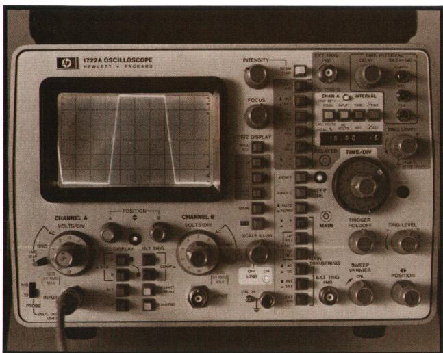
**Fig. 2.** Two markers are positioned to indicate the start and stop regions of a time-interval measurement and the digital readout shows the time interval between the markers. The example here shows the pulse width to be 18.80  $\mu s$ .
