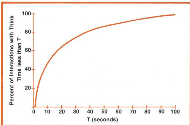
**Fig. 7.** TEPE simulates a random user think time between one second and 100 seconds. The think time distribution is exponential, and the mean value is 23 seconds, which agrees closely with published statistics.
