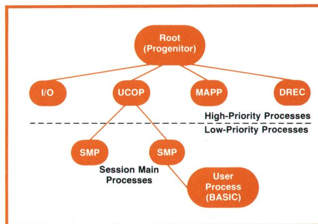
**Fig. 2.** In the original MPE process structure, BASIC is a low-priority process that executes in the general process queue. In MPET, the BASIC user's session main process (SMP) is forced to the head of the queue when it is first created. This improves session-initiation time.
