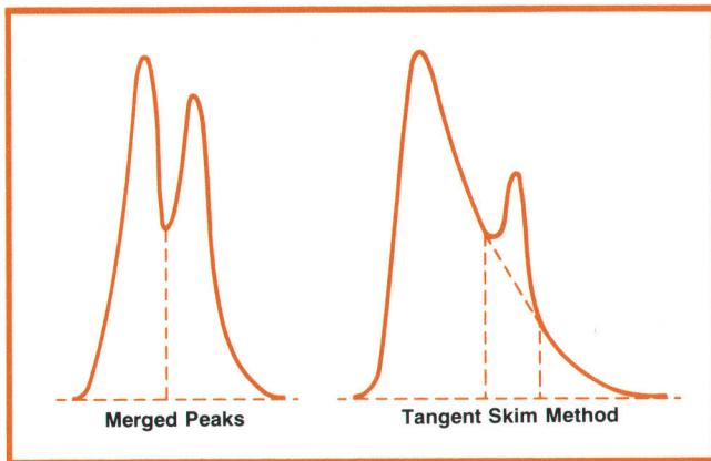
**Fig. 5.** Areas of merged peaks (left) are separated by a line dropped from the valley to the baseline. The area of a small peak riding on a tailing peak (right) is computed using the tangent line as a baseline. The area in the trapezoid below the tangent line is allocated to the tailing peak.
