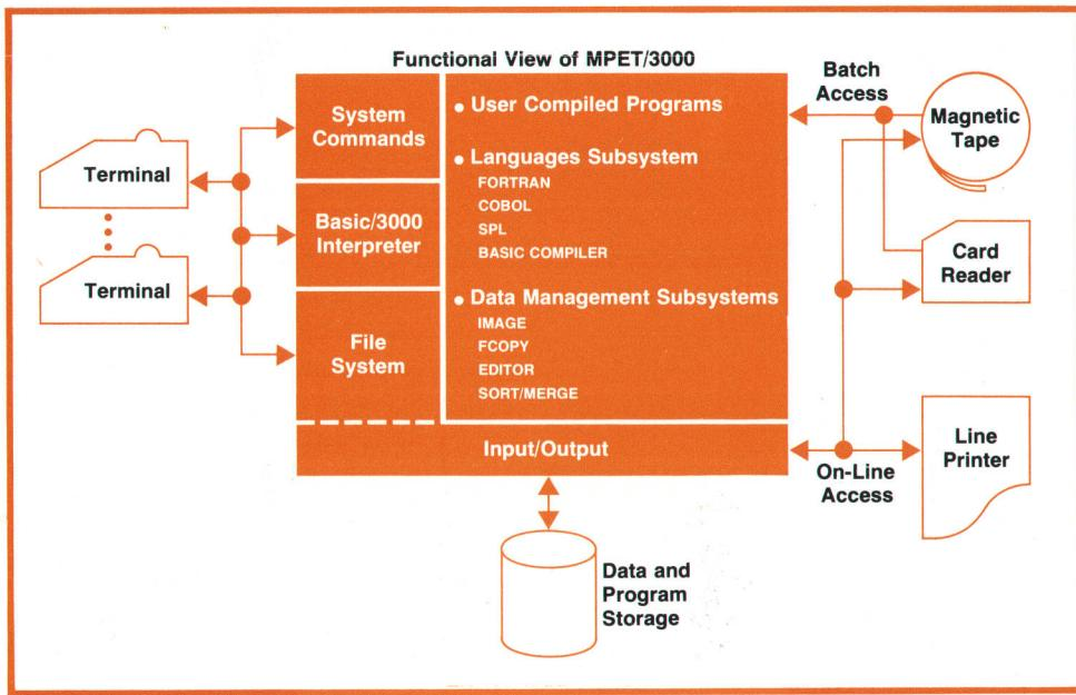
**Fig. 1.** MPET, a modification of the Multiprogramming Executive (MPE) for HP 3000 Computer Systems, optimizes the system for BASIC-language timesharing, yet retains the ability to support concurrent multilingual batch processing.
