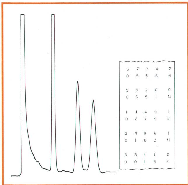
**Fig. 2.** Integrator printout with the corresponding chromatogram. The lower number of each pair gives the retention time in hundredths of minutes. The upper number gives the area count in  $\mu\text{V}\text{-seconds}$  with the digit in the right-hand column representing a power of 10 multiplier, e.g. 3311 2 means  $3311 \times 10^2$ .
