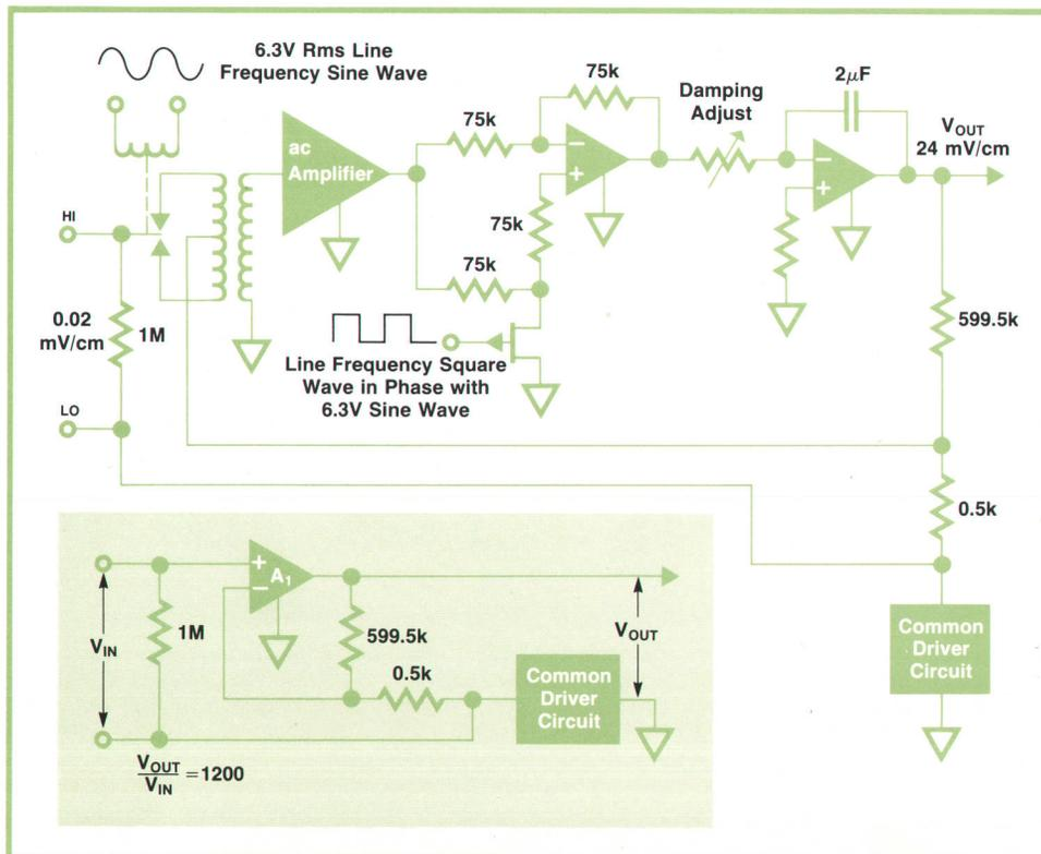
**Fig. 2.** High sensitivity of the 7047A Recorder comes from its chopper stabilized input pre-amplifier. Shown here are a simplified schematic of the preamp and an equivalent circuit (inset) for the most sensitive range. The preamp acts as a dc operational amplifier, A<sub>1</sub>.
