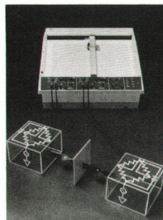
**Cover:** Our artist's representation of a two-bridge measurement that's easy for the 7047A X-Y Recorder, difficult or impossible for others. Stress-versus-strain for an unknown sample is measured by applying equal forces to the unknown and to a sample of known characteristics, using the 7047A to plot one deflection against the other. One arm of each bridge is a strain gauge. The ac generators represent common-mode voltages frequently encountered in such measurements.
