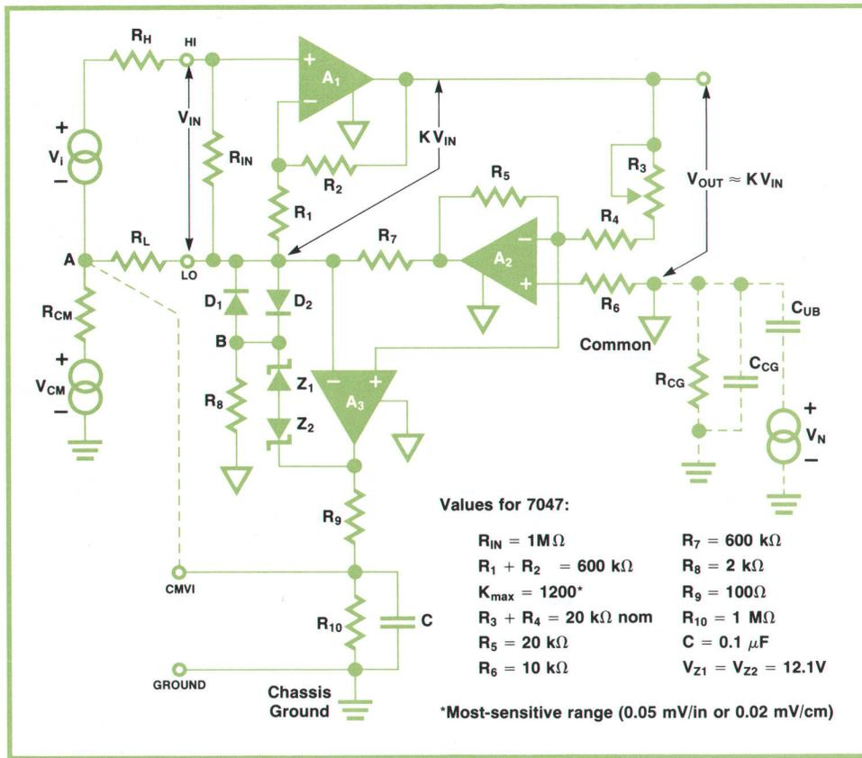
**Fig. 6.** Simplified schematic of the 7047A input circuit.  $A_1$  is the equivalent of the input preamplifier and  $A_3$  is the common driver amplifier. The COMMON MODE VOLTAGE INPUT (CMVI) does not have to be connected unless the common-mode voltage exceeds  $\pm 10\text{ V}$ .
