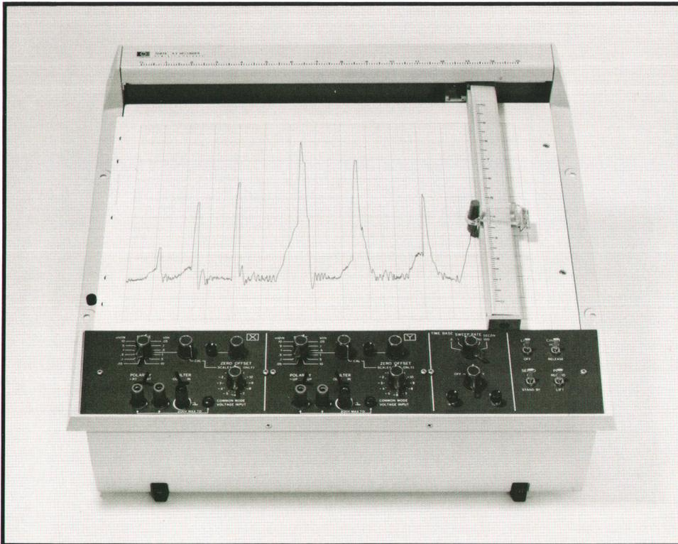
**Fig. 1.** Model 7047A X-Y Recorder has maximum input sensitivity of 0.02 mV/cm (or 0.05 mV/in with English scaling) on both axes. Common-mode rejection is greater than 130 dB with 1-k $\Omega$  impedance in series with either input terminal (or both). Six sweep speeds, calibrated zero offset, polarity switches, and input filters are standard features.
