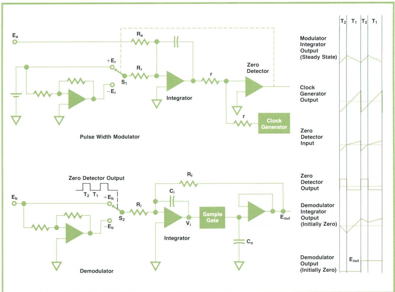
**Fig. 7.** Multiplier consists of a pulse width modulator and a demodulator. One multiplier input varies the duty cycle of the modulator output pulse, and the other varies the demodulator gain. Multiplier linearity is better than 0.2% for both inputs.
