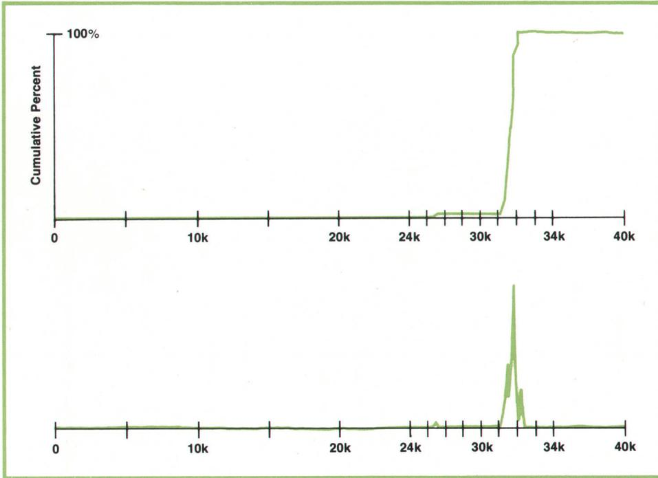
**Fig. 6.** Activity profile generated by ACP. The horizontal axis shows memory locations 0 to 40000<sub>8</sub> (16384<sub>10</sub>). The subroutines located between 31200<sub>8</sub> and 32200<sub>8</sub>, approximately, are the only ones that influence the execution time of this user's benchmark program. The little bump at 25400<sub>8</sub> is the benchmark program itself.
