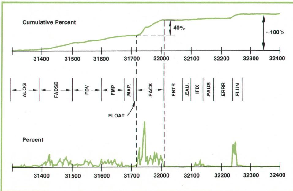
**Fig. 7.** An expanded view of the area around 32000<sub>8</sub> in Fig. 6. Resolution is two words, compared to 100 words in Fig. 6. Notice how the areas with system performance leverage stand out. The .PACK subroutine takes about 40% of the time, but the .MAP. subroutine, which resolves subscripts, has essentially zero leverage for this benchmark.
