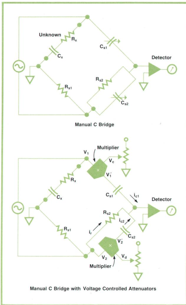
**Fig. 2.** A capacitance bridge may be balanced by adjusting standard capacitors, as shown in (a), or by adjusting the gain of a voltage-controlled attenuator, or multiplier, as shown in (b). Model 4282A uses the latter approach, adding a feedback loop so balance is achieved automatically.
