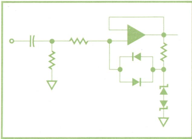
**Fig. 6.** For high voltage protection, zener diodes are connected to each input voltage follower. Circuit is designed so that, in normal operation, no ac voltage appears across the diodes, so they introduce no distortion or additional stray capacitance.
