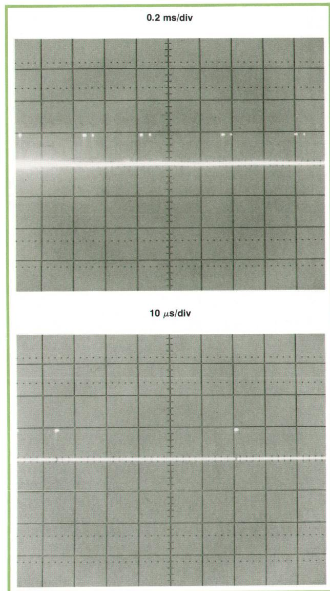
**Fig. 3.** Setting a subroutine's entry address into the switches of a breakpoint register makes it possible to see how often that subroutine is used and what its execution time is. Top photo shows this subroutine is invoked about every 0.5 millisecond. Bottom photo shows subroutine is about 70 microseconds long; pulses are entry, parameter pickup, and exit.
