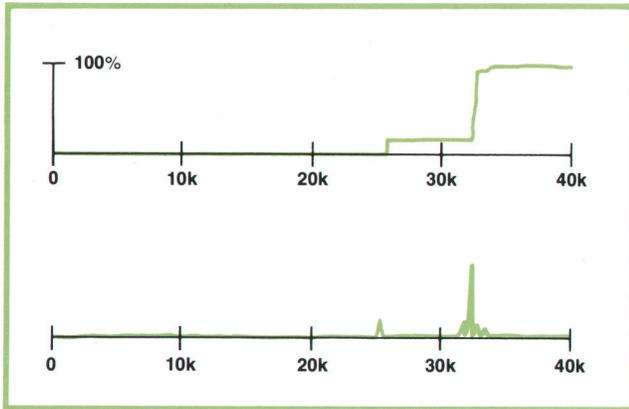
**Fig. 8.** Activity profile for the benchmark of Figs. 6 and 7 with floating-point firmware replacing the FADSB, FMP, FLOAT, FIX, and .FLUN routines and eliminating .PACK entirely. The benchmark runs six times faster, an improvement that could have been predicted from Fig. 7. Subroutine ALOG now takes 70% of the time, most of it in a 28-word section, .MAP. takes about 10% of the time, and the user's program about 20%. Thus there is still room for improvement.
