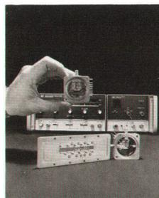
**Cover:** *In the background is the new Model 86290A 2-to-18-GHz RF Plug-in installed in an 8620A Sweep Oscillator mainframe. In the foreground are the three components whose development made the broadband RF plug-in possible: a YIG-tuned oscillator (top), a power amplifier (left), and a YIG-tuned multiplier (right).*
