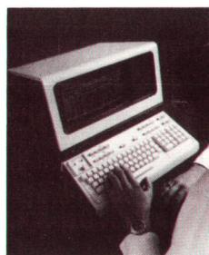
**Cover:** Model 2640A Interactive display terminal uses its optional line-drawing character set to display a form to be filled in by the operator. Microprocessor control gives this new terminal a high degree of flexibility at a relatively low cost.
