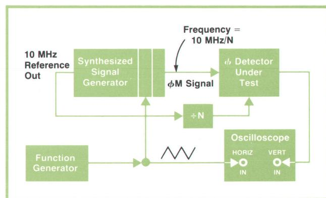
Fig. 4. Set-up for measuring phase detector characteristics.
