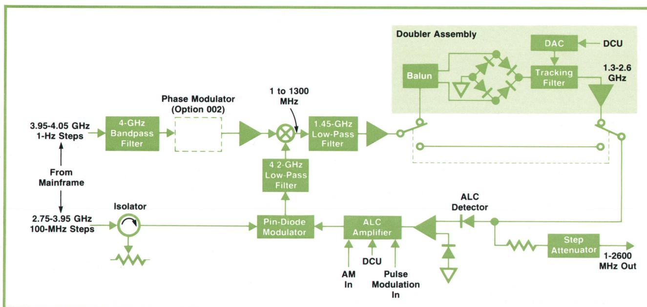
**Fig. 2.** Block diagram of the Model 86603A 2.6-GHz RF Section. Microwave signals supplied by the mainframe give difference frequencies over a range of 1-1300 MHz in 1-Hz steps. The frequency doubler extends the output range to 2600 MHz.
