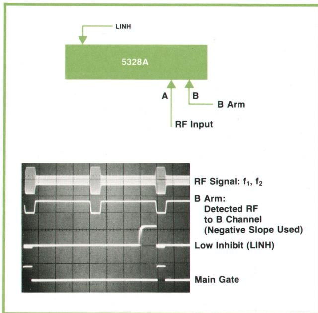
**Fig. 4.** The counter can be armed by two inputs simultaneously to make more complex measurements. Here the arming channel is channel B, but the LINH input must be high when channel B is triggered for arming to occur.
