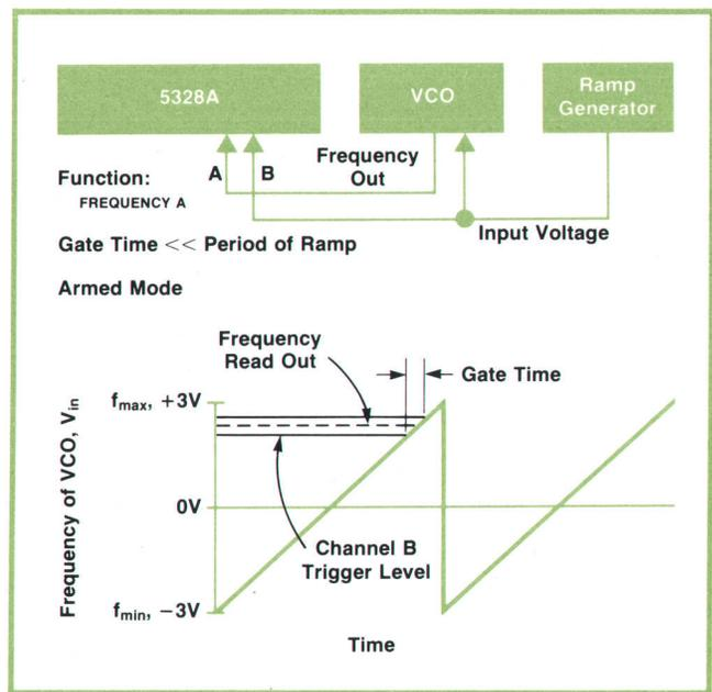
Fig. 3. In the armed mode the counter can be used to check the output frequency of a voltage-controlled oscillator as a function of its input voltage.
