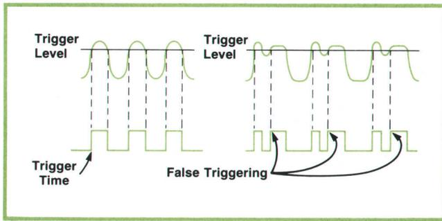
**Fig. 1.** Marker outputs show when the input amplifiers are triggering. Trigger levels can be monitored with an oscilloscope by displaying the input signal and the marker. Markers can also show false triggering, and can be used to synchronize other instruments.
