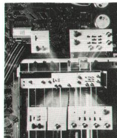
**Cover:** Model 5328A Universal Counter and its optional input modules are superimposed on a background photograph showing the counter's interior and the bus-oriented architecture that makes its high degree of modularity possible. Input
