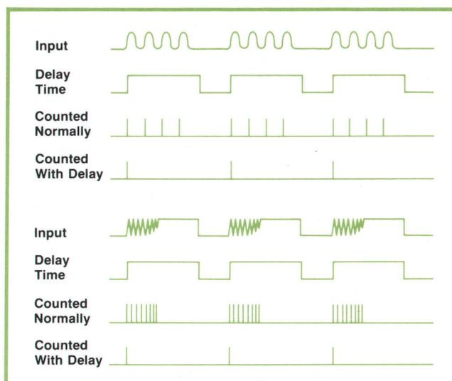
**Fig. 5.** High-performance universal module has a variable delay feature. In time interval measurements, delay causes the counter to ignore stop events until the delay times out. Delay can also be used in frequency, period, ratio, and totalize measurements to inhibit triggering on unwanted triggerable events.
