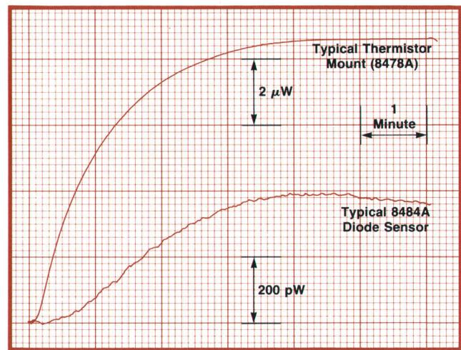
**Fig. 3.** Drift of a typical 8484A High-Sensitivity Power Sensor in response to a hand grasp, compared with that of a typical thermistor power sensor. Both sensors were on their most sensitive ranges, which differ by  $10^4$  in sensitivity.
