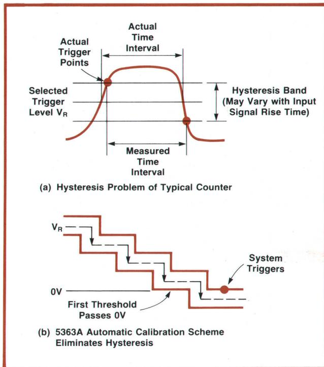
**Fig. 2.** (a) Because of hysteresis, the actual trigger point of a counter is offset from the selected level by an unknown amount, often 50 mV or so. (b) Model 5363A Time Interval Probes automatically calibrate themselves; they detect the actual reference voltage at which a grounded probe triggers, then add this offset to the reference voltage in subsequent measurements. Actual trigger level is then within a few millivolts of the selected level.
