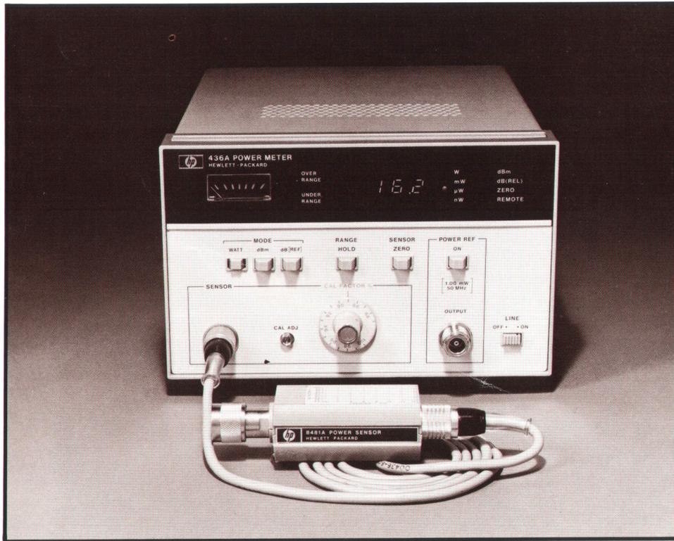
**Fig. 1.** Model 436A Digital Power Meter with Model 8481A Power Sensor measures power from  $3\mu\text{W}$  to 200 mW at frequencies from 10 MHz to 18 GHz. Five other sensors extend the frequency and power ranges.
