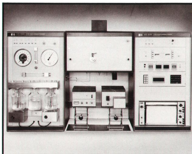
**Fig. 3.** The Model 1010B Liquid Chromatograph. The solvents are in the glass containers on the left; the pumps are inside this cabinet. The column is inside the center cabinet with the injection port protruding from the panel. The detectors are on the shelf below. The flow controller is in the cabinet at right.
