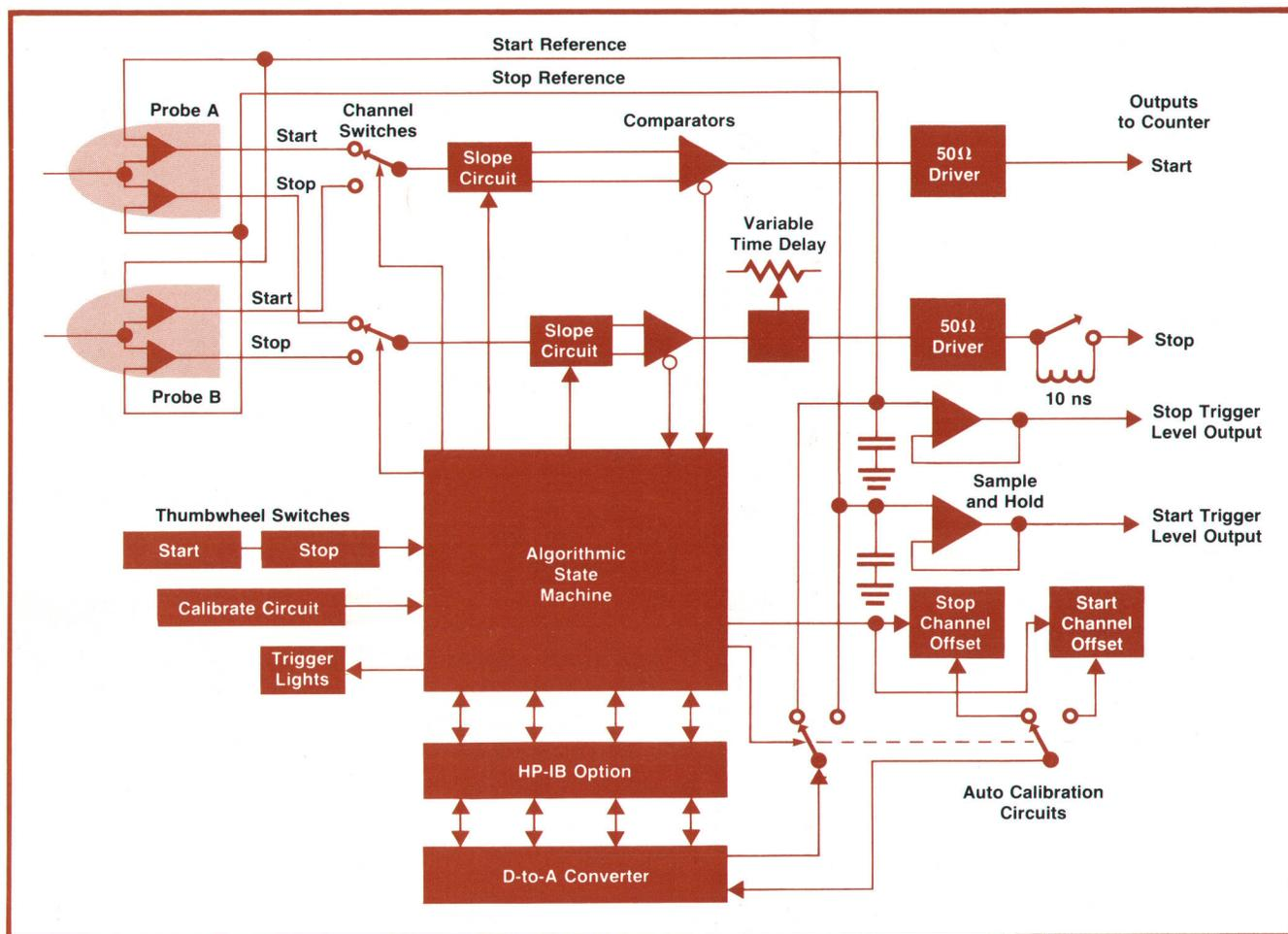
**Fig. 3.** Each probe has a potential start and stop input. Red and green trigger lights above each probe indicate which probe has been selected for stop and start, respectively, and flash off when triggering occurs. A state machine controls system operation.
