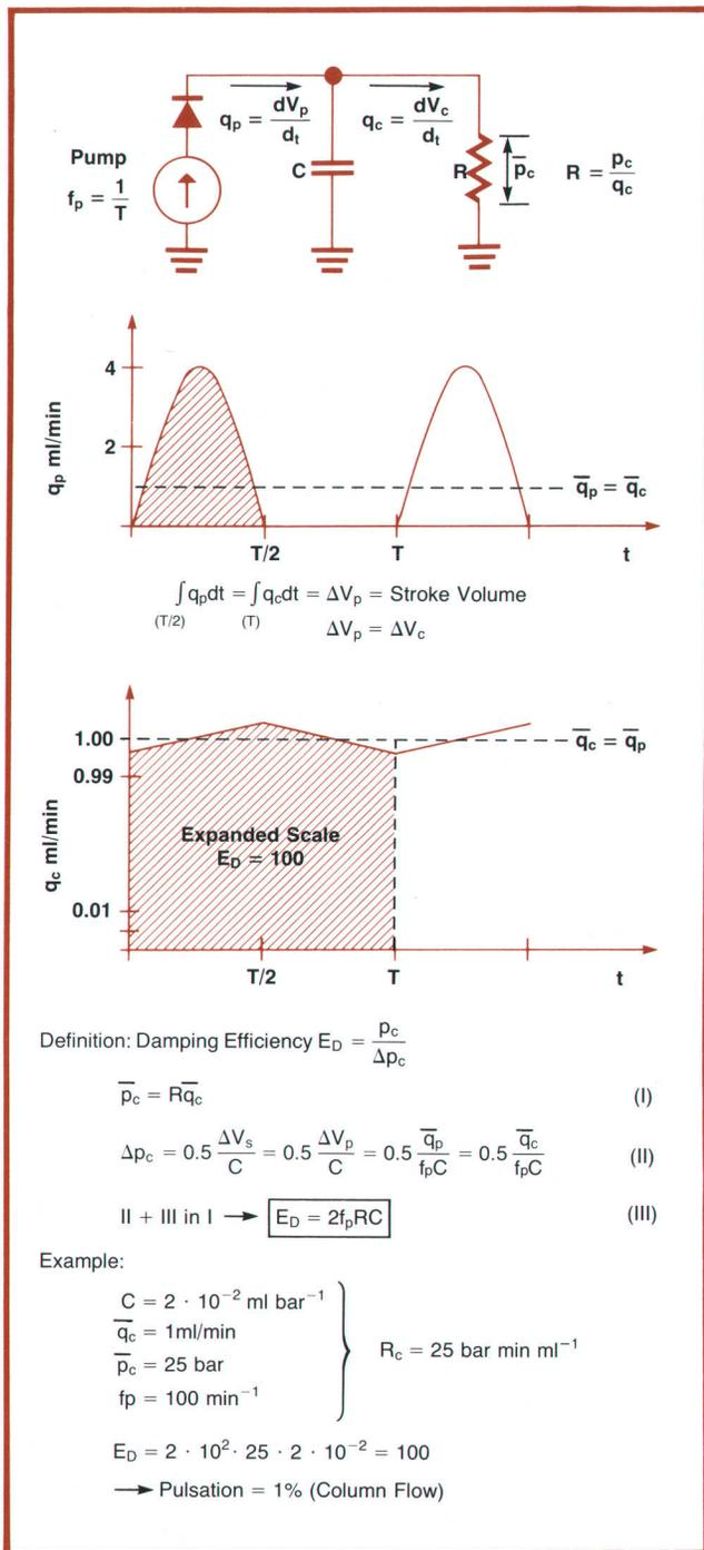
**Fig. 5.** Hydraulic capacitor (C) and a flow restriction (R) are the analog of an RC filter. The diode is the analog of the pump's check valve. As the equations show, adequate smoothing can be obtained with a relatively low value of R provided C is large enough.
