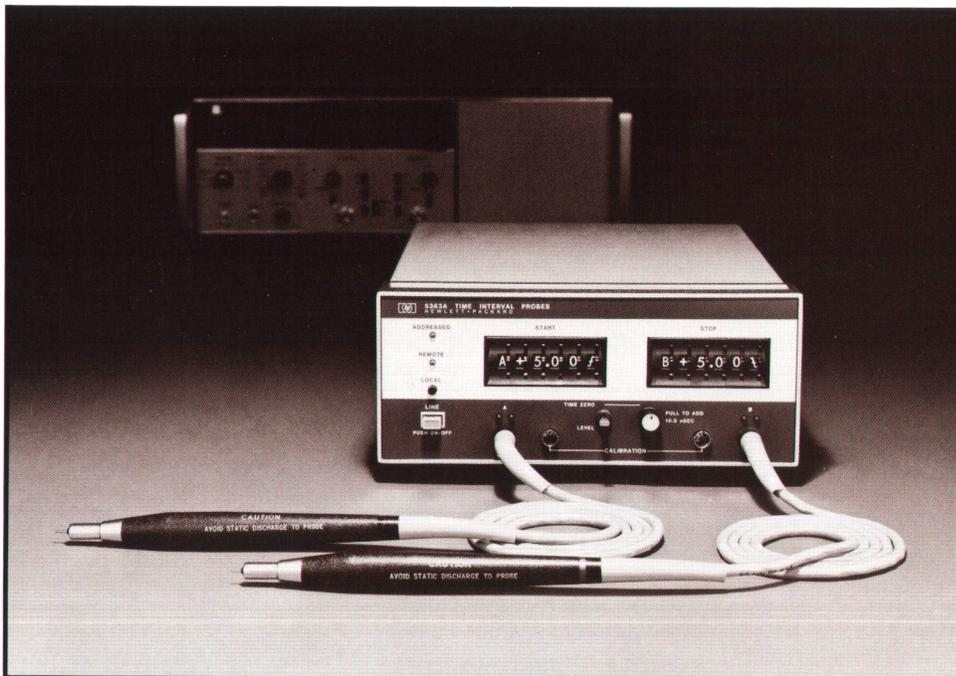
**Fig. 1.** Model 5363A Time Interval Probes consist of two low-capacitance (10 pF) active probes and associated electronics in a separate box. Either probe can be used alone to make start/stop measurements or both probes can be used, one for start and one for stop. Trigger levels are adjustable from  $-9.99$  V to  $+9.99$  V. An adjustable delay equalizes propagation time differences in start and stop channels.
