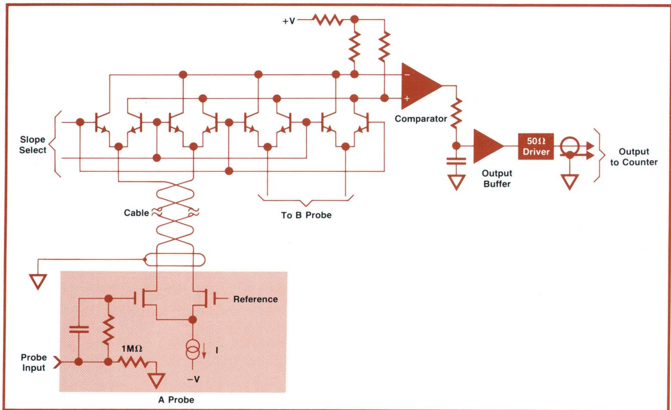
**Fig. 4.** Start or stop channel is basically a voltage comparator. The input circuit presents a standard comparator with a signal that has a single transition direction and a small dynamic range centered in the comparator's window.
