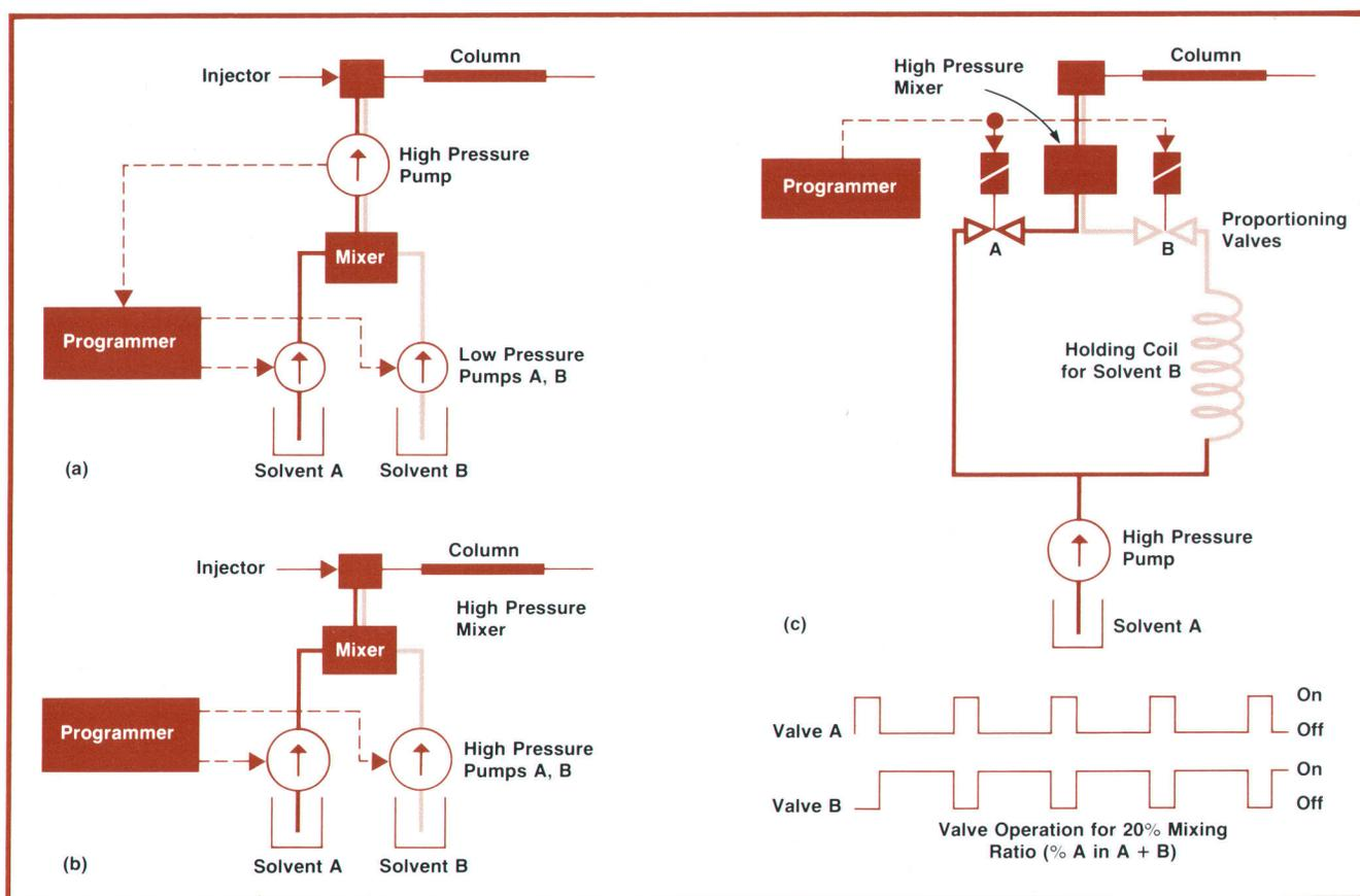
**Fig. 1.** Three types of gradient elution systems. The type shown in (a) uses two low-pressure pumps to control the flow of solvents to the high-pressure pump. That in (b) has two high-pressure pumps to control solvent flow. The one in (c) uses a single pump with a holding-coil bypass and proportioning valves.
