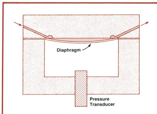
**Fig. 4.** Hydraulic capacitor consists of a rigid vessel filled with a compressible fluid. The capacitance  $C$  is equal to the ratio of the change volume  $V$  to a change in pressure  $p$  or,  $C = dV/dp$ . Since  $dV = V dp/\kappa$ ,  $dV/dp = V/\kappa = C$ .
