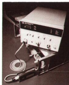
**Cover:** A mini-system that shows off the features and capabilities of the new Model 436A Digital Power Meter and the new Model 8484A Power Sensor (foreground). A Hewlett-Packard Interface Bus option puts the 436A under calculator control. The sensor allows accurate power measurements down to -70 dBm.
