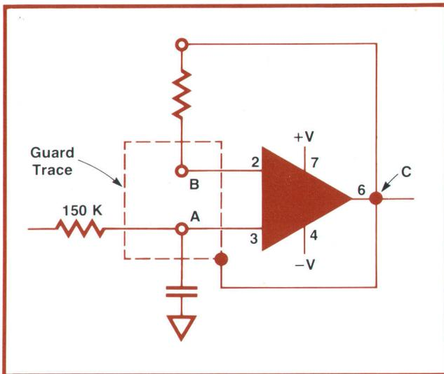
**Fig. 6.** Guarded amplifier inputs reduce leakage problems with wet printed circuit boards, making it possible for the 436A to work in 95% relative humidity and under severe conditions of condensation.
