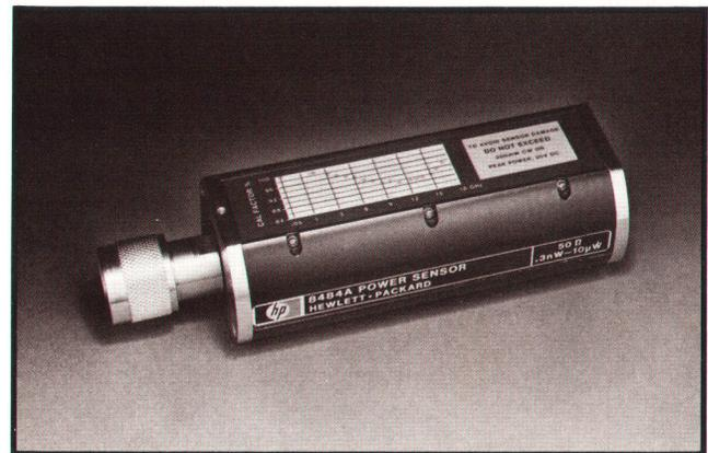
**Fig. 1.** Model 8484A Power Sensor works with HP 435A and 436A Power Meters to measure power from  $-70$  to  $-20$  dBm over a frequency range of 10 MHz to 18 GHz. Calibration factor is shown on housing as a function of frequency.
