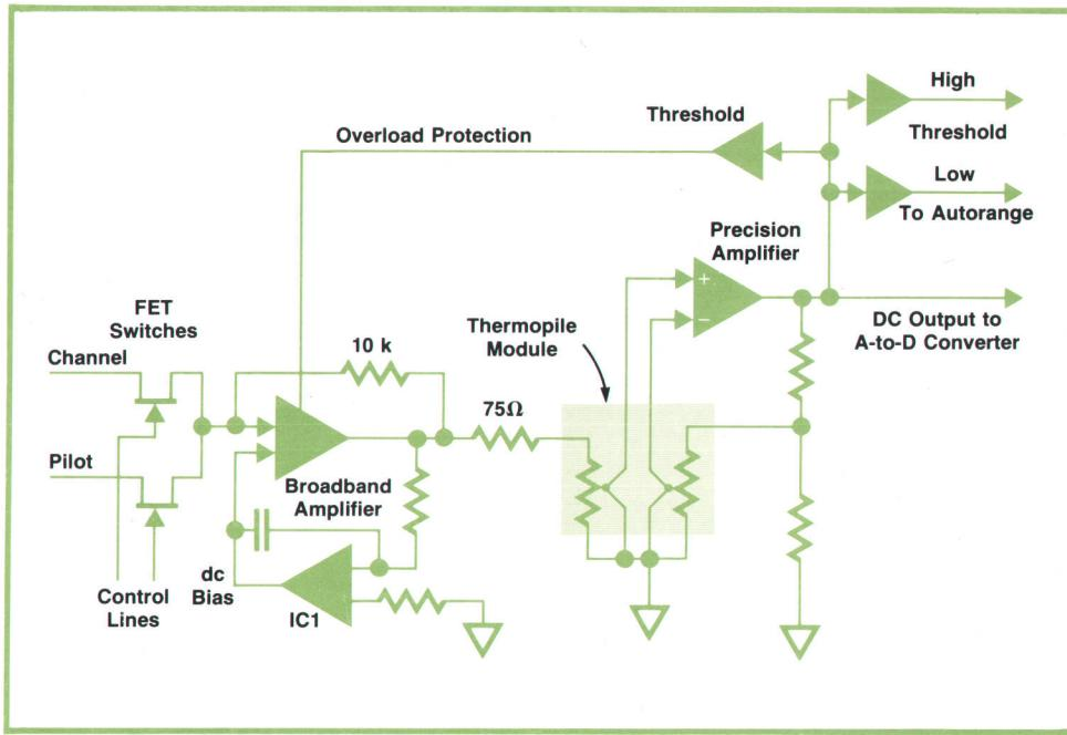
**Fig. 5.** Power level detector matches a precise fraction of its dc output to the rms value of the input signal in this feedback arrangement. To preserve the excellent linearity of the thermopile (<0.01 dB error over a 10-dB range), a precision IC operational amplifier that minimizes offsets and thermal drift is used.
