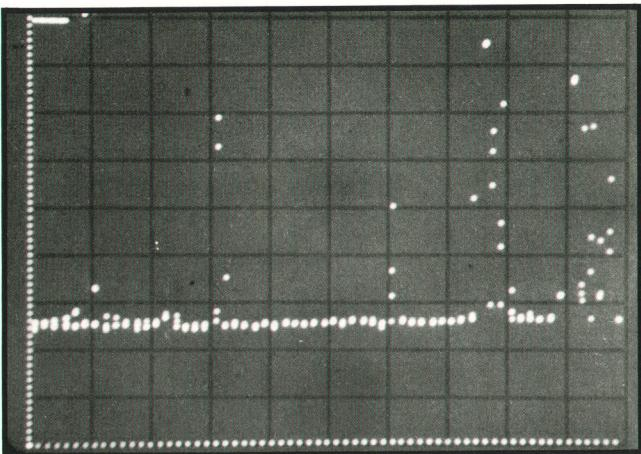
**Fig. 4.** This display on the optional CRT monitor shows signal levels in the 60 channels of a supergroup. Most channels are not in use and lie at the idle noise level (the short horizontal line at left is the reference level at -20 dBm). Channels with several dots in a vertical line are speech channels while the three bright dots at top are data channels. The vertical scale is 10 dB/div.
