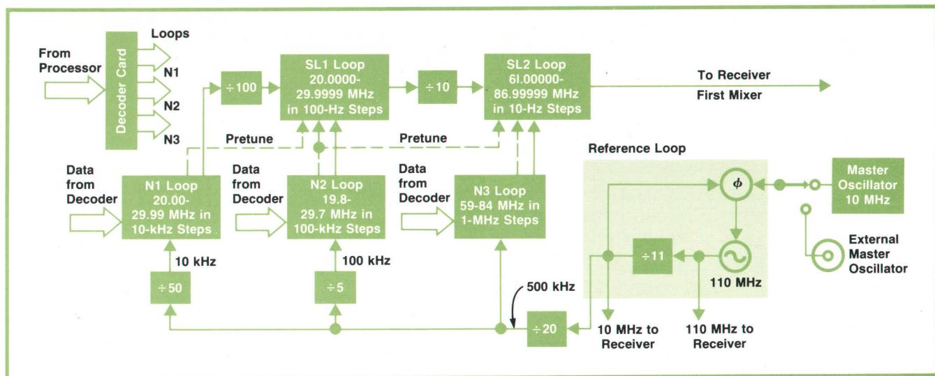
**Fig. 1.** Block diagram of the synthesizer used for generating local oscillator frequencies in the Model 3745A Selective Level Measuring Set. It is tuned by digit-serial data sent from the instrument's processor and stored in shift registers on the decoder board.
