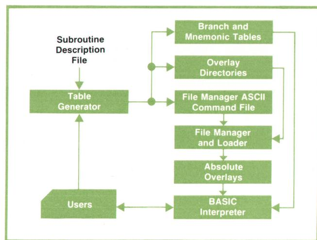
**Fig. 4.** The process of producing overlays and branch and mnemonic tables is completely independent of the BASIC interpreter. Thus a user can configure his own set of subroutine tables without interfering with other terminals using BASIC.
