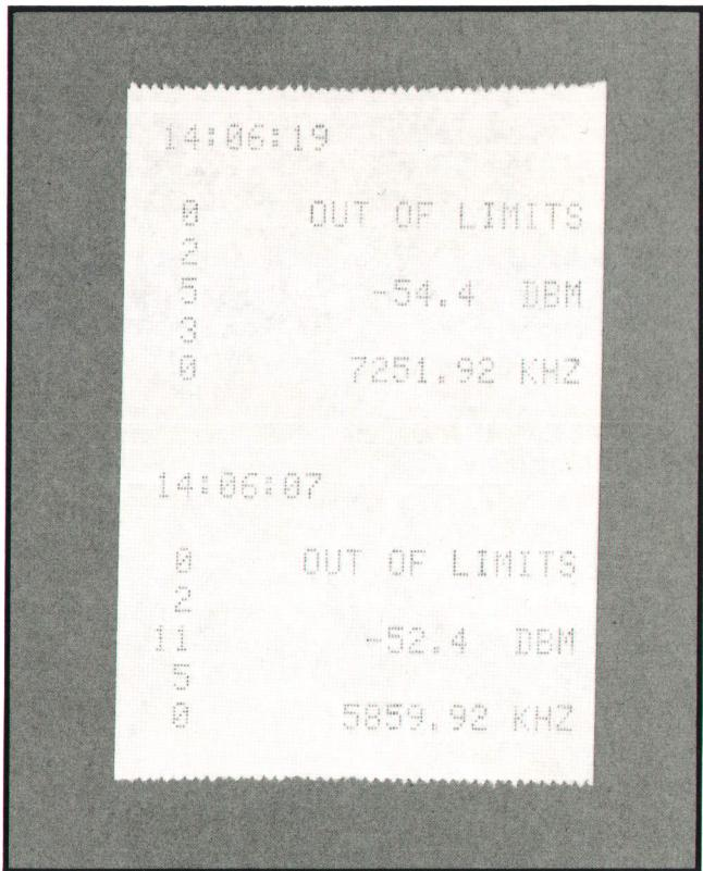
**Fig. 3.** Typical printout from the optional digital printer lists the time of day and the FDM description of the measured channel (vertical column of numbers).
