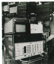
**Cover:** *Picking one particular channel out of a babble of thousands of frequency-multiplexed communications channels is greatly simplified by a new selective level measuring set that talks the language of the telephone engineer. Microprocessor control is the key to this new ability, as described in the series of articles beginning on this page. Our thanks to Farion Electric for the loan of their facilities for this photo.*
