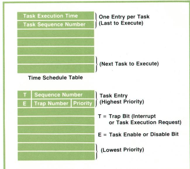
**Fig. 5.** The BASIC scheduler allows program execution to be controlled by the time of day or by external events. This is what makes the new BASIC a real-time system. Scheduling of tasks requires three tables: the trap table, the time schedule table, and a priority stack. These tables are interrogated before execution of each BASIC program statement.
