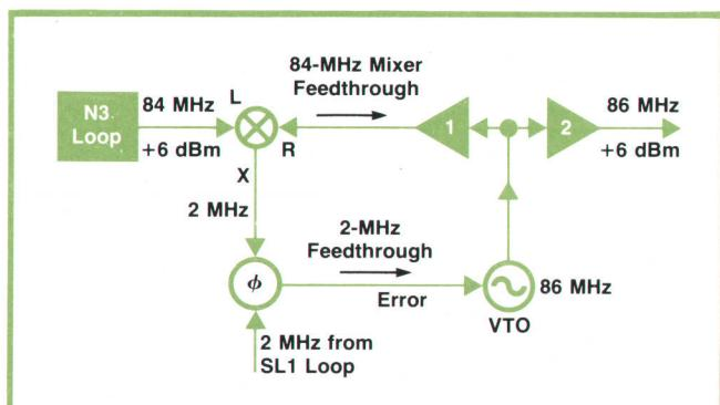
**Fig. 3.** Spurious outputs can be generated at the SL2 output by direct feedthrough of the N3 frequency by way of the mixer and by modulation of the VTO by feedthrough of the phase-detector switching frequency.
