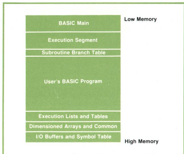
**Fig. 2.** The real-time BASIC interpreter consists of nine modules: a main module and eight segments. Each user program has its own copy of the main module and the execution segment, arranged in memory as shown here. The interpreter is arranged this way to provide maximum efficiency in memory use and minimum time spent in disc accesses.
