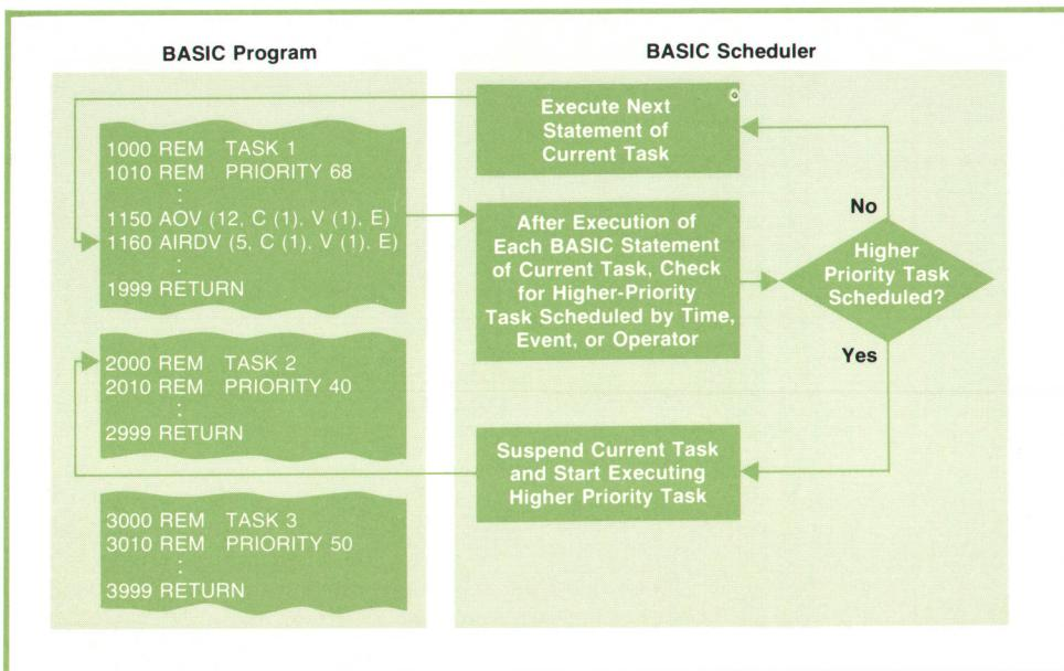
**Fig. 6.** Operation of the real-time BASIC scheduler as a typical program executes. After execution of each program statement, the scheduler checks for time and event interrupts. It examines task timing and priorities and either continues running the current task or begins a newly scheduled task having higher priority.
