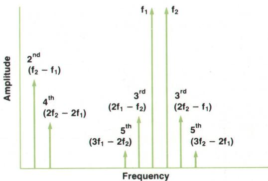
The drawing shows a typical situation involving two signals,  $f_1$  and  $f_2$ , processed by a nonlinear device. The intermodulation products include frequencies that lie close to the signals, the third-order terms ( $2f_1-f_2$ ,  $2f_2-f_1$ ) being particularly troublesome. Products higher than fifth order are usually negligible.
