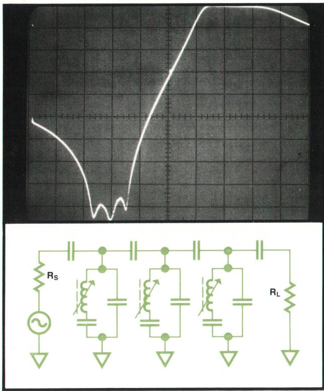
**Fig. 3.** Configuration of a typical IF bandpass filter used in the new SLMS. The filter has stopband notches below the passband that suppress image frequencies and IF feedthrough. The CRT display shows the frequency response of the 101.75-kHz bandpass filter which has staggered notches to broaden the stopband (vertical scale: 10 dB/div; horizontal scale: 1 kHz/div).
