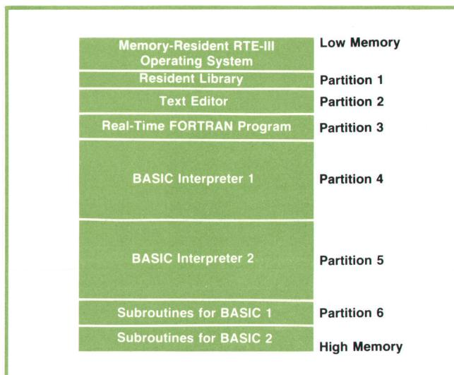
**Fig. 3.** Real-time BASIC is an option to the HP real-time executive systems, RTE-II and RTE-III. RTE-III can maintain several copies of the BASIC interpreter in separate partitions of memory. This is a simplified RTE-III memory map with two BASIC interpreters simultaneously resident in memory.
