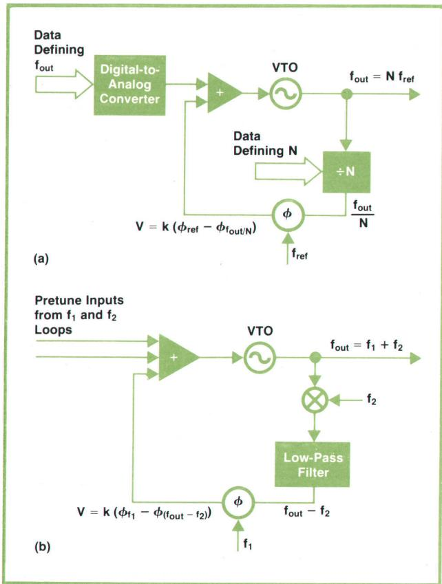
**Fig. 2.** Divider loops (a) use digital dividers to obtain a submultiple of the output frequency. The result of comparing this to the reference frequency controls the voltage-tuned oscillator (VTO), giving an output frequency that is an exact multiple of the reference frequency. Summing loops (b) use a VTO controlled by a phase comparator to derive a frequency that is the sum of a divider loop output and a decade submultiple of the previous frequency (see Fig. 1).
