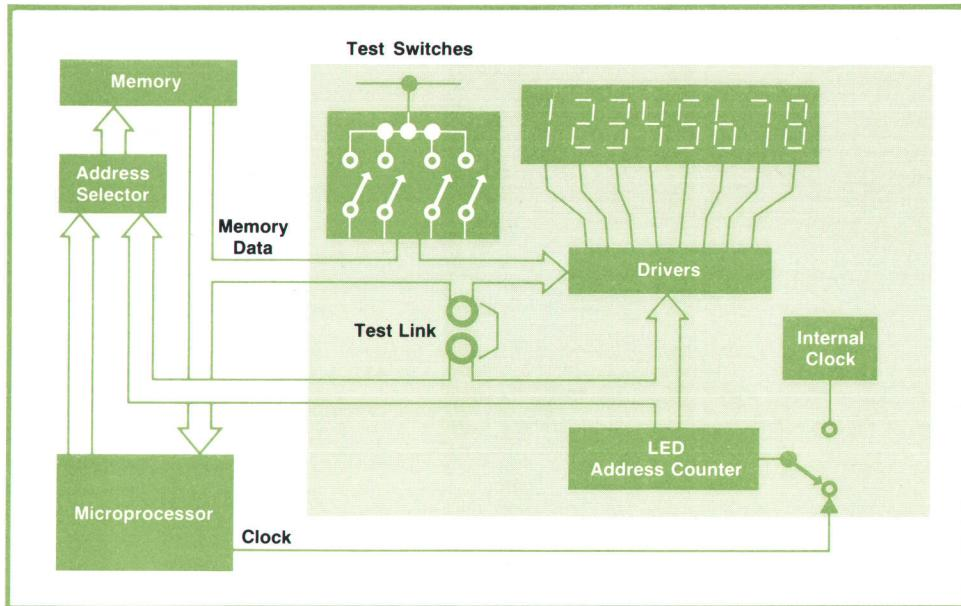
**Fig. 2.** Direct memory access allows display of measurement information during times that the microprocessor is not using memory. When the display is unplugged from the processor, it can operate from its own internal clock with data placed on the input lines by the test switches or by a link to the address lines.
