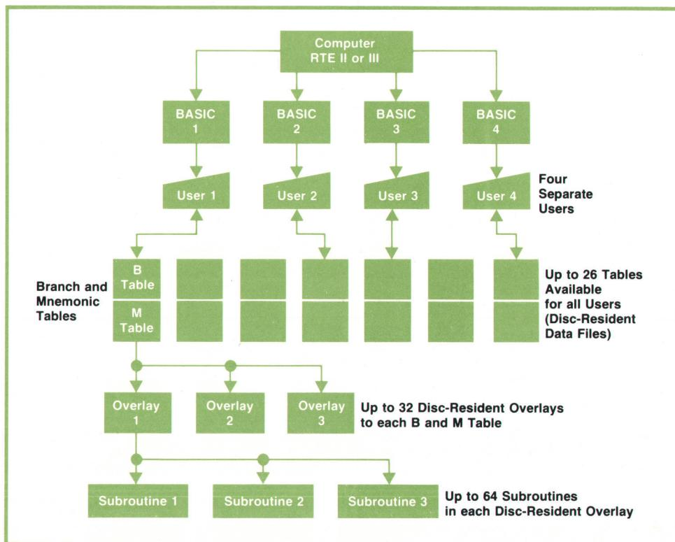
**Fig. 1.** Real-time BASIC supports up to four independent terminals. Any user can attach subroutines and functions to BASIC to be used on his terminal. The system may have up to 26 sets of subroutines and functions. Each set is identified by a branch table and a mnemonic table and may consist of as many as 32 overlays, each containing up to 64 subroutines and functions.
