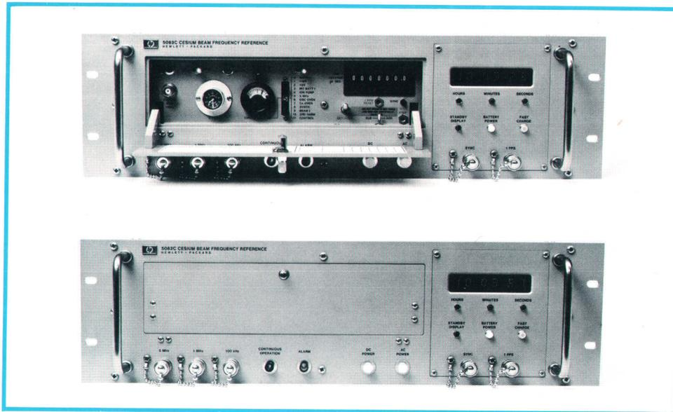
**Fig. 1.** Model 5062C Cesium Beam Frequency Reference is designed for navigation, communications, and guidance systems, and other applications requiring laboratory-standard accuracy in a rugged, compact instrument. Specified accuracy is  $\pm 3 \times 10^{-11}$  over a temperature range of  $-28^\circ$  to  $+65^\circ\text{C}$ . Weight is 32 kg with optional standby battery.
