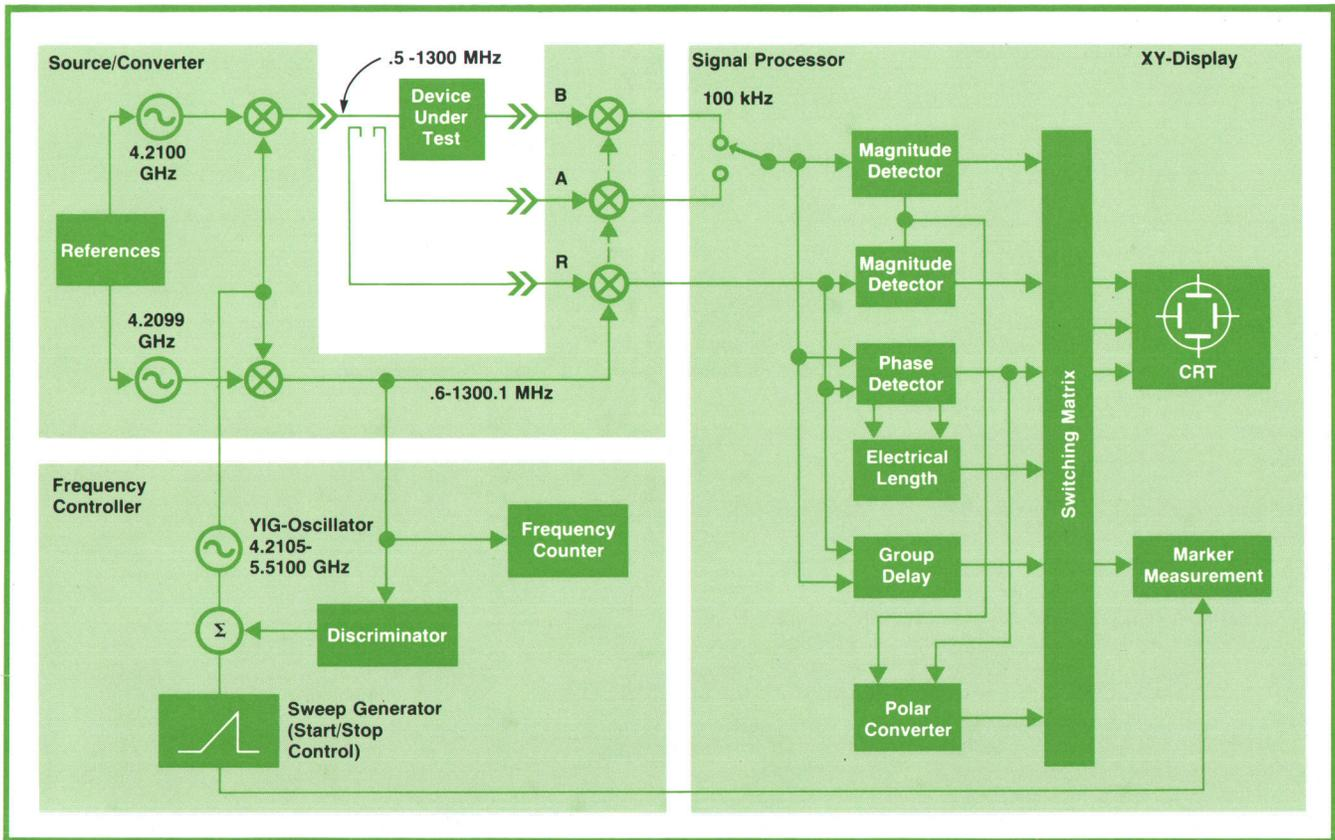
Fig. 7. Organization of the Model 8505A Network Analyzer.
