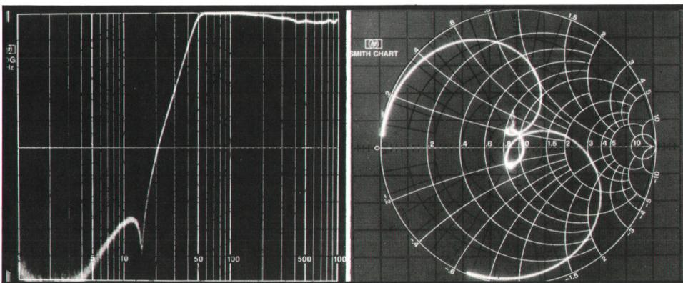
**Fig. 2.** Swept-frequency measurements may be displayed in either cartesian or polar coordinates. Transparent Smith-chart overlays, as shown in the photo of a filter input impedance at right, are provided for direct readout of impedance with the polar displays. Overlays with logarithmic scales are also provided for logarithmic sweeps, as in the photo at left showing the response of a 65-MHz high-pass filter over a 100-dB dynamic range, swept from 1 to 1000 MHz.
