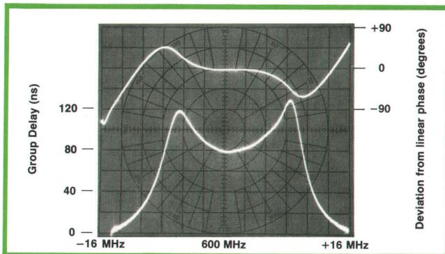
**Fig. 4.** Dual trace display shows swept measurement of group delay (lower trace) and deviation from linear phase shift (upper trace). Group delay is defined as the negative rate of change of the phase deviation curve.
