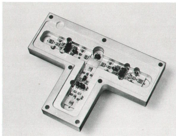
The 100-kHz tank circuit in the IF output improves the signal-to-noise ratio but its impedance in the RF range is higher than wanted. The solution to this problem was to use an IF input amplifier that has an input impedance of less than 3 ohms. The IF input amplifier is not part of the microcircuit but it is mounted close to the down converter for minimum line length. It is followed by a 300-kHz low-pass filter for further attenuation of the LO and RF signals.
