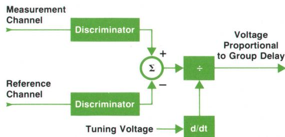
The block diagram for the circuits performing the group delay measurement is shown above. The two discriminators obtain voltages proportional to the frequencies at the input and output of the device, and a voltage proportional to the frequency difference  $\Delta\omega$  is obtained by subtracting one from the other. The tuning ramp from the frequency sweep control is differentiated to obtain  $\alpha$ , the rate of change of frequency, and used to divide  $\Delta\omega$  to obtain  $t_D$ .
