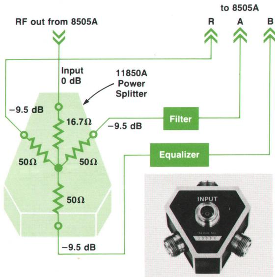
a three-way power splitter is an important tool. The Model 11850A/B Power Splitter was designed to match signal tracking between any two ports within 0.1 dB in magnitude and 1.5° in phase. It is available in both 50Ω and 75Ω versions.
