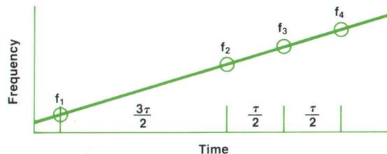
quency increases linearly during the counter gate, however, so the total count is higher than wanted. The counter pauses, then counts down on the RF for another gate time ( $f_3$  to  $f_4$ ).
