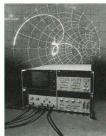
**Cover:** The subject of this month's issue, Model 8505A Network Analyzer presents swept-frequency measurements in either Cartesian or polar coordinates on its CRT display and its digital displays give the frequency, magnitude, phase, and delay of any point selected on the CRT trace by a movable marker.
