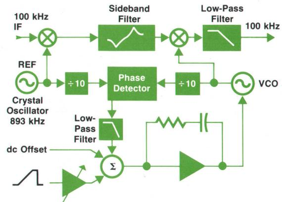
The phase detector is a conventional 0-360° detector. To extend the offset range, the oscillator outputs are divided by a factor of 10 before the phase comparison, allowing the VCO to be offset almost as much as 3600° from the reference. By suitable choice of a voltage level to place the zero offset condition at the center of the phase detector's range, the offset operates over a range of  $\pm 1700^\circ$ .
