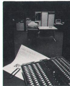
**Cover:** Against a backdrop photo of an HP 3000 Series II Computer System are a Series II memory board and an example of an Error Correcting Memory Log Analysis. The Series II memory corrects all single-bit memory errors so they don't affect
