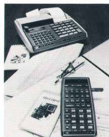
**Cover:** The HP-97 and the HP-67 are fully programmable portable calculators that can run each other's programs. The HP-97 has a built-in thermal printer. The HP-67 and HP-97 are described in the article on page 2. The printer and the HP-91 Calculator that was the first to use it are described in the article on page 9.
