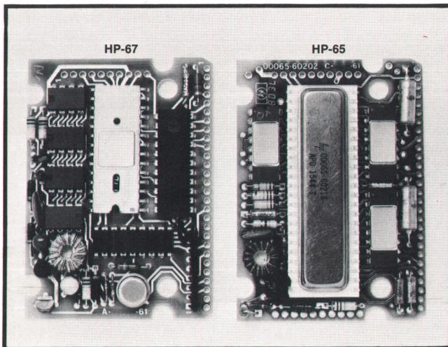
**Fig. 5.** A new combined ROM and data-storage chip makes it possible to put all the HP-67 logic in discrete packages on a conventional two-sided printed circuit board. Here the HP-67 logic board is compared with the HP-65 logic board.
