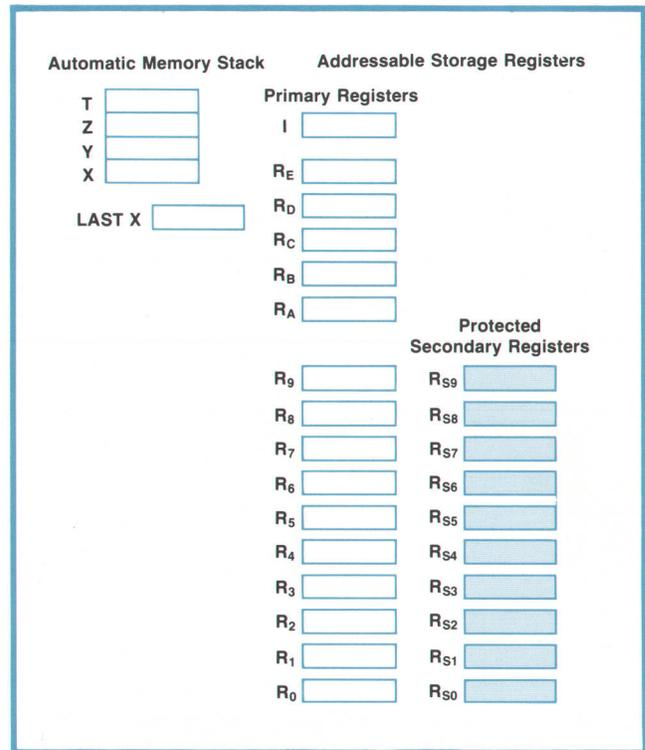
**Fig. 4.** The HP-67 and HP-97 have a four-register operational stack and a register that retains the last number in the X-register, which is the display register. There are 26 addressable data storage registers, including the I-register, that can be used for indirect control. Protected secondary registers cannot be accessed directly with STO and RCL keys. These registers are used most often for statistical functions and programming, but they can be accessed from the keyboard using the P=S key.
