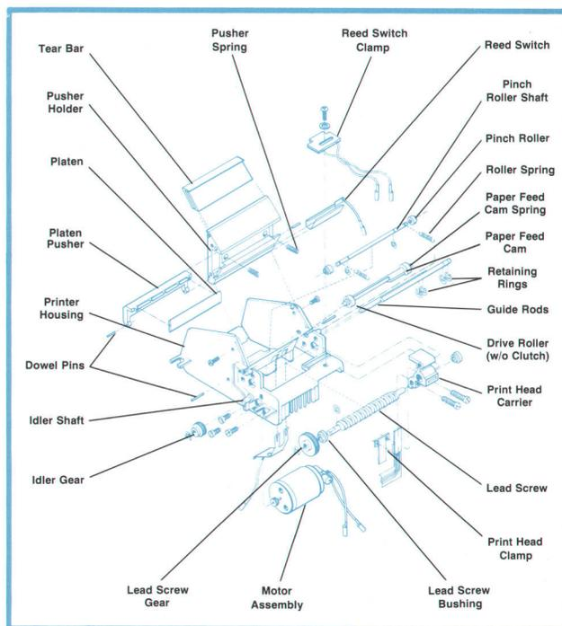
Fig. 9. Printer mechanism.
