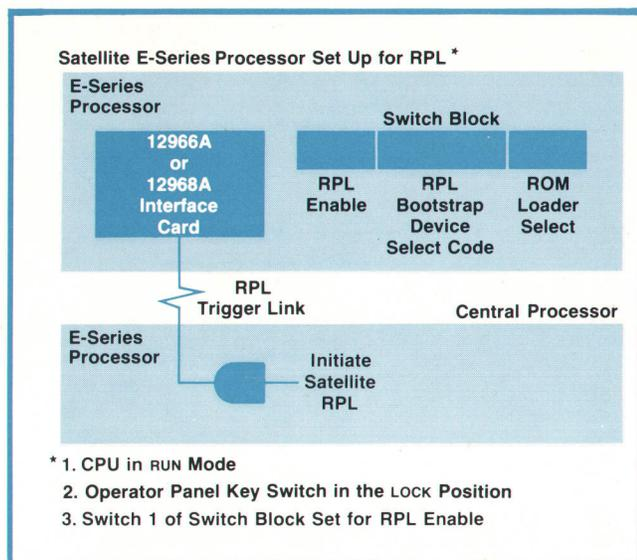
**Fig. 2.** Remote program load is a feature of the E-Series base set microcode that makes it possible to initiate an automatic bootstrap and run operation from a local or remote site. Here a distributed-system central station triggers a satellite E-Series processor.
