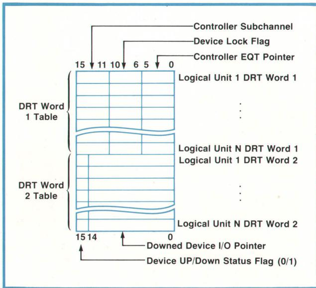
**Fig. 5.** To improve the management of I/O device errors, the device reference table (DRT) was doubled in size. Each I/O device has associated with it one or more logical units, each of which has a DRT entry. The new DRT word 2 for each entry contains a device up/down status flag and a pointer. Formerly, device status flags were in the equipment table (EQT) of the corresponding I/O controller.
