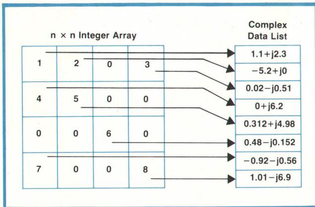
**Fig. 2.** OPNODE uses a sparse Y matrix algorithm, in which the zeros in the Y (admittance) matrix are not stored as data. The technique is efficient and fast. A 40-node ladder network is solved at a rate of about one frequency per second.
