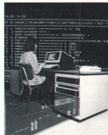
**Cover:** *Contributing to the performance of the new HP 1000 Computer System are an enhanced operating system featuring on-line generation (represented by the CRT display), and a high-performance processor, the 21MX E-Series Computer.*
