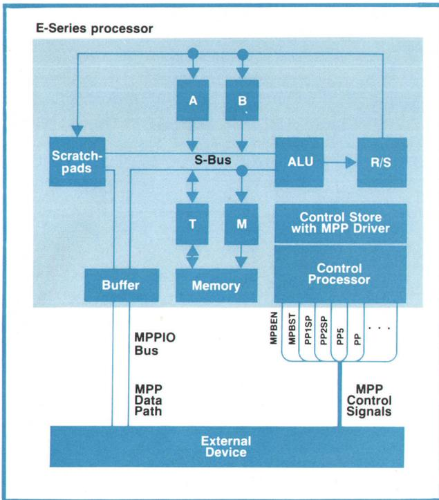
**Fig. 3.** The microprogrammable processor port (MPP) is a new high-bandwidth direct data path between the E-Series processor and an external device, such as a front-end processor, a special arithmetic processor, or another E-Series processor.
