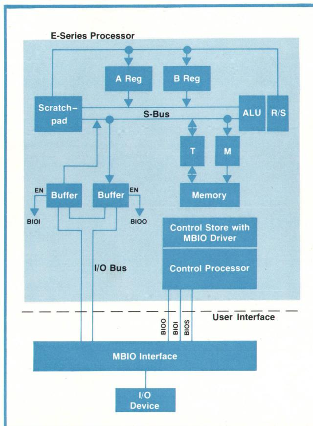
**Fig. 4.** Microprogrammable block I/O is a new feature that provides a microprogrammable data path between the E-Series processor and the I/O bus. Data transfers between I/O bus and processor take only a single microcycle.
