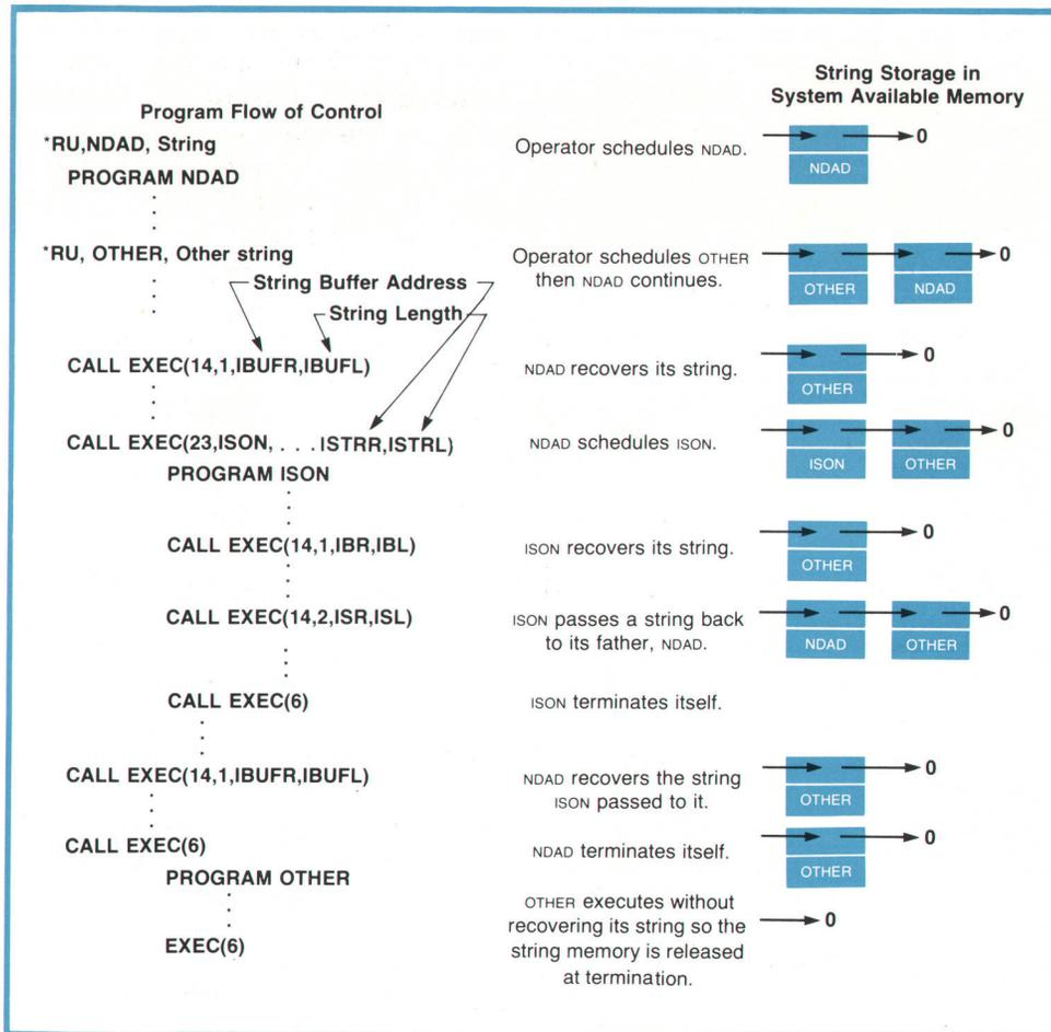
**Fig. 4.** An example of system string communication. Programs NDAD and OTHER are scheduled by the operator while program ISON is scheduled by NDAD. Each time a program is scheduled an optional buffer is saved for it in system available memory. Each time a program recovers a string this memory is released. When OTHER terminates, its unrecovered string is released.
