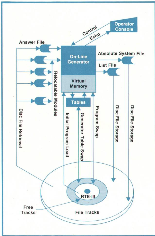
**Fig. 1.** The on-line generator makes it possible to develop a new RTE-II/III operating system configuration under control of the present configuration, concurrently with other system activities. The entire generation process can be directed from a disc answer file. All program modules to be included in the new operating system must exist in relocatable disc files. The new system is stored in an absolute system disc file after generation.
