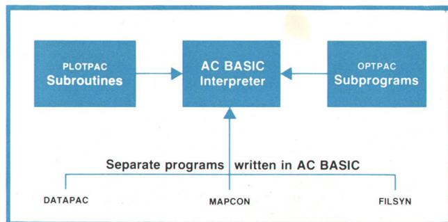
**Fig. 1.** OPNODE is a software package, written in AC BASIC, that runs on HP automatic network and spectrum analyzer systems. It can model, analyze, and optimize linear networks that have up to 40 nodes and 200 components. The OPNODE package includes all of the software modules shown here.
