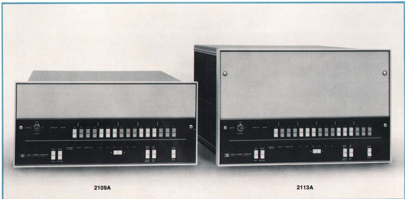
**Fig. 1.** 21MX E-Series Computers have approximately twice the performance of earlier 21MX Computers (the M-Series), at about the same cost. They are used as the processors in HP 1000 Systems and are suitable for OEM applications as well.
