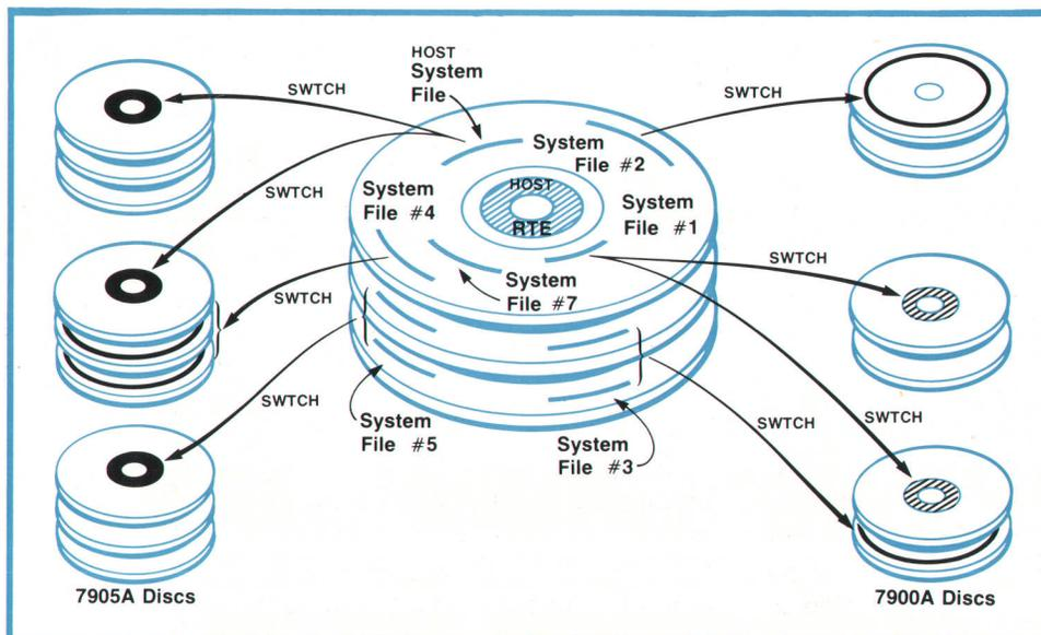
**Fig. 2.** The actual changeover from one RTE-III/III operating system configuration to another is performed by the utility program, SWTCH. Shown here are several types of SWTCH transfers of various RTE-III/III system configurations from their respective disc files to their target disc areas. An important feature of SWTCH is its ability to preserve the file structure of the system being replaced.
