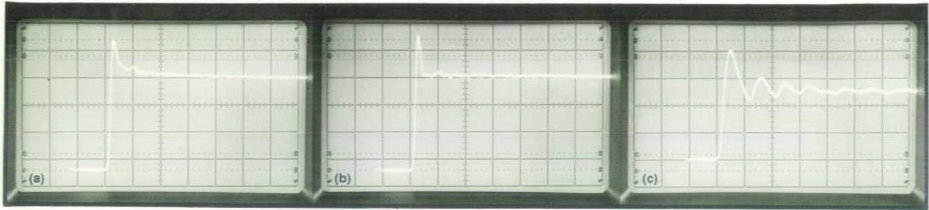
**Fig. 6.** Fast step as viewed on a 275-MHz oscilloscope using a type 10017A miniature 10:1 probe. Signal, oscilloscope, and probe are identical in all three photos; the differences are the result of the grounding attachment hardware: (a) using the 10024A IC clip (Fig. 5) with integral grounding; (b) using the spring-tip ground (Fig. 3); (c) using a conventional IC clip, hook tip, and 20-cm ground lead (Fig. 4). Sweep time is 10 ns/cm.
