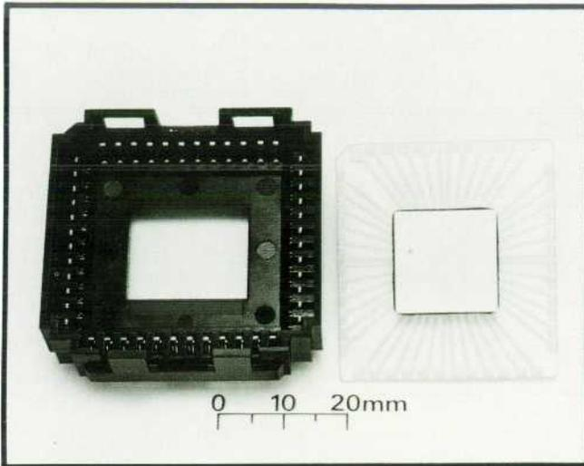
**Fig. 9.** The MC<sup>2</sup> is packaged on a 48-pad ceramic substrate. A special low-insertion-force socket is used.
