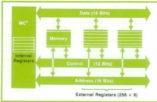
**Fig. 1.** A system based on HP's new CMOS/SOS processor, the MC<sup>2</sup>, is organized around a parallel bus structure. Data, address, and control buses are separate; multiplexing is not used.
