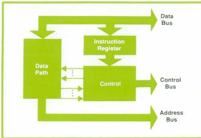
**Fig. 4.** *MC<sup>2</sup> basic block diagram. The data path consists of four blocks of logic that may be connected to a common internal bus or operated independently. See Fig. 5.*
