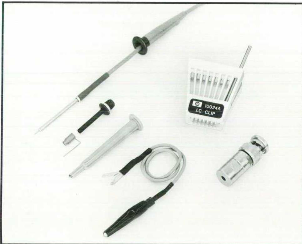
**Fig. 2.** New probe, shown at top with its insulating sleeve removed, is supplied with a spring-type ground lead, a slip-on hook tip, and a flexible ground lead with an alligator clip and it will also be supplied soon with a miniature pincer-type "grabber" (not shown). An IC clip and a probe-tip-to-BNC adapter are also available.
