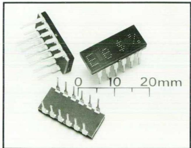
**Fig. 1.** New, small, dot-matrix display has four LED alphanumeric characters in a 12-pin package having standard 0.1-inch lead spacing. With a significant portion of the operating electronics on-board the display unit itself, the display is easier to integrate into a system than earlier dot-matrix displays.
