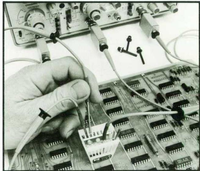
**Fig. 5.** Miniature probe with insulating sleeve removed is held in place on an IC lead by the optional IC clip. The bare ground-reference pin, shown here in the right-hand corner of the clip, can be inserted at any lead position. It grounds reference planes within the clip that in turn contact the barrel of the probe(s). Risetimes as short as 1.3 ns are preserved by this arrangement (Fig. 6).
