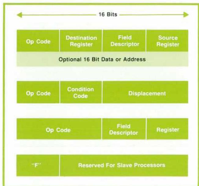
Fig. 3. MC<sup>2</sup> instruction formats. There are 34 classes of instructions. All are 16 bits wide. 16 additional bits for data or addresses are optional.
