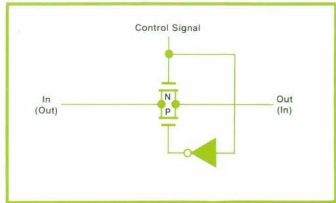
**Fig. 6.** *Logic blocks in the data path are connected to the main bus by full complementary transmission gates. These gates are fast (<1.5 ns delay), small (540 μm<sup>2</sup>), and bidirectional, thereby simplifying complex logic implementation.*
