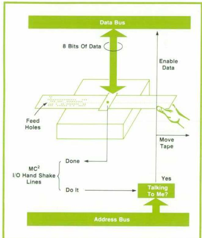
**Fig. 2.** The MC<sup>2</sup> is optimized for controller applications, and treats I/O devices as banks of registers. This simple paper tape reader interface takes advantage of the processor's static and asynchronous properties and direct I/O manipulation.
