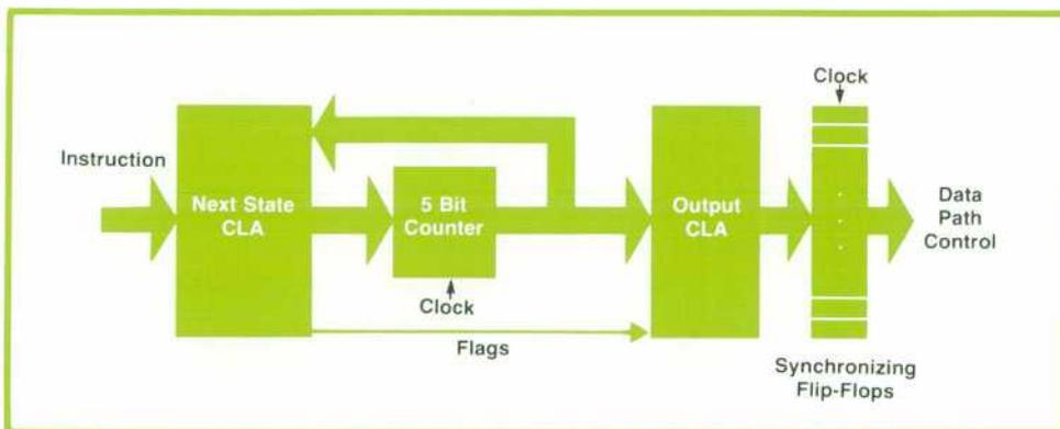
**Fig. 8.** MC<sup>2</sup> control section block diagram. Custom logic arrays (CLAs) are like programmable logic arrays (PLAs, a form of read-only memory) but do not have a full output matrix. The CLAs are controlled by a five-bit counter.
