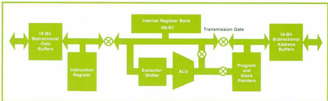
**Fig. 5.** *MC<sup>2</sup> data path block diagram. External registers used for I/O operations are treated in the same way as the internal registers. This allows flexibility in manipulating data while keeping the length of instructions to a minimum.*
