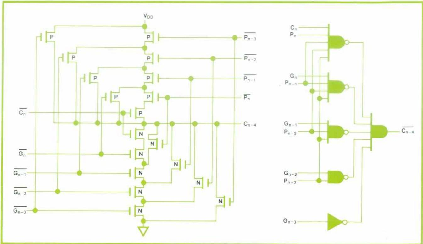
**Fig. 7.** The ALU uses functional gating to save area and generate a 16-bit carry in 35 ns; only half the number of transistors are needed as for a conventional gate realization. Four-bit look-ahead is used in generating the 16-bit carry. There are four carry look-ahead circuits like the one shown here. The ripple method is used within each four-bit block; the combination of methods also helps save area.
