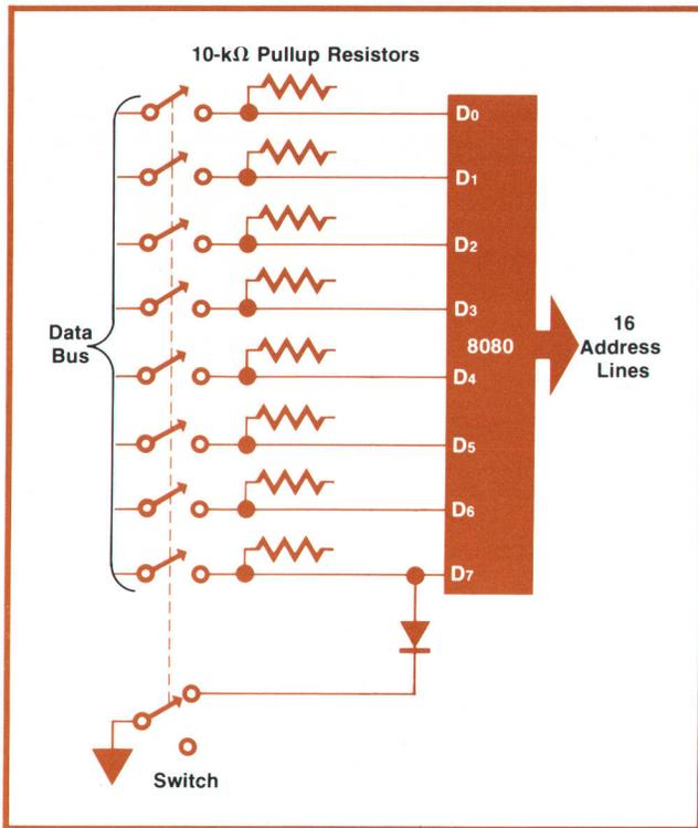
**Fig. 1.** To be an effective troubleshooting technique, signature analysis must be designed into a product. For example, for a test of the address lines of a microprocessor, there should be a switch that opens the data bus and forces the microprocessor to free run. The address lines can then be checked and can also be used as control inputs to the signature analyzer.
