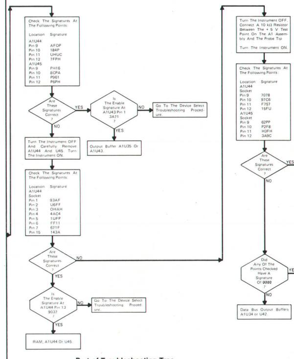
Fig. 8. An example of a troubleshooting chart from the 3455A Voltmeter service manual. The chart tells which part to replace under certain conditions.
