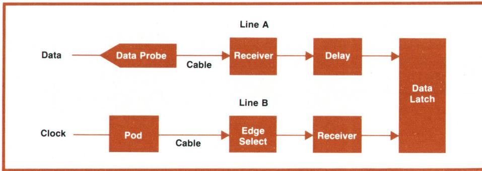
**Fig. 4.** Delays through probe and pod channels are matched so that hold time (the time that input data must remain stable after a clock edge) is non-positive. Setup time (the time that input data must be stable before a clock edge) is typically 7 ns.
