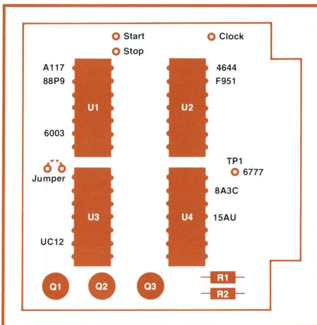
**Fig. 5.** A service manual may use a picture or drawing of the board being tested, showing proper signatures at various test points. A troubleshooting tree in the manual guides the service person, who need not know the function of each component. A board overlay or template may also be used.
