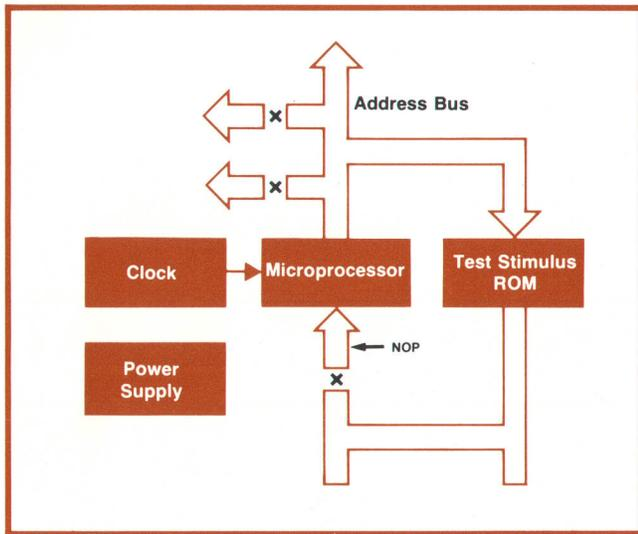
**Fig. 2.** Signature analysis test procedures should verify the operation of key portions—the “kernel”—of a product first, then use the kernel to test other circuits. A typical kernel might consist of microprocessor, clock, power supply, and one or more read-only memories.
