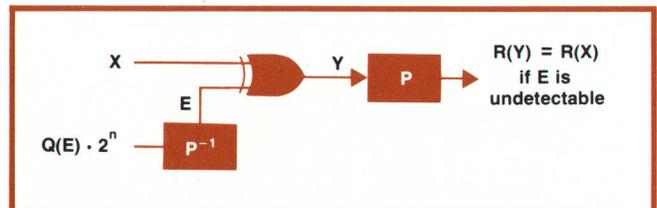
Fig. 4. A diagrammatical representation of errors undetectable by signature analysis. For long data sequences the probability of not detecting an error approaches  $1/2^n$ , where  $n$  is the number of flip-flops in the feedback shift register.
