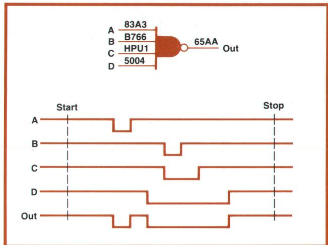
**Fig. 3.** The test stimulus should test each component thoroughly. Otherwise a circuit, such as this AND gate, can have stable and correct signatures at each input and output node and still be bad. For example, input B or C might have an open bonding wire inside the IC, but in this case the error is masked by input D. Careful test stimulus design avoids this.
