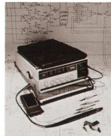
**Cover:** *Those strange-looking strings of four alpha-numeric characters on the instrument's display and the schematic diagram are signatures, and the instrument is the 5004A Signature Analyzer, a troubleshooting tool for field repair of digital systems.*
