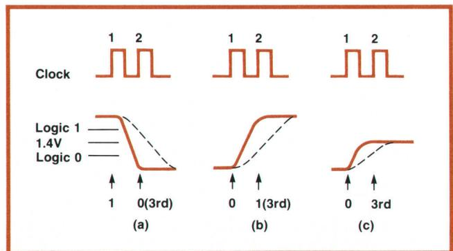
**Fig. 5.** 5004A input impedance is returned to 1.4V to eliminate ambiguities caused by input RC tolerances. Here are three possible results of the input data's changing from a 0 or 1 at clock 1 to a third state at clock 2. The solid and dotted lines are for different values of input RC. In (a), the input at clock 2 can be seen as a logic zero or a third state, depending on the value of RC. (b) is the reverse of (a). In (c), with the input returned to 1.4V, the result is always a third state.
