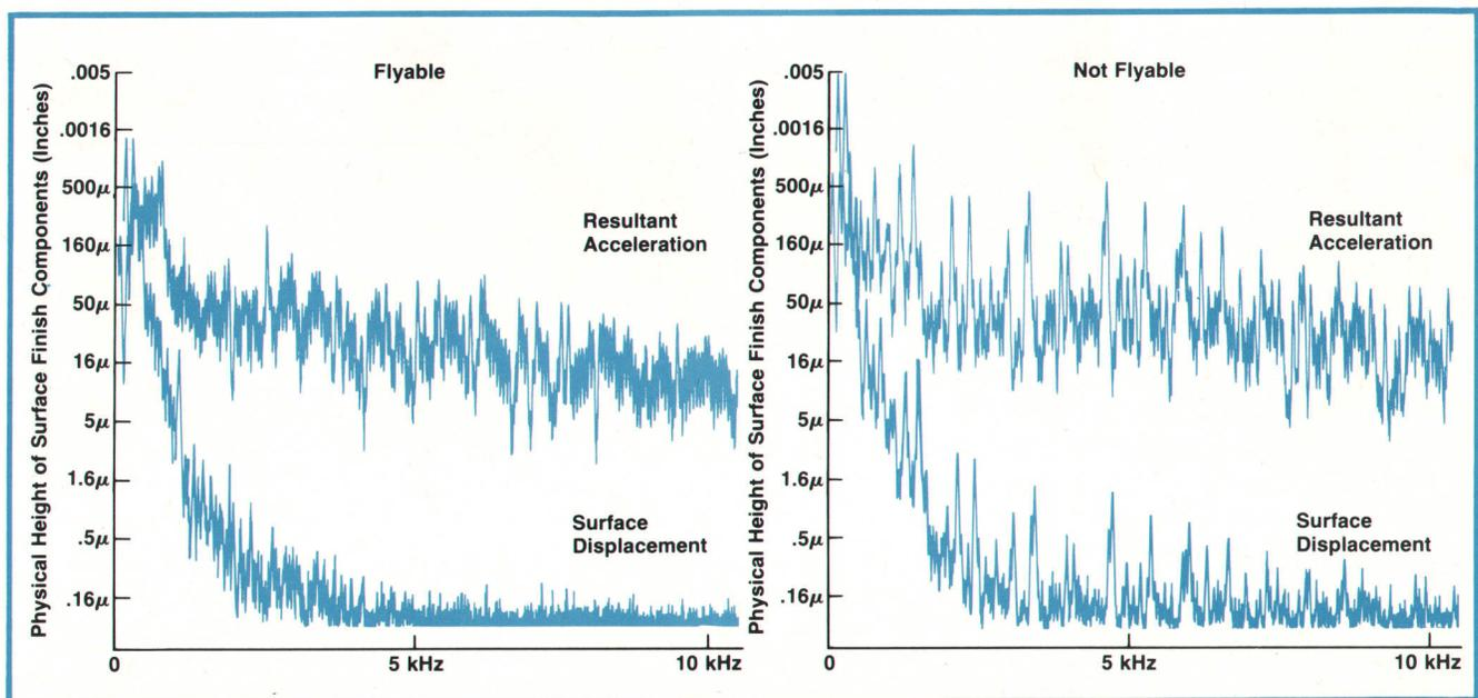
**Fig. 4.** Disc surface undulations can cause head accelerations that lead to head-disc crashes. Shown here are flyable and non-flyable head-disc combinations. Head-media compatibility in the 7920A Disc Drive was investigated using an HP Fourier Analyzer to measure the transfer functions of various system components.
