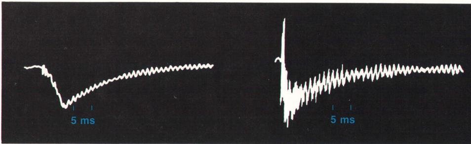
**Fig. 5.** Head seating and settling were investigated using heads with sliders containing crystal accelerometers. Desirable output at left shows rapid seating and settling times. Output at right shows hard impact of the slider on the disc, slow seating, and long periods of ringing.
