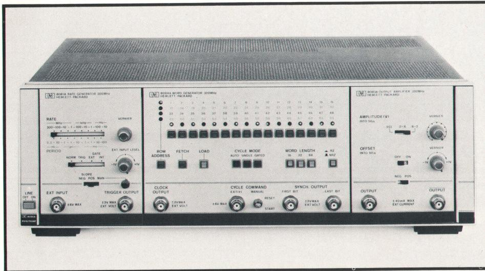
**Fig. 2.** 300-MHz word generator assembled from 8080-series modules produces words 16, 32 or 64 bits long, repetitively or in bursts. The dual-output amplifier supplies the word and its complement with transition times of 800 ps.
