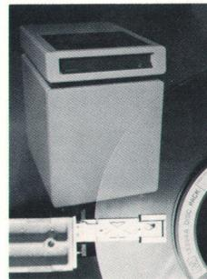
**Cover:** Model 7920A Disc Drive is pictured in a double exposure with its disc pack and one of its read/write heads. The disc pack consists of two protect discs and three data discs and holds 50 megabytes of data. Average seek time is 25 ms.
