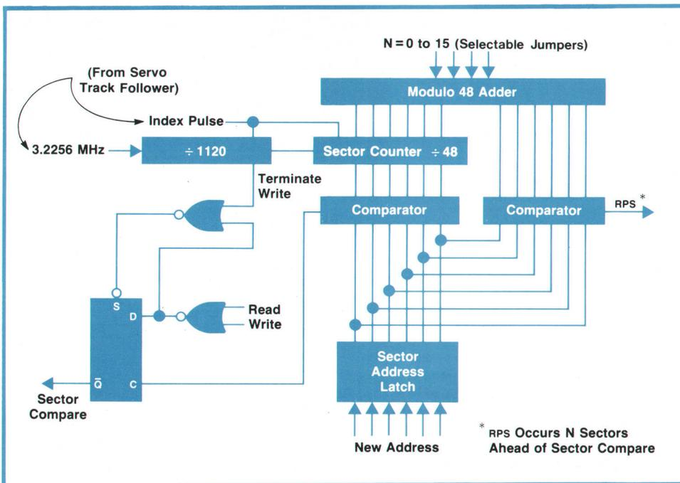
Fig. 11. Sector sensing system monitors circumferential head position.
