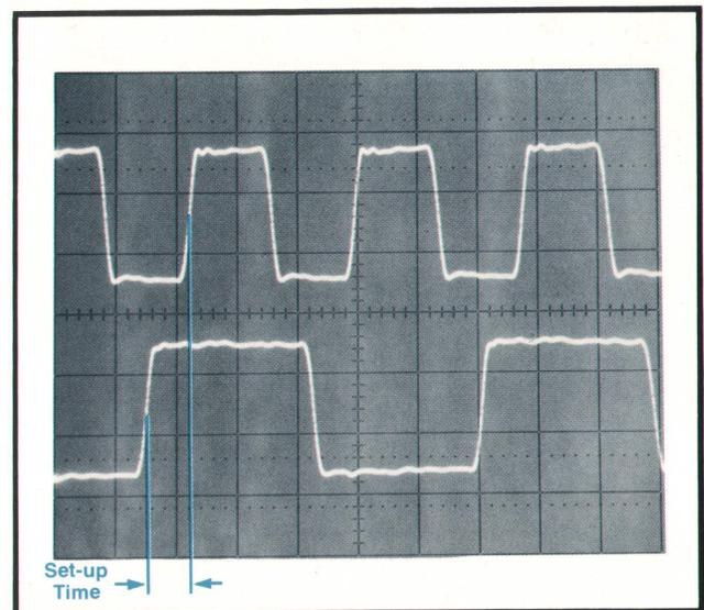
**Fig. 4.** Channel B of the Model 8092A Delay Generator can be switched to function as a frequency divider, producing square waves at one-half the repetition rate of channel A. Use of the interchannel delay then allows examination of setup and hold times of flip-flops.
