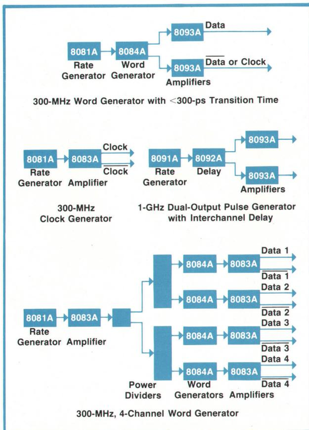
**Fig. 3.** A few of the several pulse/word-generator configurations possible using modules in the 8080 series. Some configurations, such as the multichannel word generator, may require more than one mainframe to house all the modules.
