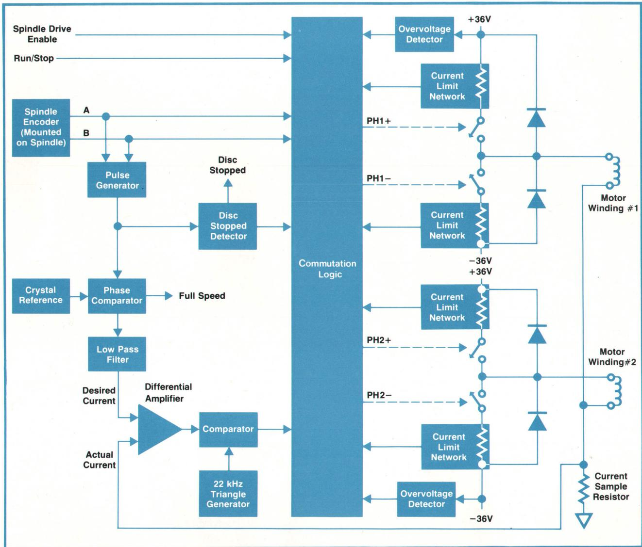
**Fig. 9.** Spindle rotation system is basically a highly efficient switching amplifier. (The switches shown are actually transistor switches.) The system maintains the spindle speed at 3600 r/min. To stop the drive, change the disc pack, and restart the drive takes only 70 seconds.
