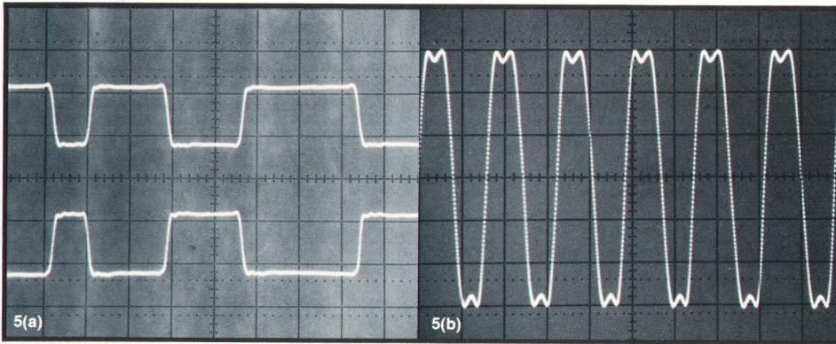
**Fig. 5.** Dual output of the Model 8083A 300-MHz Output Amplifier (a) reproduces the amplifier input at the channel A output while supplying the complement of the input at the channel B output, enabling the generator to drive differential-input devices. Pulse polarity is also selectable. Model 8093A Output Amplifier supplies pulses with less than 300-ps transition times (b). Pulse repetition rate here is 600 MHz. (Oscilloscope sweep time: 1 ns/div.)
