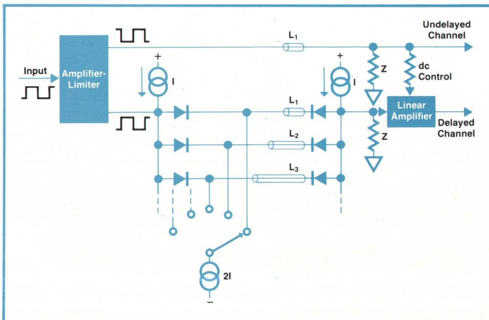
**Fig. 8.** Method of switching transmission lines in the Model 8092A Delay Generator/Frequency Divider to select the pulse delay. With three groups of switched transmission lines in series, the total relative delay is selectable from 0 to 9.9 ns in 100-ps steps.
