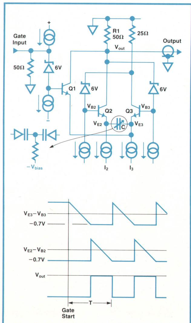
**Fig. 6.** Emitter-coupled oscillator for repetition rates to 1 GHz. Waveforms show time-varying voltages within the oscillator. In the absence of a gating pulse, transistor Q1 clamps the oscillator in a state that corresponds to the running state at the end of time interval T so the first pulse of a burst will be identical to subsequent pulses.
