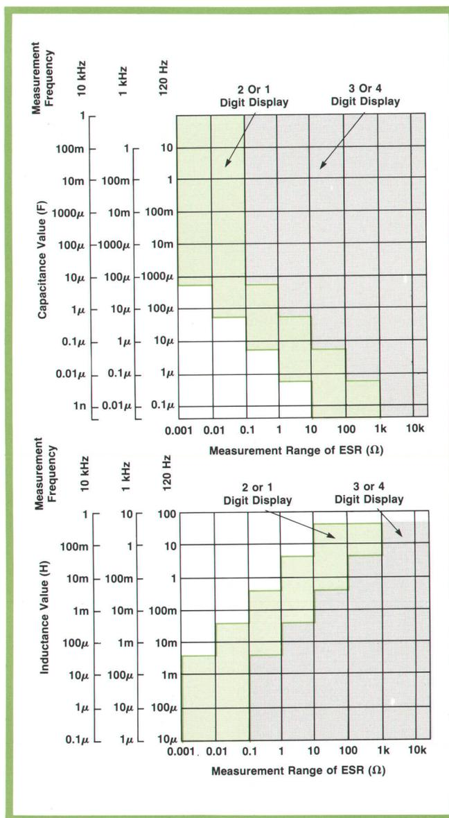
**Fig. 2.** Capacitance and inductance ranges over which the equivalent series resistance (ESR) can be measured with the Model 4262A LCR Meter. The 10-kHz test frequency extends these ranges by a factor of 10 over those usually found in meters of this type.
