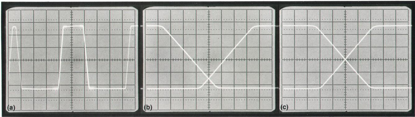
**Fig. 3.** Time-interval measurements are made with Model 1743A by first adjusting the START and STOP controls so the brightened segments of the trace span the start and stop points of the measurement (a), then switching to the  $\Delta$ TIME mode to expand both brightened segments to full screen width (b). The START and STOP controls are then adjusted so the desired start and stop points are on the same vertical graticule line (c), in this case the pulse 50% level.
