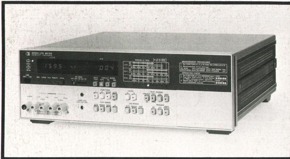
**Fig. 7.** Model 4262A LCR Meter, shown here without options, has a front panel arrangement that facilitates manual control when manual control is preferred to automatic operation. With the HP-IB option installed, all pushbutton functions are programmable through the HP interface bus (all options are field installable).
