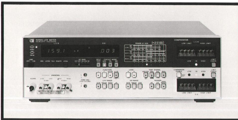
**Fig. 1.** Model 4262A LCR Meter, shown here with the comparator option installed, measures the inductance (L), capacitance (C), resistance (R), dissipation factor (D), and quality factor (Q) of components with 3½ digit resolution. Three test frequencies (120 Hz, 1 kHz, and 10 kHz) enable measurements of a wide range of component values.
