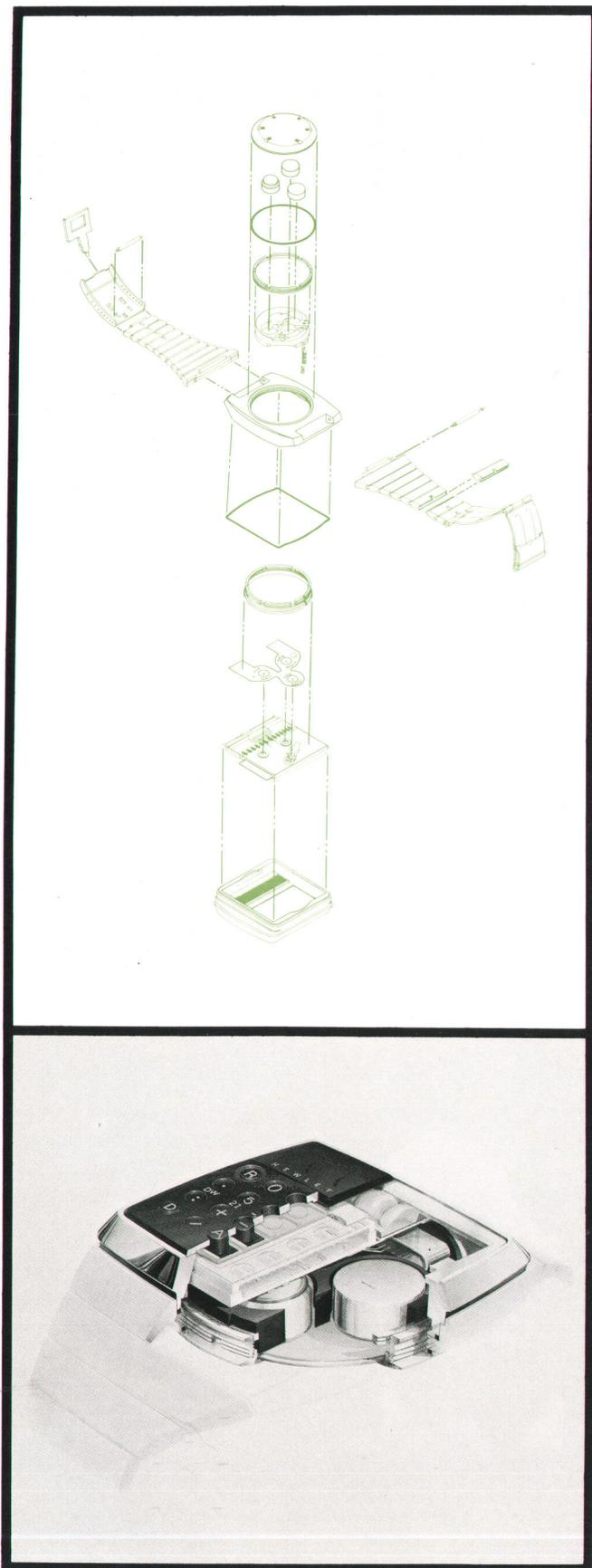
Fig. 4. Exploded and cutaway views of the HP-01.
