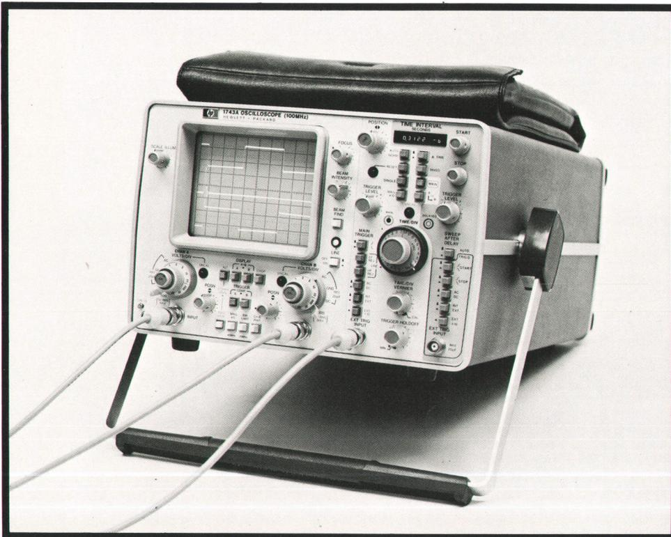
**Fig. 1.** Model 1743A is a general-purpose, dual-channel, 100-MHz oscilloscope that has the capability of measuring very short time intervals with 100-ps resolution. By using a crystal-controlled oscillator as a time reference, and averaging readings, Model 1743A provides the most accurate time-interval measurement capability available in real-time oscilloscopes.
