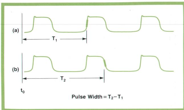
**Fig. 2.** Model 1743A Oscilloscope alternately measures the time from the start of the sweep to a point selected by the START control (a) and to a second point selected by the STOP control (b). Obtaining the difference between the two readings gives the time between START and STOP points.
