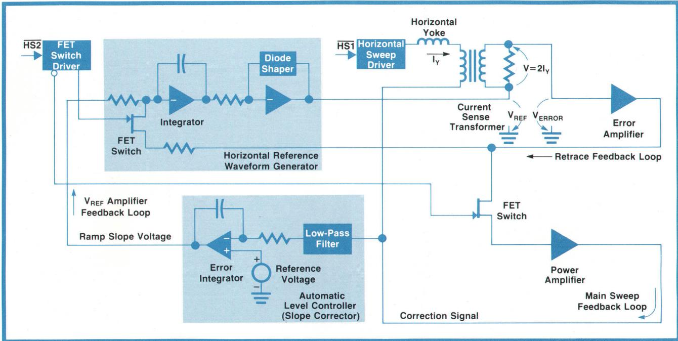
**Fig. 7.** System 45 horizontal sweep circuit uses active linearity correction. The scheme is frequency independent, thus allowing the use of two different horizontal frequencies for the alphanumeric and graphics rasters. The actual yoke current is compared with an ideal waveform to generate a correction signal.
