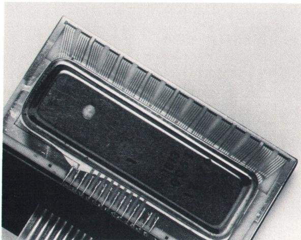
**Fig. 1.** In previous printheads used only for alphanumeric printing there are spaces between groups of print resistors that correspond to the two-dot space between characters. These spaces were used for the return path for the resistor current.
