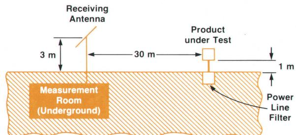
Fig. 3. EMI test range similar to that used by VDE in Offenbach, West Germany. The surface is paved with asphalt and a wire mesh under the asphalt provides a stable reflected wave.
