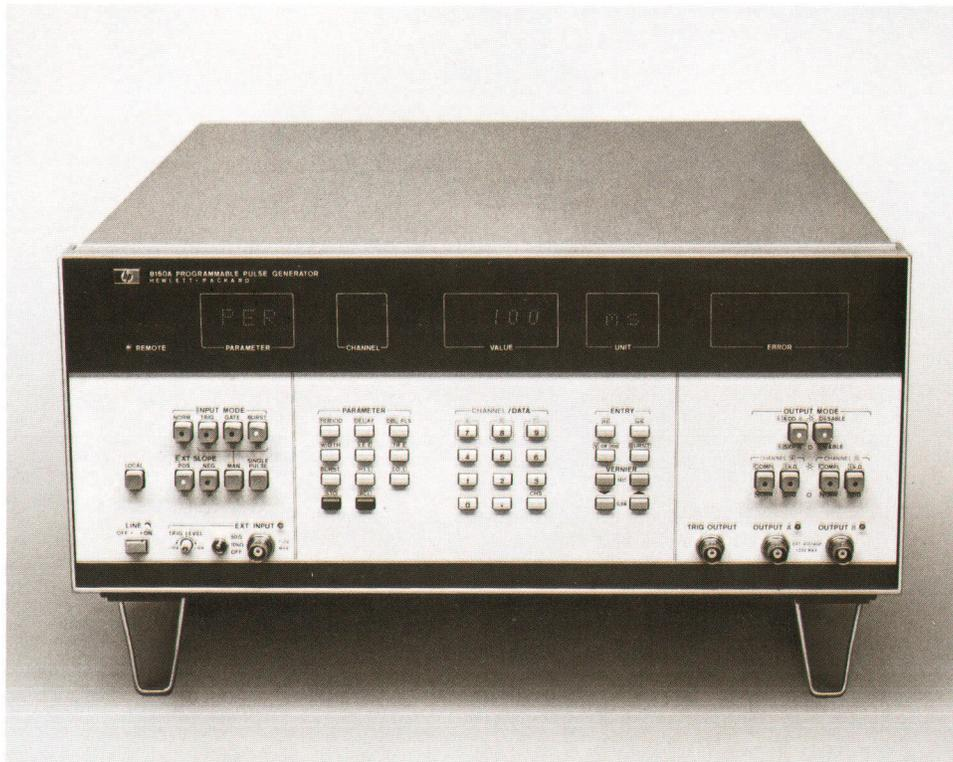
**Fig. 1.** Model 8160A Programmable Pulse Generator produces pulses whose characteristics are within 1-3% of the values entered through the front panel or by way of the HP Interface Bus. Period range is 20.0 ns to 999 ms, amplitude range is 0.10 to 9.99V (into 50 $\Omega$  from a 50 $\Omega$  source impedance), and transition times are variable from 06.0 ns to 9.99 ms. The instrument shown here has the optional second channel that enables two-phase or three-level waveform generation.
