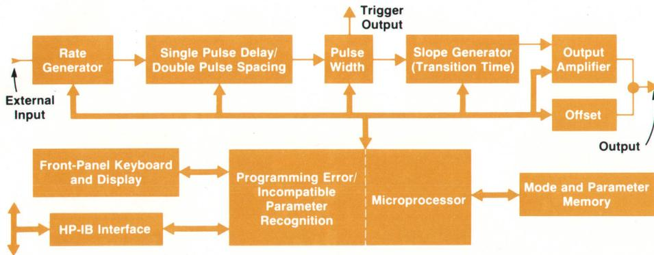
**Fig. 2.** Block diagram of the 8160A Programmable Pulse Generator. All pulse parameters and operating modes are controlled by the microprocessor whether the instrument is operated manually or remotely through the HP Interface Bus.
