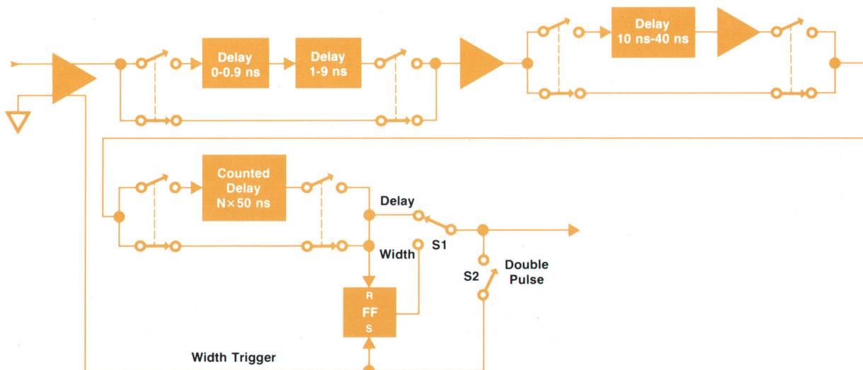
**Fig. 11.** Basic time-interval circuit functions as either a delay or a width generator depending on the setting of switch S1. For double pulse operation, switch S2 passes both the trigger pulse and the delayed trigger to the width circuit following.
