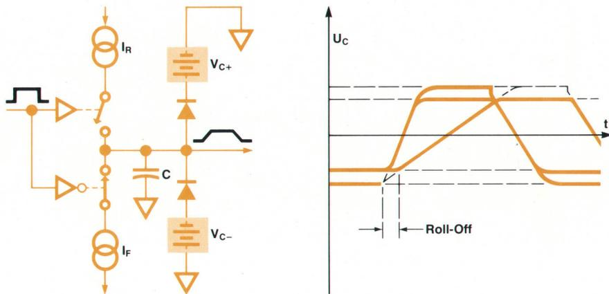
**Fig. 12.** Conventional slope generator is followed by a limiter stage to remove the step at the start of each transition. Changing the leading edge slope thus affects the start time of the pulse. This is the roll-off effect.
