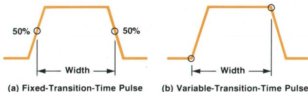
**Fig. 3.** Definitions of pulse width. The traditional way defined the width of pulses with fixed transition times as the time between the 50% points of the leading and trailing edges (a). Current practice for pulses with variable transition times (b) defines pulse width as the time from the start of the leading edge to the start of the trailing edge (10% and 90% points). This measure is unaffected by a change in transition time of either edge.
