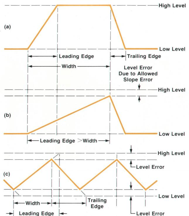
**Fig. 4.** If the leading-edge transition time exceeds pulse width, the amplitude (high level) will be less than that programmed (b). If the pulse width plus the trailing edge transition time exceeds the pulse period, the pulse baseline (the low level) will be higher than that programmed. Both errors are allowed by the 8160A and can occur simultaneously (c).
