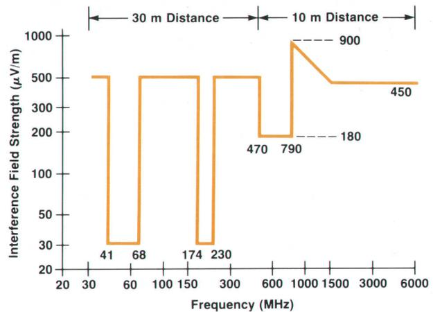
Fig. 2. VDE interference field strength limits and distance of measurement.
