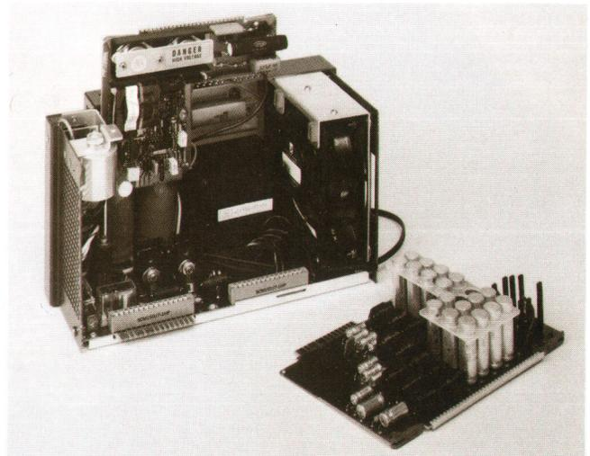
**Fig. 16.** Power supply with one circuit board removed and another raised in position to disclose details. Although the supply is compact, cooling air is able to flow freely over heat-dissipating surfaces.
