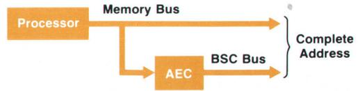
**Fig. 3.** At the start of each memory access the address extension chip places the contents of one of its six registers on the BSC bus. This block select code and the address from the processor form the complete address.
