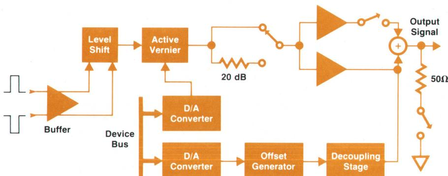
**Fig. 15.** Organization of the output stage. With the 50 $\Omega$  termination switched in, the output stage absorbs reflections from external impedance mismatches. With it switched out, the effective source impedance is 1 k $\Omega$ .
