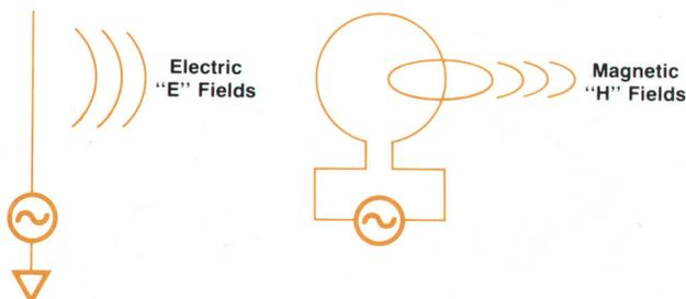
Fig. 1. Radiation model of electric and magnetic fields.
