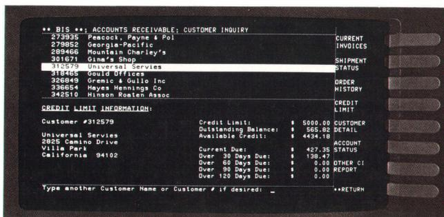
**Fig. 6.** In this customer record application, the user can scroll the customer of interest into the inverse-video row and press the appropriate softkey to see detailed information on that customer displayed in the lower window.
