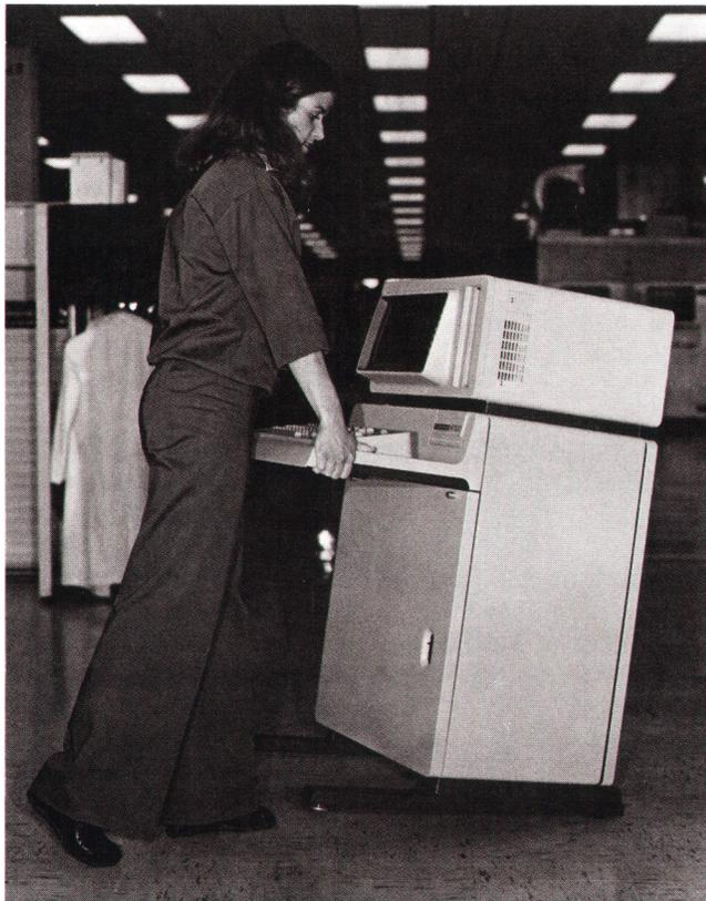
**Fig. 4.** HP 300 can be moved like a wheelbarrow.
