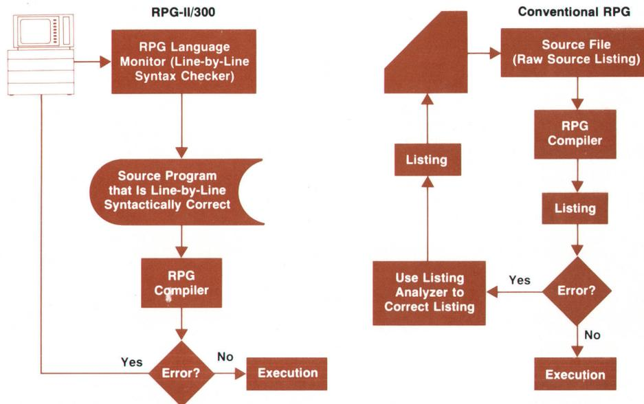
Fig. 6. RPG-II/300 and conventional RPG program development cycle.
