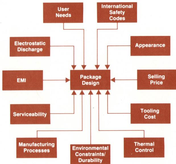
Fig. 1. Design parameters for the HP 300 package design.
