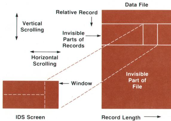
**Fig. 5.** Files can be attached to windows so that data can be displayed exactly as it appears in a file. Each window may be scrolled independently through its attached file, up or down, left or right.
