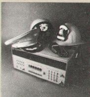
If our cover photograph tells you that this month's featured instrument tests the kinds of transmitters that are used by fire, police, and airline personnel, we've been successful. Model 8901A Modulation Analyzer is a new kind of analyzer that makes it possible to do a better job of testing AM and FM transmitters, signal generators, crystal oscillators, and many other devices that operate in the radio frequency range, specifically 150 kilohertz to 1300 megahertz.
