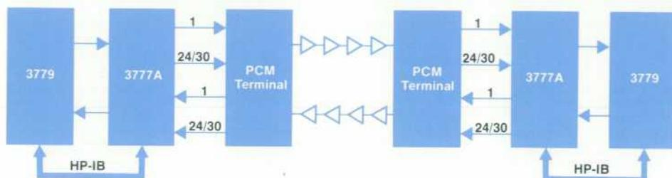
Fig. 1. End-to-end measurement setup.
