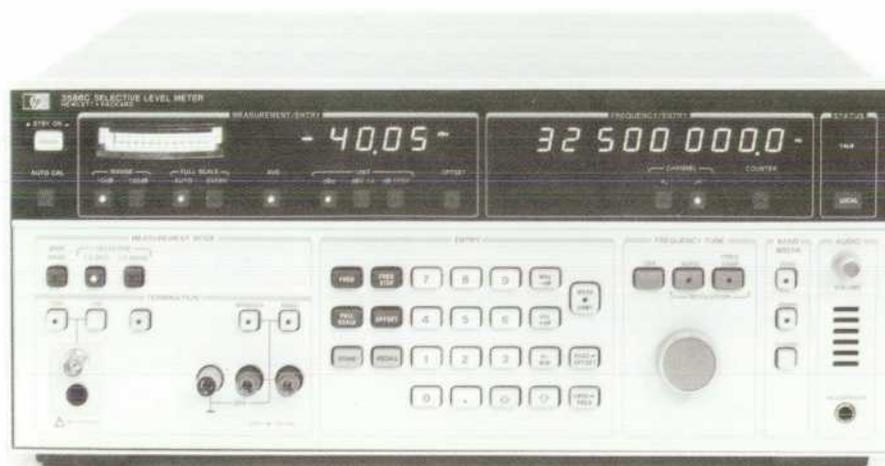
**Fig. 1.** Model 3586A/B/C Selective Level Meter (3586C shown) is designed for general-purpose wave analysis and telecommunications applications including audio, sonar, radio, and frequency division multiplex (FDM) systems testing. It has a frequency range of 50 Hz to 32.5 MHz,  $\pm 0.2$ -dB level accuracy, and 0.1-Hz frequency resolution.
