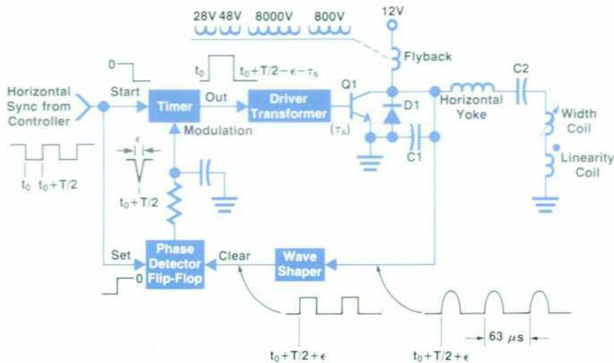
**Fig. 4.** Horizontal amplifier circuit. The phase control loop is used to maintain the beam position with respect to dot timing. The flyback autotransformer provides the high potentials required for CRT operation.
