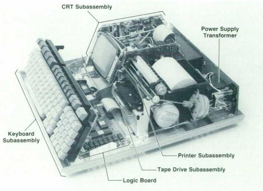
**Fig. 2.** Internal view of the HP-85 with the major subassemblies identified. The compact designs of these subassemblies make it possible to provide a complete computer system in a single portable package.
