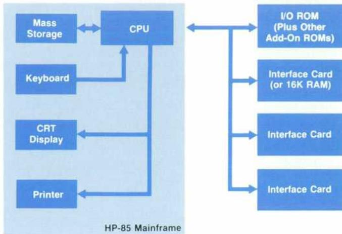
**Fig. 1.** The basic functional blocks for the HP-85 personal computer are integrated into a single mainframe for a self-contained computer system. Four I/O slots are provided to expand system capability. Various combinations (such as the one shown) of the add-on ROM drawer, additional 16K RAM, and peripheral interfaces can be installed in these four slots.
