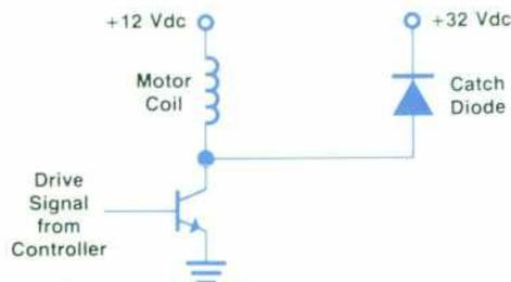
**Fig. 3.** Printer motor driver circuit. The energy stored in the motor's inductance is returned to the system power supply through the catch diode. This approach speeds up the stepping rate and conserves power.
