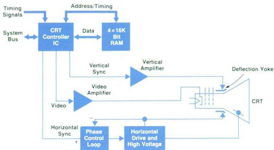
**Fig. 2.** Block diagram of the CRT subassembly for the HP-85. The heart of this unit is the CRT controller IC, which generates timing signals, draws characters, and interfaces to the main system.
