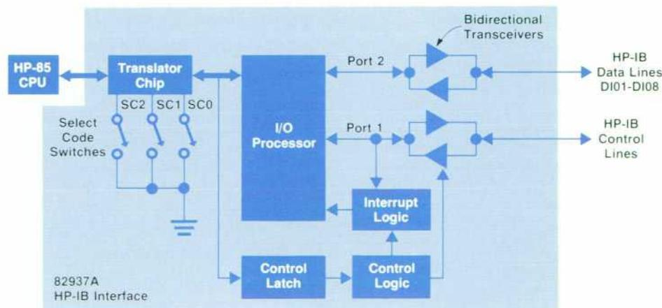
**Fig. 2.** Typical interface card design. The translator chip permits communication between the system CPU and the microprocessor on board the interface. The I/O processor then implements the electrical requirements for the particular interface functions.
