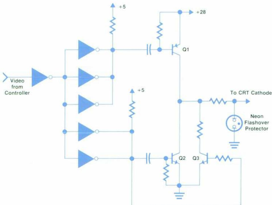
**Fig. 5.** Video amplifier circuit. The TTL drivers on the left prevent Q1 and Q2 from going into saturation. Class C operation is used to conserve power. Q3 is used to maintain beam intensity when displaying long lines.
