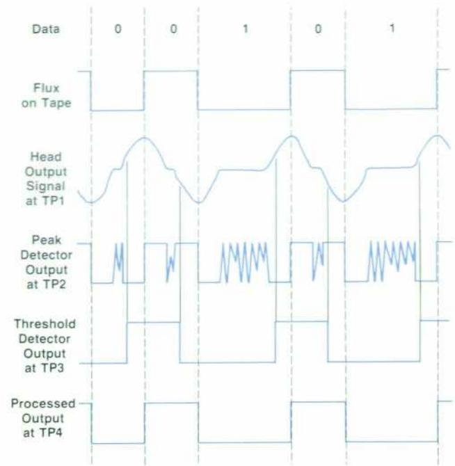
Fig. 7. Time relationship between the various signals involved in reading data from the tape. See Fig. 6 for the location of these signals in the read/write amplifier and detector circuit.
