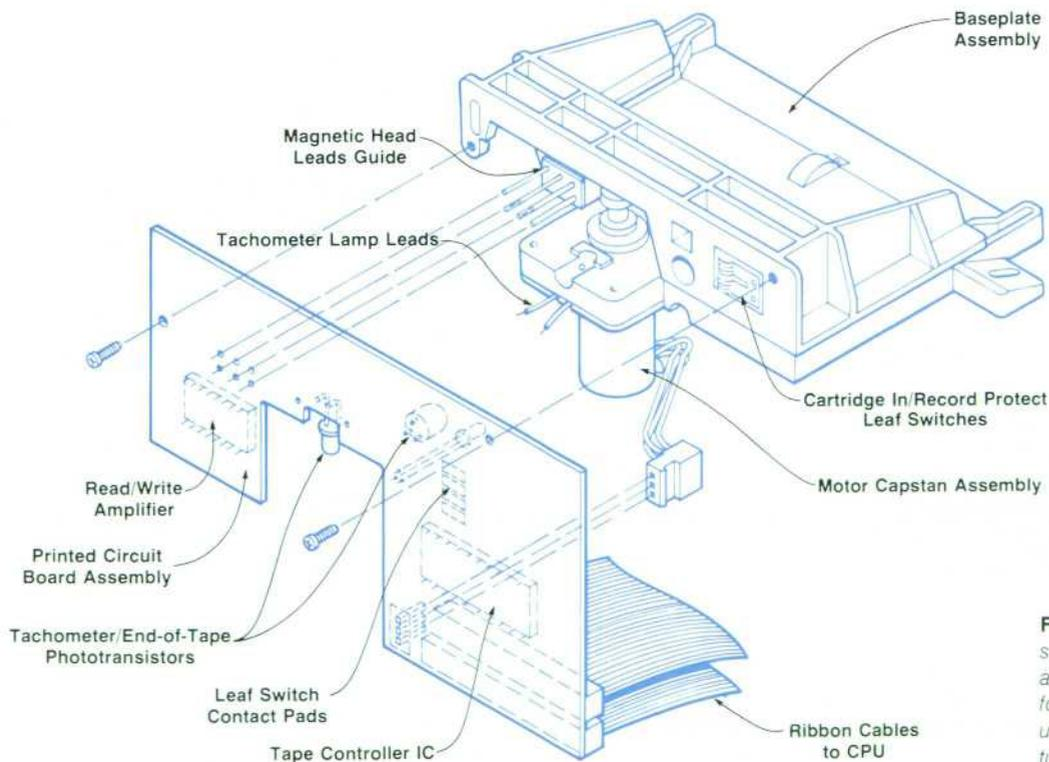
**Fig. 8.** Tape cartridge transport subassembly. The mechanical and electrical designs combine to form a compact, highly reliable unit that can be easily manufactured.
