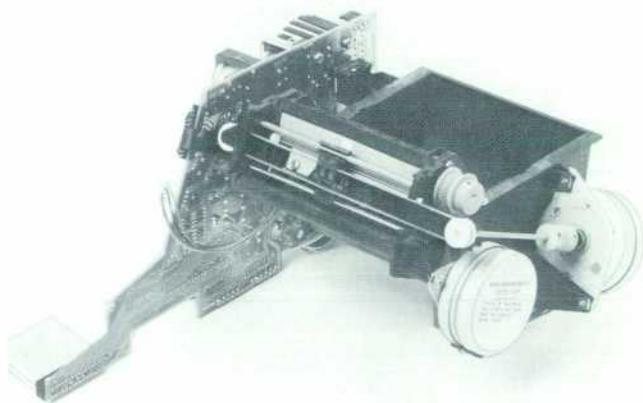
**Fig. 1.** HP-85 thermal printer subassembly. In addition to the printing mechanism, this subassembly also contains both the support electronics for printing and the circuitry for the HP-85 power supply.
