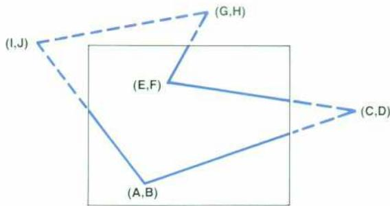
**Fig. 2** Example of clipping performed by the HP-85 system when the plot exceeds the boundary of the screen display. First, a line is drawn from (A,B) toward point (C,D) off-screen. A line drawn now from (C,D) to (E,F) will intersect the edge of the CRT display at the proper point. Thus, the CRT acts as a window on a much larger plotting space. The size of the window is specified by the SCALE statement.
