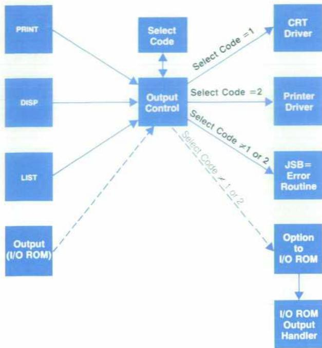
**Fig. 4.** An output control routine directs the output from PRINT, DISP, and LIST statements to the selected peripheral. If the peripheral is not present, the routine calls an appropriate error routine. When additional peripherals are added to the HP-85 system the I/O ROM supplies an additional OUTPUT command and redirects the normal error subroutine call from the output control routine to the appropriate subroutine in the I/O ROM.
