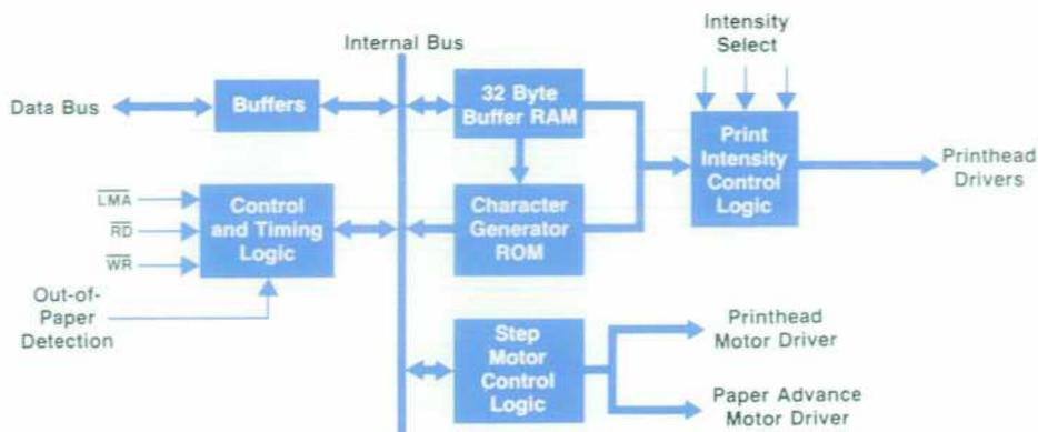
**Fig. 2.** Block diagram for the printer controller integrated circuit. This chip controls the printer mechanism motors and print intensity, buffers the data to be printed, and handles control and timing functions.
