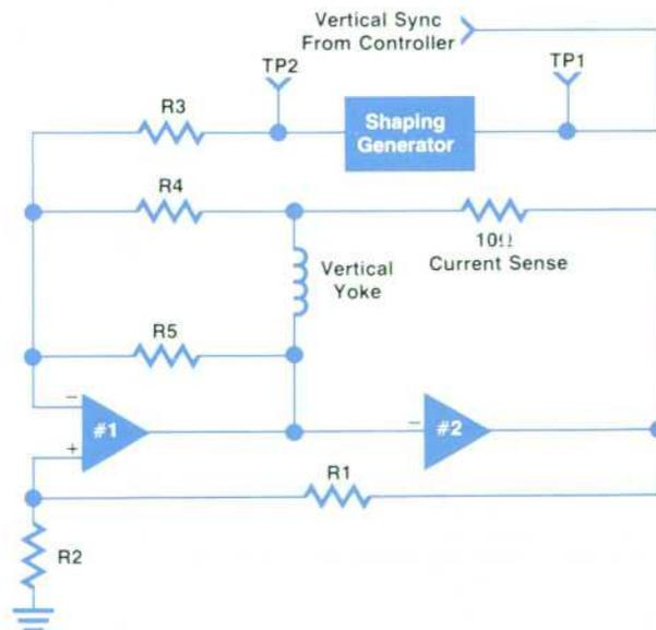
**Fig. 3.** Vertical amplifier circuit. The two amplifiers are class AB designs operating in phase opposition, and the resistors are used for feedback from the current sense resistor. The shaping generator compensates for higher writing velocities at the edges of the display.
