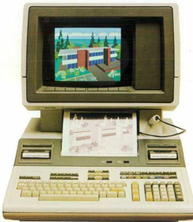
**Fig. 2.** The System 45C is an integrated computer graphics system with a high-resolution color display, thermal printer, two tape cartridge drives, light pen, high-performance I/O, and mass storage capability.
