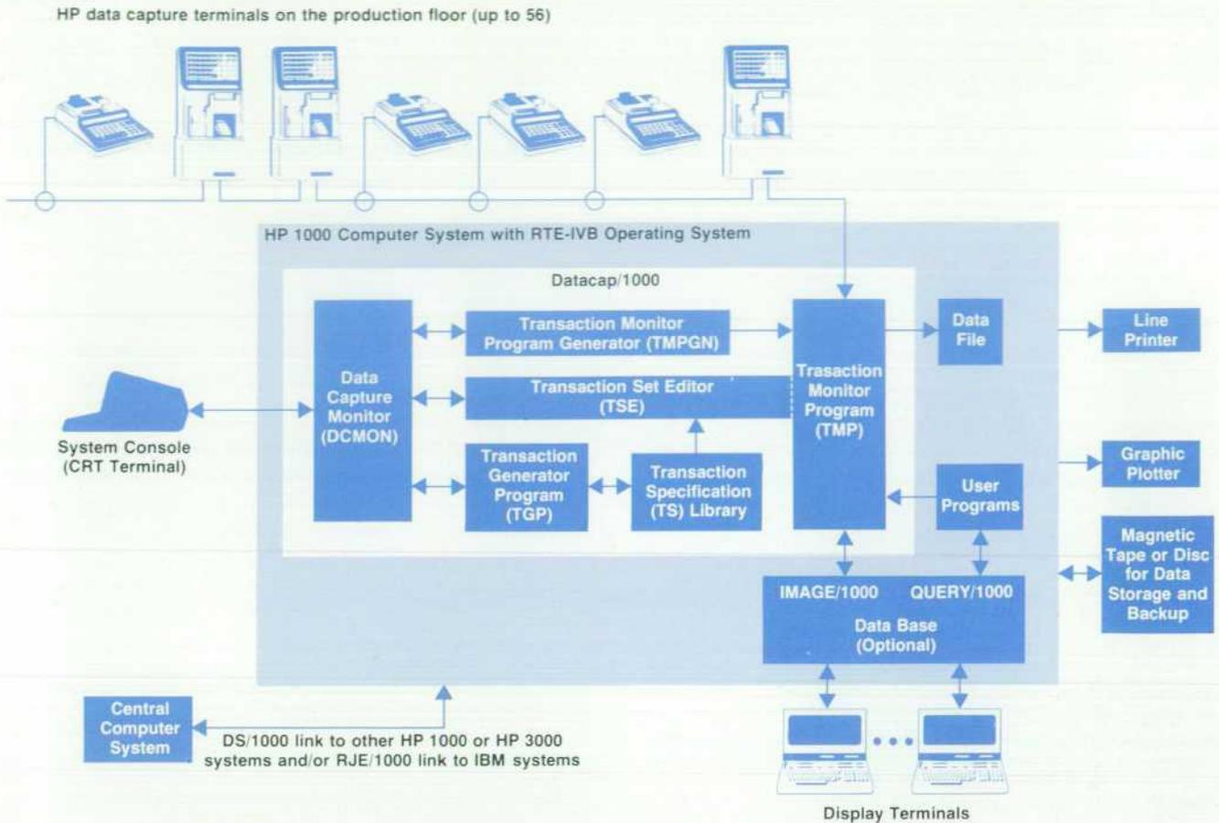
**Fig. 3.** Major components of DATACAP/1000. The transaction generator program (TGP) and transaction monitor program generator (TMPGN) interactively lead the user through the process of building transaction specifications and the transaction monitor program (TMP). The TMP then manages the collection of factory data and creates data files or enters the data into the IMAGE/1000 data base, if present.
