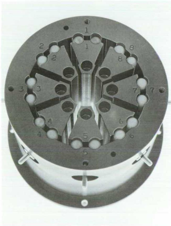
Fig. 4. Octopole assembly. This unit deflects the beam with high accuracy and is used to direct the beam to each of the  $64\text{-}\mu\text{m}$ -square raster-scanned blocks in the system's 5-mm-square field-of-view.
