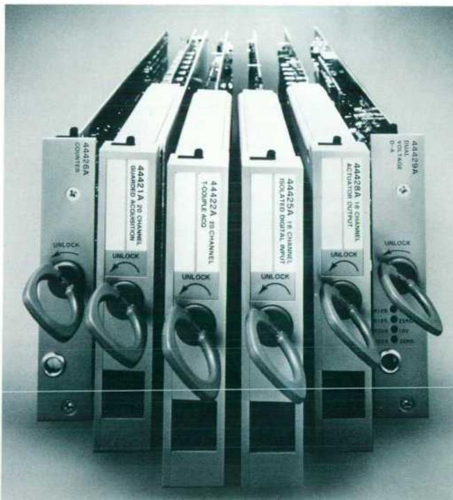
**Fig. 1.** The 3497A Data Acquisition/Control Unit has a variety of plug-in assemblies that measure physical parameters, actuate devices, input and output digital data, convert digital commands to voltages and currents, and scan many channels.
