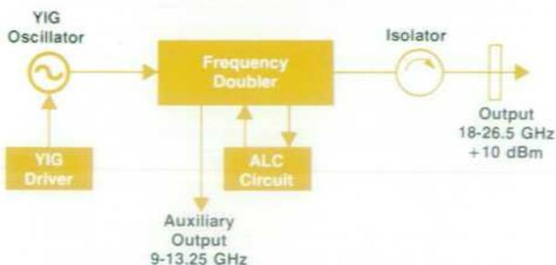
Fig. 4. Block diagram of the 83570A 18-to-26.5-GHz plug-in.
