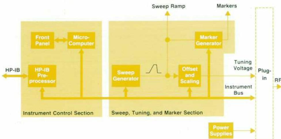
**Fig. 7.** Block diagram of the 8350A Sweep Oscillator.
