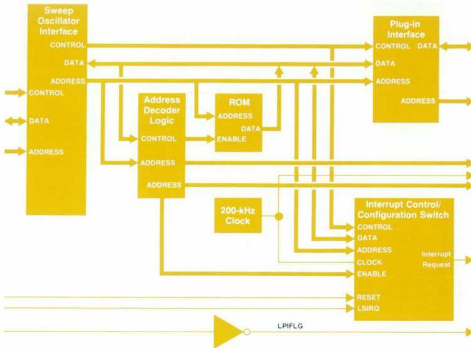
Fig. 6. Digital control section of the 83500 Series plug-ins.
