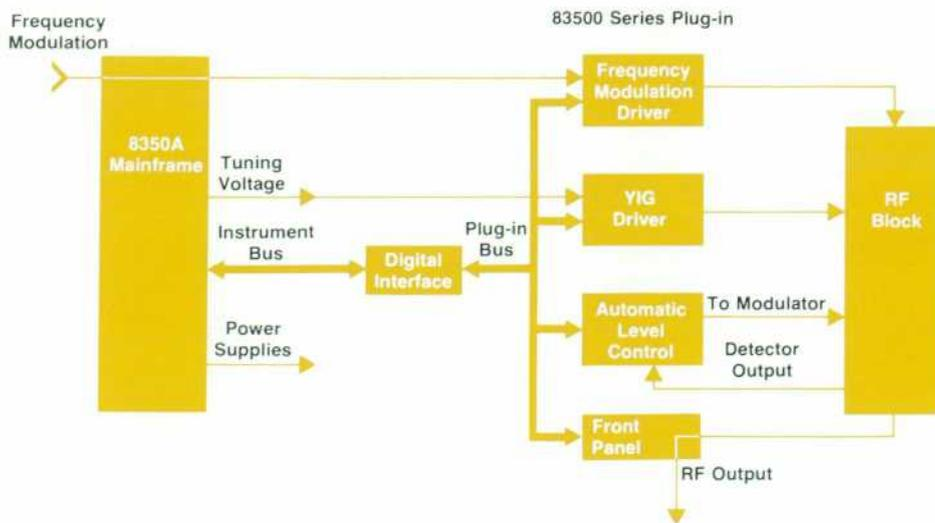
Fig. 2. General block diagram of an 83500 Series plug-in.
