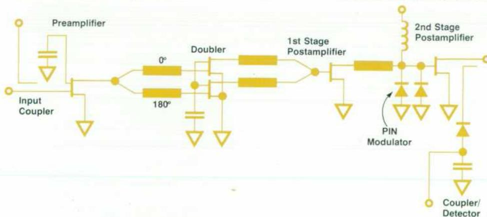
**Fig. 2.** Schematic diagram of the frequency doubler.
